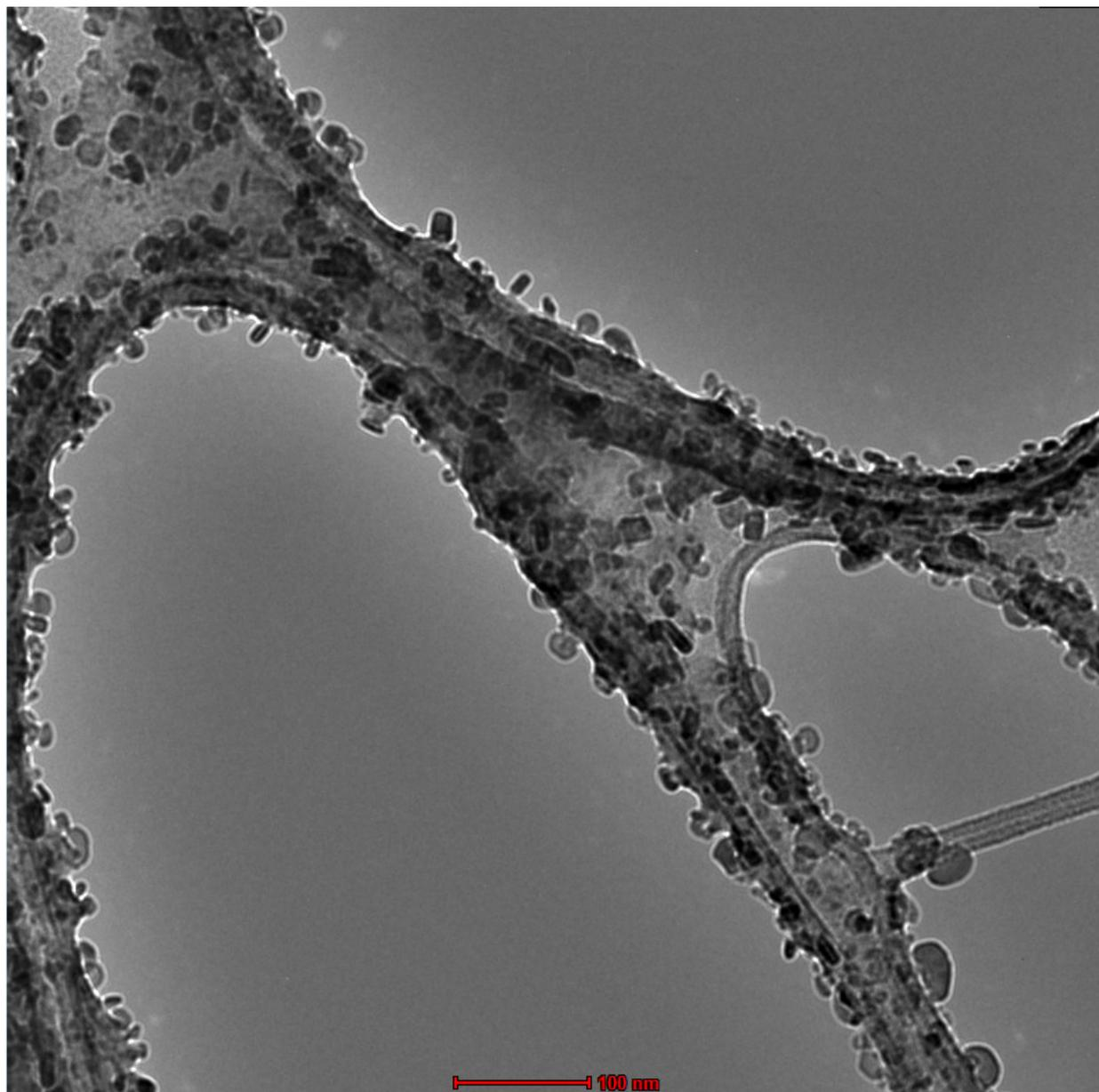
**Figure S4:** TEM image of FeS<sub>2</sub> Nano-Spheres after photocatalytic experiment. It can be seen that the particles to extent degrade during the process, which is also shown by the shift in the absorbance peak, but remain mostly intact.
