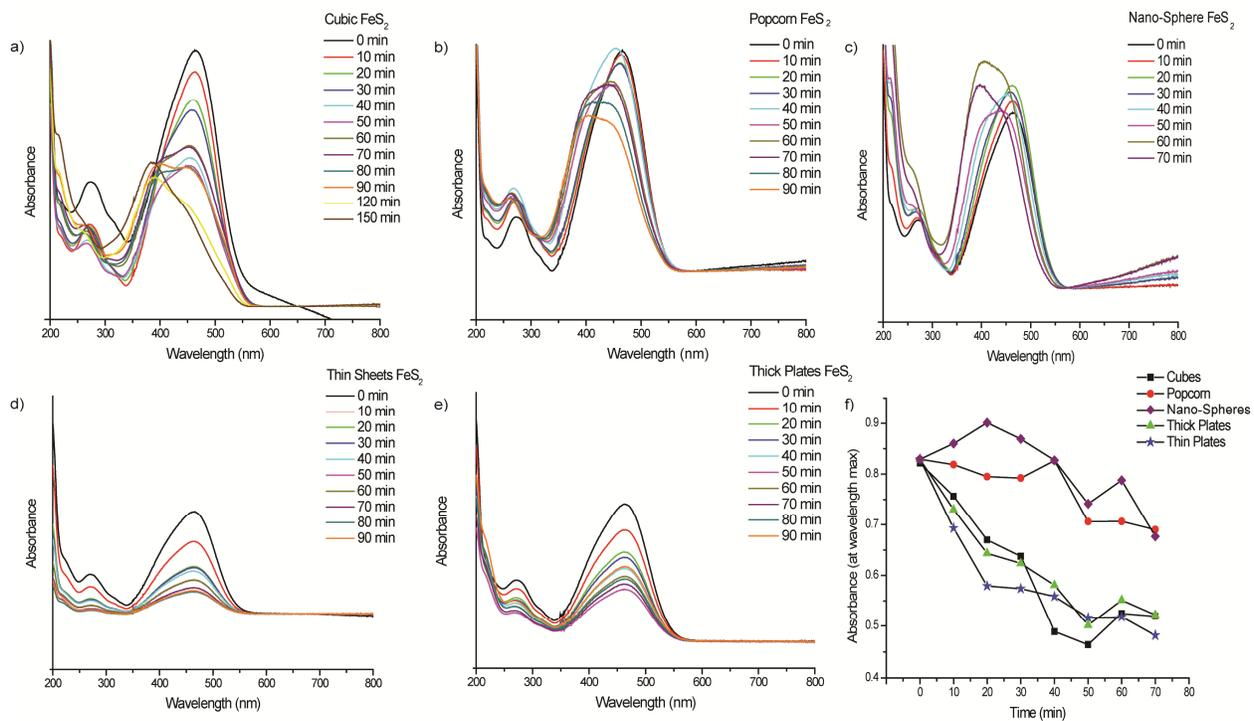
**Figure S3:** Methyl orange degradation spectra results for (a) cubes, (b) popcorn, (c) nano spheres, (d) thin sheets, (e) thick sheets. Absorbance at  $\lambda_{\max}$  vs. time (min) for all samples presented in (f).
