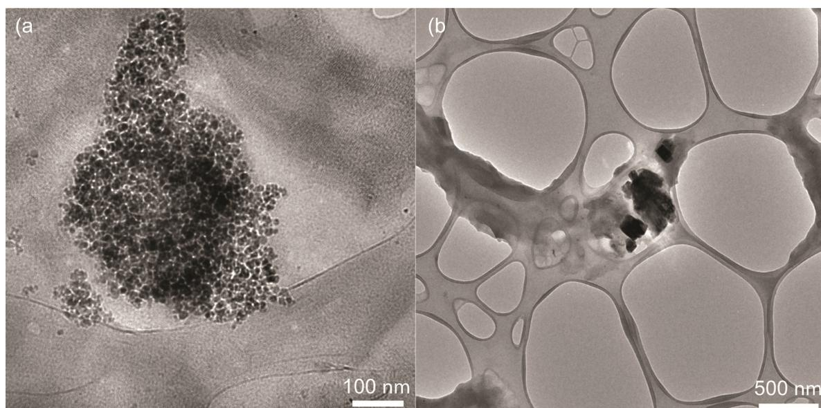
**Figure S2:** TEM images of seed's at 5 min into reaction of FeCl<sub>2</sub> precursor at (a) 220°C synthesis showing that the seeds start as Quantum dots and (b) 120°C synthesis the seeds start as cubes.
