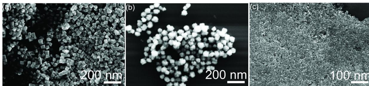
**Figure S1:** SEM images of FeS<sub>2</sub> nanocubes (120°C synthesis), popcorns (170°C synthesis) and nano spheres (120°C synthesis) of FeCl<sub>2</sub> precursor.
