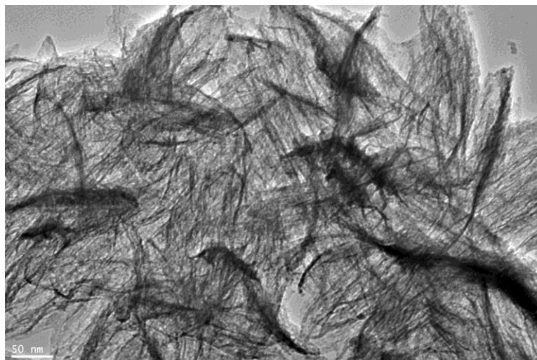
Fig.S3 TEM images of the sample synthesized via hydrothermal treatment at 200 °C for 10 h with the addition of 40 g NaNO 3 .
