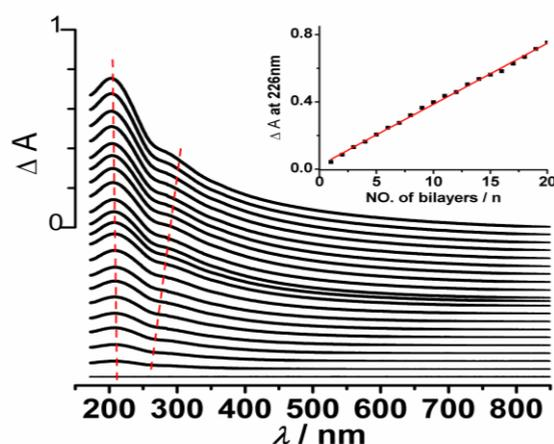
Figure S1. UV/vis absorbance spectra of [PDDA@GO]<sub>n</sub> with different numbers of bilayers from 0 to 20. Inset shows the linear relation between the absorbance at the peak and the number of bilayers.
