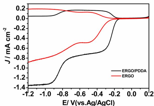
Figure S4. RRDE of ERGO/GC and (ERGO/PDDA)/GC electrodes in air-saturated 0.1 M KOH with the rotation rate of 2500 rpm.
