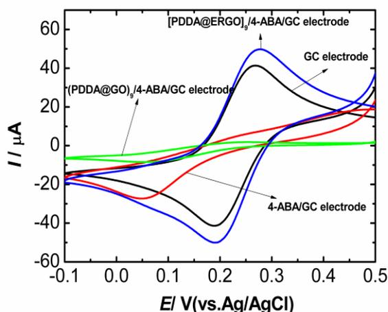
Figure S2. CV curves recorded at GC, 4-ABA/GC, [PDDA@GO]<sub>9</sub>/4-ABA/GC, and [PDDA@ERGO]<sub>9</sub>/4-ABA/GC electrodes for 5 mM [Fe(CN)<sub>6</sub>]<sup>3-/4-</sup> in 0.1 M KCl solution at the scan rate of 5 mV s<sup>-1</sup>.
