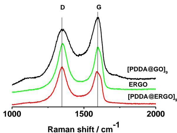
Figure S5. The Raman spectra of [PDDA@ERGO]<sub>9</sub>, pure ERGO and [PDDA@GO]<sub>9</sub>.
