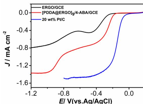
Figure S3. RDE linear sweep voltammograms for oxygen reduction on the ERGO/GC and [PDDA@ERGO]<sub>9</sub>/4-ABA/GC electrodes and 20 wt% Pt/C in air-saturated 0.1 M KOH at a rotation rate of 2500 rpm. Scan rate: 10 mV s<sup>-1</sup>.
