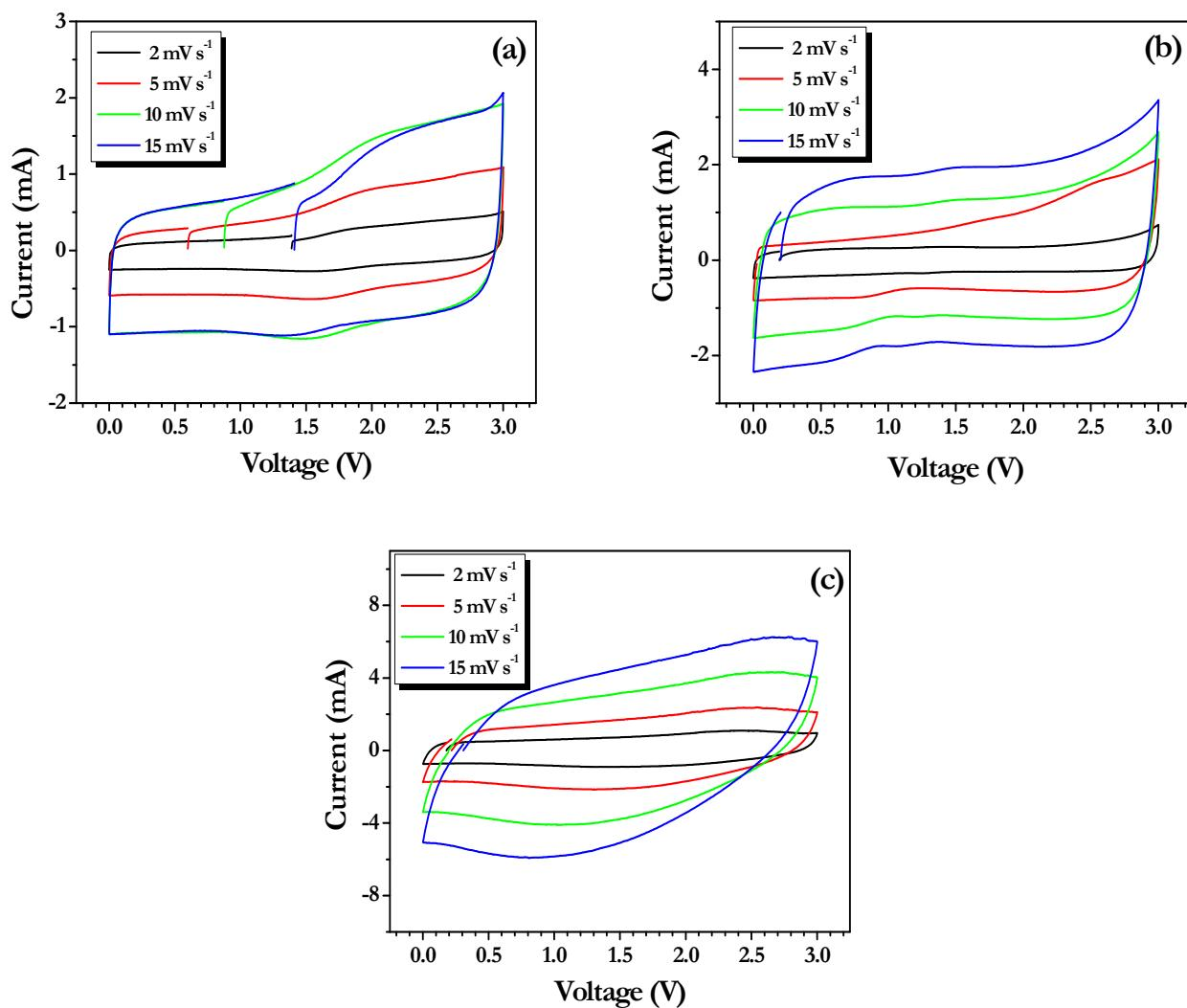
**Figure S2.** CV curves of (a) Li(Mn<sub>1/3</sub>Ni<sub>1/3</sub>Fe<sub>1/3</sub>)O<sub>2</sub>/AC (b) Li(Mn<sub>1/3</sub>Ni<sub>1/3</sub>Fe<sub>1/3</sub>)O<sub>2</sub>-PPy/AC and (c) Li(Mn<sub>1/3</sub>Ni<sub>1/3</sub>Fe<sub>1/3</sub>)O<sub>2</sub>-PANI/AC cells recorded at different current rates between 0-3 V in the presence of 1 M LiPF<sub>6</sub> in EC:DMC (1:1 v/v.).
