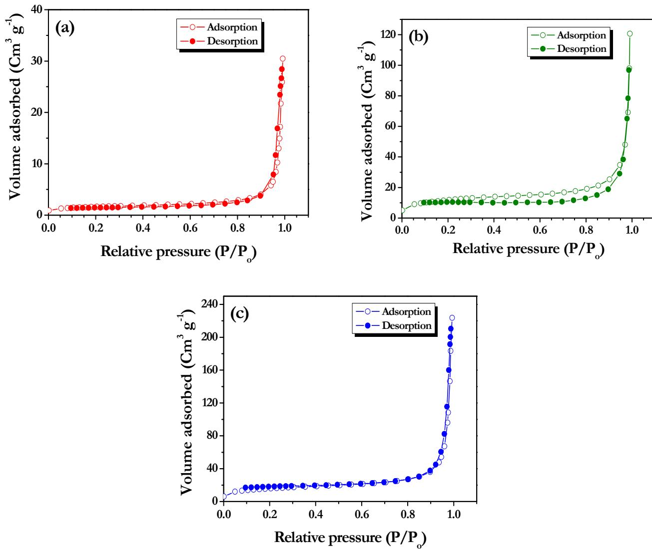
**Figure S1.**  $\text{N}_2$  adsorption/desorption isotherms (a)  $\text{Li}(\text{Mn}_{1/3}\text{Ni}_{1/3}\text{Fe}_{1/3})\text{O}_2$  (b)  $\text{Li}(\text{Mn}_{1/3}\text{Ni}_{1/3}\text{Fe}_{1/3})\text{O}_2\text{-PPy}$  and (c)  $\text{Li}(\text{Mn}_{1/3}\text{Ni}_{1/3}\text{Fe}_{1/3})\text{O}_2\text{-PANI}$  composite materials.
