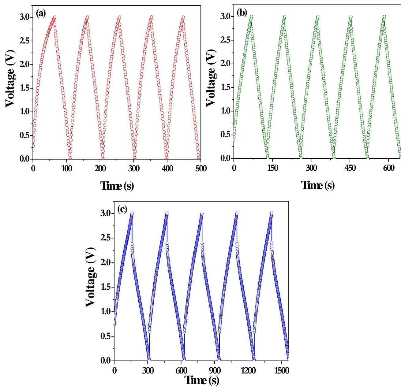
**Figure S3.** Charge discharge curves of (a)  $\text{Li}(\text{Mn}_{1/3}\text{Ni}_{1/3}\text{Fe}_{1/3})\text{O}_2/\text{AC}$  (b)  $\text{Li}(\text{Mn}_{1/3}\text{Ni}_{1/3}\text{Fe}_{1/3})\text{O}_2\text{-PPy}/\text{AC}$  and (c)  $\text{Li}(\text{Mn}_{1/3}\text{Ni}_{1/3}\text{Fe}_{1/3})\text{O}_2\text{-PANI}/\text{AC}$  cells recorded at 0.72  $\text{A g}^{-1}$  current density between 0–3 V in 1 M  $\text{LiPF}_6/\text{EC:DMC}$  (1:1 v/v.) electrolyte.
