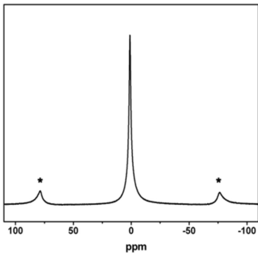
**Fig. S6**  ${}^7\text{Li}$  MAS NMR spectrum of PAF-18-OLi exhibiting a single resonance at  $\delta = 0.80$  ppm.
