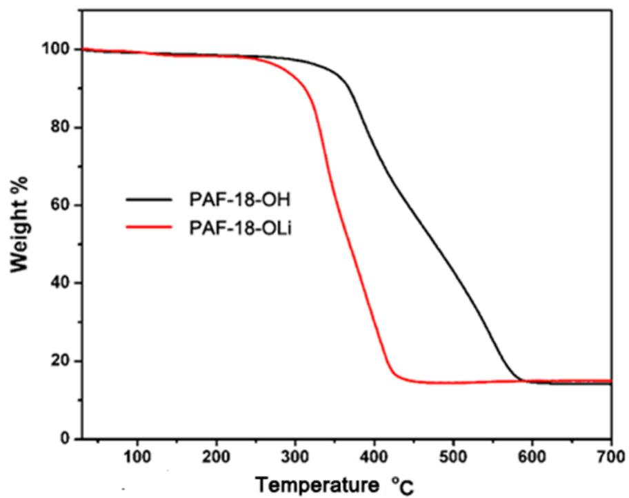
**Fig. S4** TG curves of PAF-18-OH and PAF-18-OLi samples.
