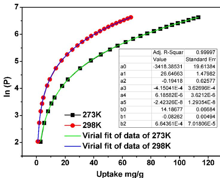
**Fig. S9** CO<sub>2</sub> adsorption isotherms of PAF-18-OH at 273K and 298K and the corresponding fittings based on the virial equation.
