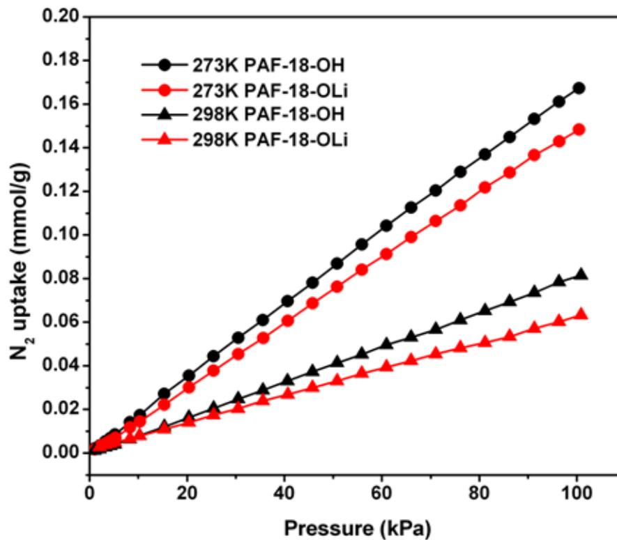
**Fig. S8** N<sub>2</sub> adsorption isotherms of PAF-18-OH and PAF-18-OLi at 273 K and 298 K.
