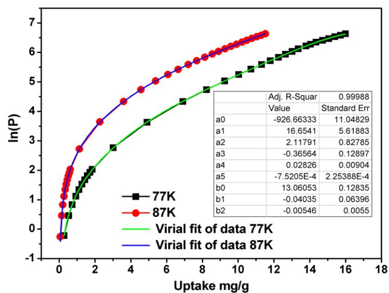
**Fig. S12** Hydrogen adsorption isotherms of PAF-18-OLi at 77 K and 87 K and the corresponding fittings based on the virial equation.
