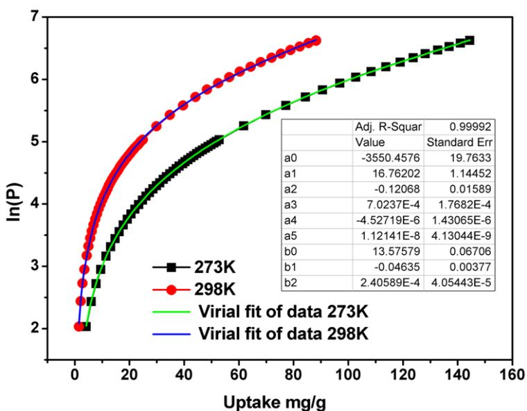
**Fig. S10** CO<sub>2</sub> adsorption isotherms of PAF-18-OLi at 273K and 298K and the corresponding fittings based on the virial equation.
