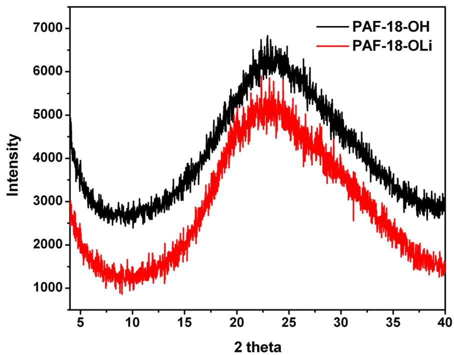
**Fig. S1** PXRD patterns of PAF-18-OH and PAF-18-OLi samples.
