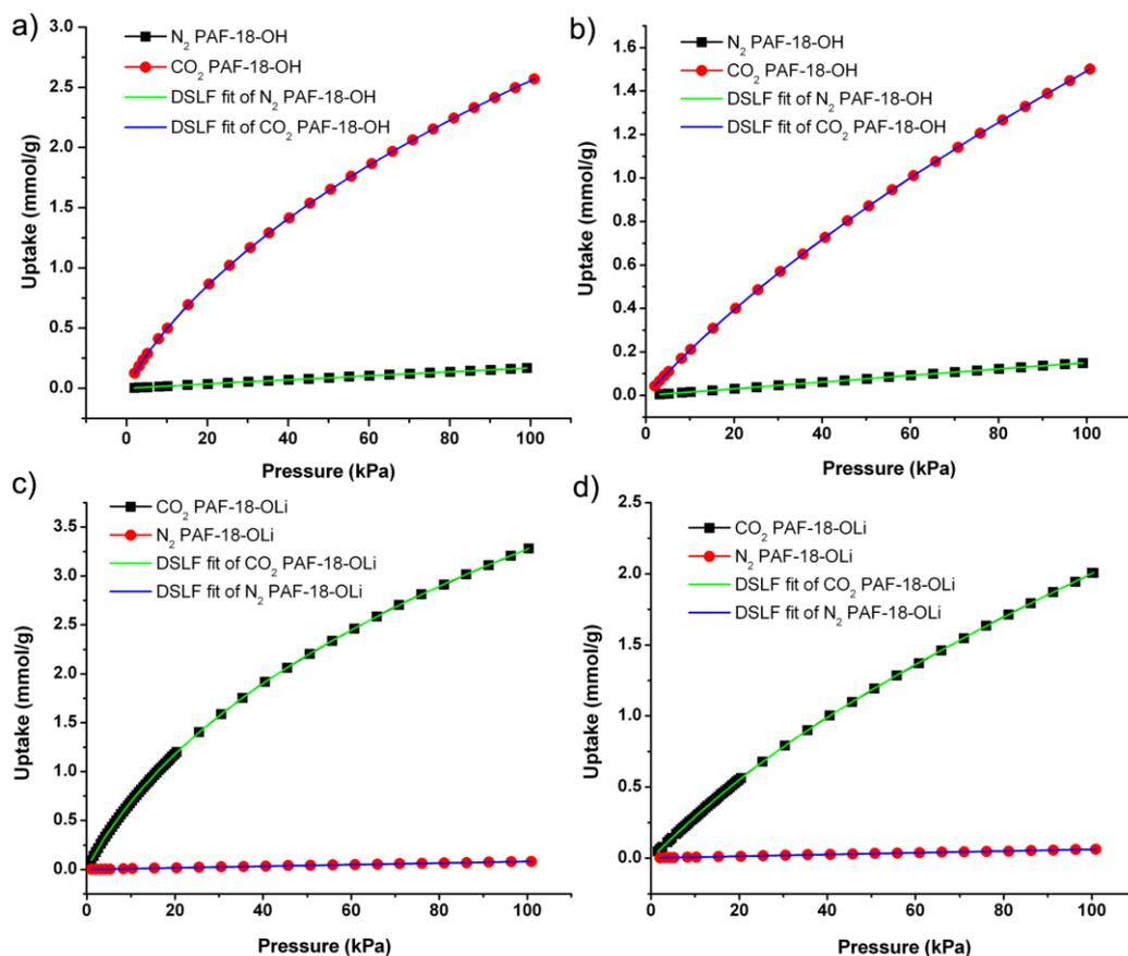
**Fig. S13** The adsorption isotherms of pure component CO<sub>2</sub> and N<sub>2</sub> for PAF-18-OH at 273K (a) and 298K (b), and for PAF-18-OLi at 273K (c) and 298K (d). Isotherms are fitted using the dual-site Langmuir-Freundlich equation.
