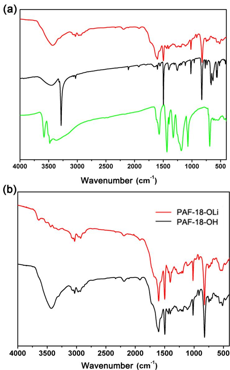
**Fig. S3** (a) FTIR spectra of tetrakis(4-ethynylphenyl)methane (black), 2,4,6-tribromo-benzene-1,3,5-triol (green) and PAF-18-OH (red), (b) FT-IR spectra of PAF-18-OH and PAF-18-OLi products.
