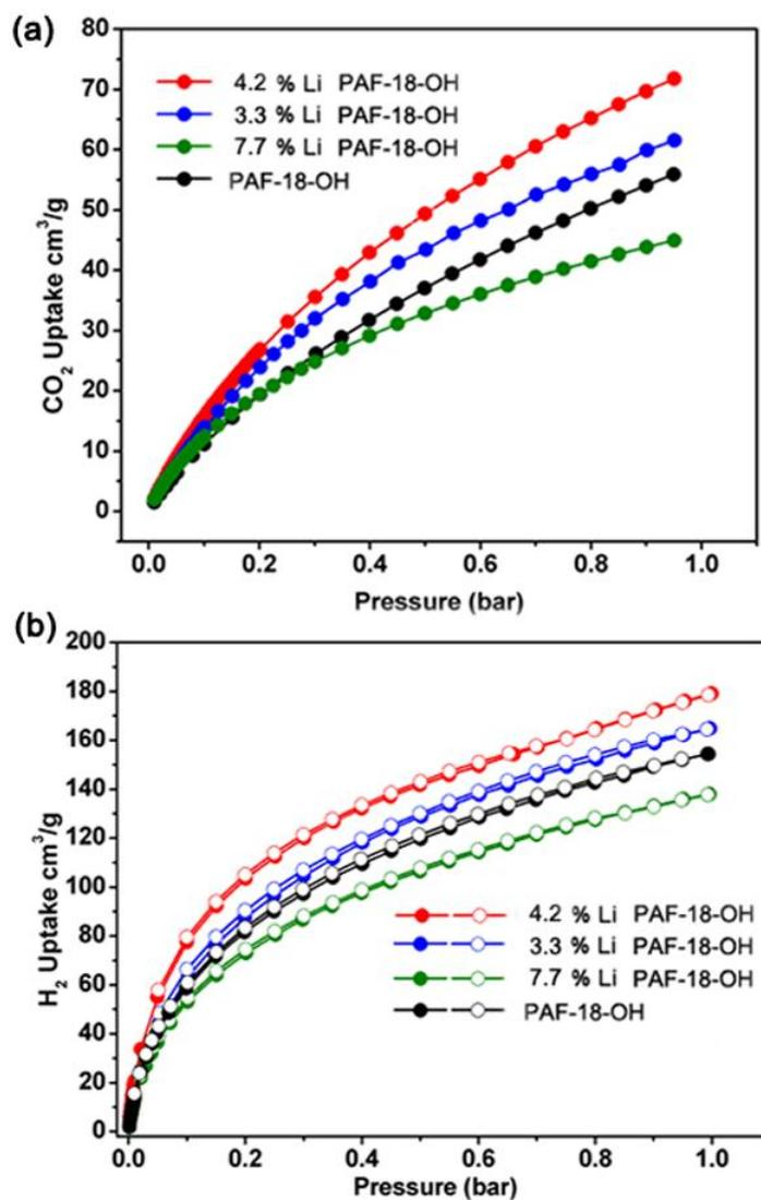
**Fig. S7** Plots of CO<sub>2</sub> (a) and H<sub>2</sub> (b) adsorption isotherms on PAF-18-OH and PAF-18-OLi with different Li contents.
