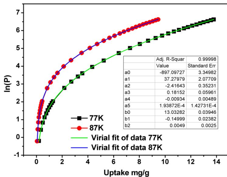
**Fig. S11**  $H_2$  adsorption isotherms of PAF-18-OH at 77 K and 87 K and the corresponding fittings based on the virial equation.
