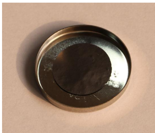
Figure S4. A photograph of the free-standing H-Fe 3 O 4 /GS-2 electrode.
