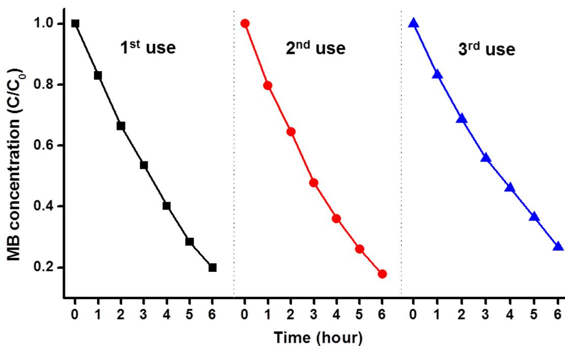
**FIGURE S10.** Photocatalytic activity of CeO<sub>2</sub> sheets calcinated at 573 K during repeated usage under visible light. The CeO<sub>2</sub> sheets were collected by filtration, rigorously washed with deionized water after each reaction, and dispersed in a MB solution (26.7 μM).
