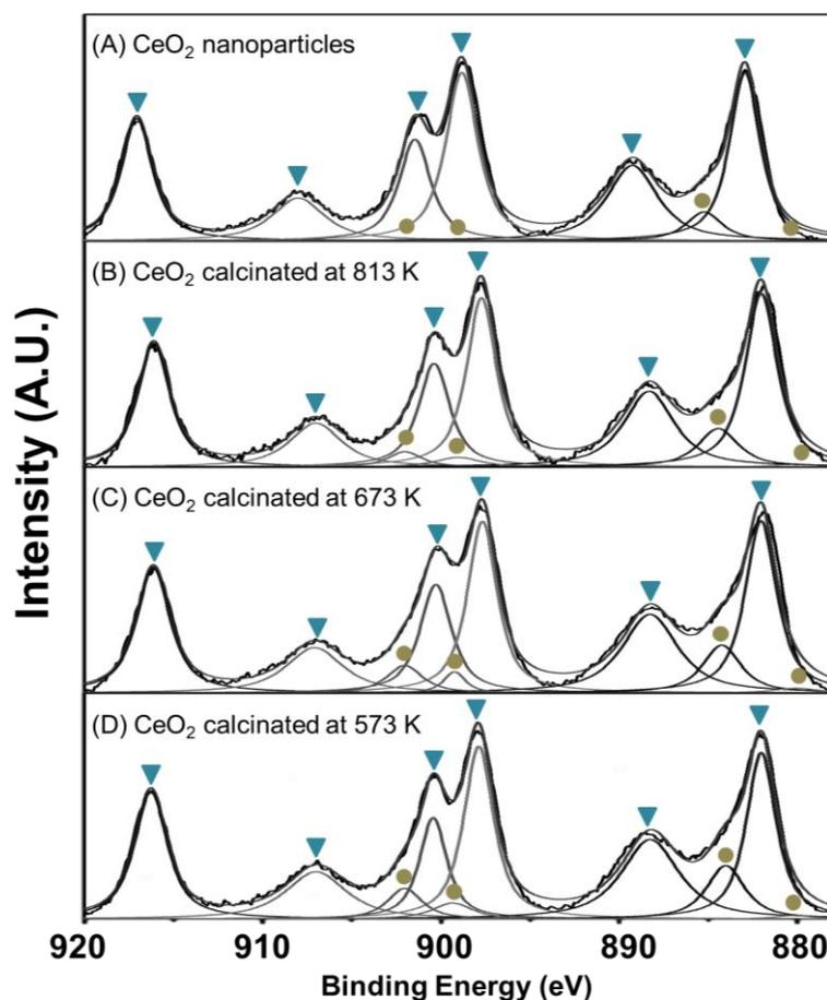
**FIGURE S8.** XPS spectra of nano-grained CeO<sub>2</sub> sheets and CeO<sub>2</sub> nanoparticles. The peaks between 895 and 910 eV originated from Ce 3d<sub>3/2</sub>, while peaks from 875 to 890 eV correspond to Ce 3d<sub>5/2</sub>. The peaks at 880.1, 885.2, 899.2, and 902.0 eV are attributed to Ce<sup>3+</sup> (circles) and the characteristic peaks of Ce<sup>4+</sup> (triangles) are centered at 882.1, 888.1, 898.0, 900.8, 906.8, and 916.3 eV.
