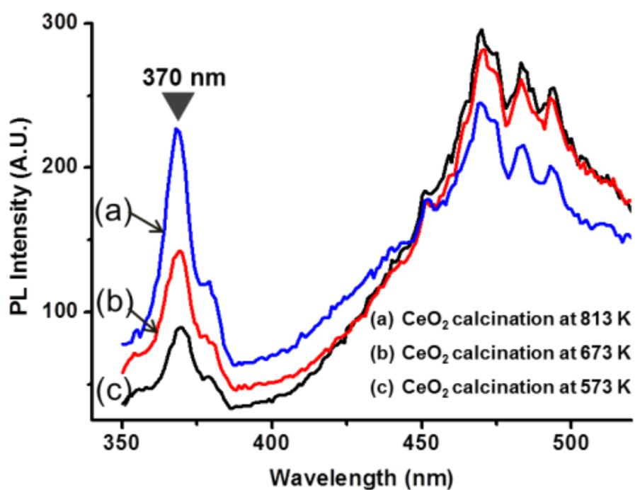
**FIGURE S9.** Room-temperature photoluminescence spectra of nano-grained CeO<sub>2</sub> calcinated at (a) 813, (b) 673, and (c) 573 K obtained with an excitation wavelength of 265 nm. The spectra show strong emission peaks at 370 nm and around 475 nm.
