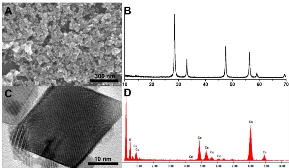
**FIGURE S7.** (A) SEM image and (B) XRD pattern of CeO<sub>2</sub> nanoparticles (purchased from Sigma-Aldrich Co., < 25 nm). (C) TEM image of the CeO<sub>2</sub> nanoparticles. (D) Energy dispersive X-ray spectroscopy spectrum of CeO<sub>2</sub> nanoparticles, which shows the existence of cerium and oxygen atoms. Note that copper atoms came from the TEM grid that was used for supporting the sample.
