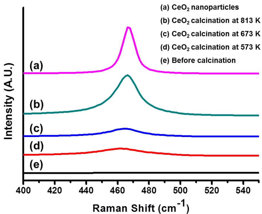
**FIGURE S6.** Raman spectra of (a) CeO<sub>2</sub> nanoparticles and nano-grained CeO<sub>2</sub> sheets calcinated at (b) 813, (c) 673, and (d) 573 K. The spectra show different degrees of Raman peak-broadening of a symmetric stretching mode of Ce-8O vibrational unit at around 466.28 cm<sup>-1</sup>.
