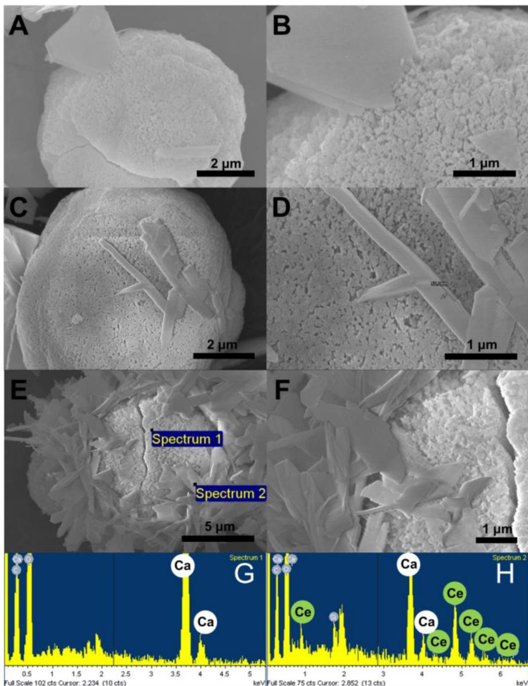
**FIGURE S2.** SEM images of PDA-induced  $\text{CaCO}_3$  microspheres incubated in an  $\text{CeCl}_3$  solution for 30 mins (A, B), 60 mins (C, D) and 90 mins (E, F). Energy-dispersive X-ray spectroscopic analysis of (G) deformed area of a vaterite microsphere and (H) newly formed sheet on the surface of the vaterite microsphere.
