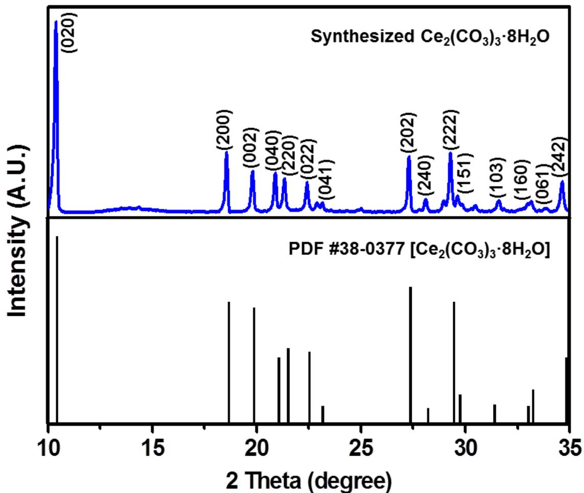
**FIGURE S4.** XRD pattern of sheet-like precipitates obtained from PDA-induced  $\text{CaCO}_3$  vaterite microspheres incubated in  $\text{CeCl}_3$  solution for 2 hours, which shows diffraction peaks corresponding to orthorhombic structure of  $\text{Ce}_2(\text{CO}_3)_3 \cdot 8\text{H}_2\text{O}$  (JCPDS No. 38-0377).
