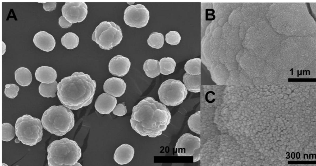
**FIGURE S1.** (A) SEM image of PDA-induced vaterite phase  $\text{CaCO}_3$  microspheres. (B, C) Magnified SEM images showing that amorphous calcium carbonate (ACC) nanoparticles are well clustered to form spherical vaterite phase of  $\text{CaCO}_3$  microstructure.
