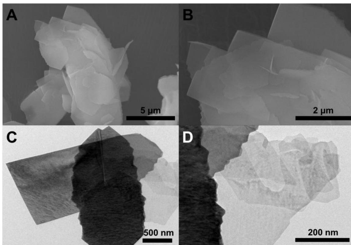
**FIGURE S3.** (A, B) SEM and (C, D) TEM images of sheet-like structure of  $\text{Ce}_2(\text{CO}_3)_3 \cdot 8\text{H}_2\text{O}$  obtained with PDA-induced  $\text{CaCO}_3$  vaterite microspheres after incubation under  $\text{CeCl}_3$  solution for 2 hours are shown in different scales. Vaterite microspheres were completely dissolved and  $\text{Ce}_2(\text{CO}_3)_3 \cdot 8\text{H}_2\text{O}$  sheets were formed.
