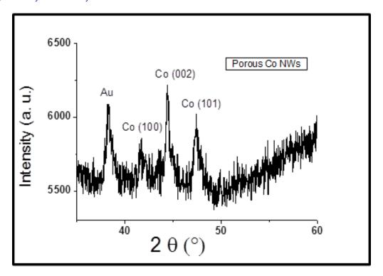
SI1. XRD pattern of porous Co NWs (r = 100 nm;  $R_1 = 35$  nm). The gold is attributed to the metallic contact used during electrodeposition.
