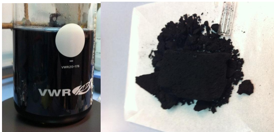
Fig. S1. Digital pictures of as prepared Sn-rGO (Please note that this procedure was repeated several times to check reproducibility and was also done with fewer amounts (1 g) of \text{SnCl}_2 )
