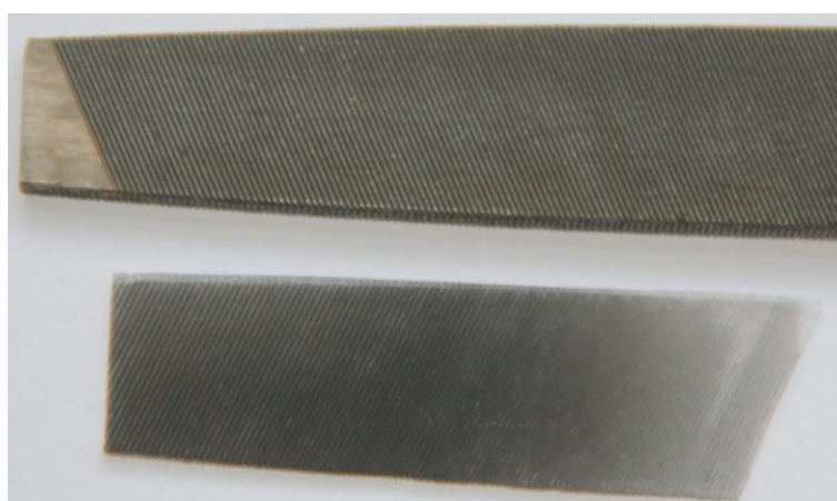
Fig. S1 Digital images of rasp (top) and the SWCNTs/PDMS obtained using rasp as substrate (bottom).
