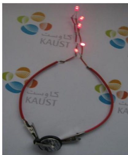
Figure S9. Demonstration of five red LEDs lighting by a PANi-NT pseudocapacitor in EMIMBF 4 electrolyte after a long-term cycling of 10000 times under current density of 10 A/g.
