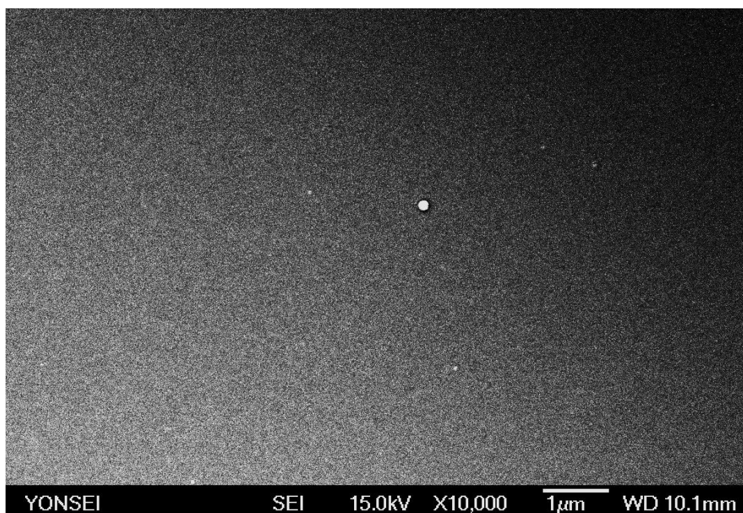
Figure S1. Scanning electron microscopy image of a thermally evaporated silver thin film.
