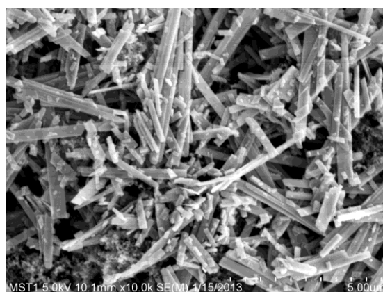
Fig.S2 A FE-SEM image of the MoO 3 contrast electrodes prepared through the conventional route.
