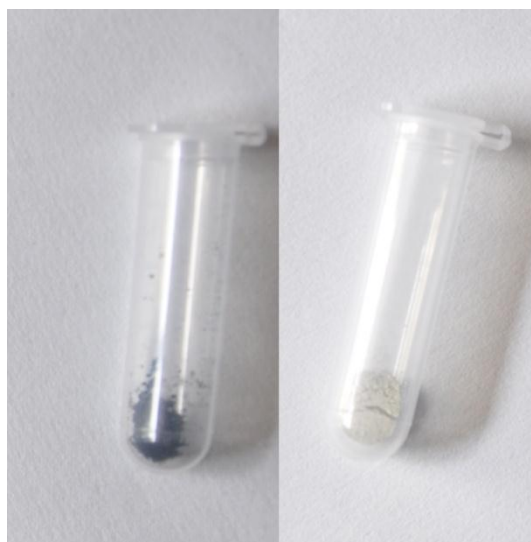
Figure S9 Photographs of A) \text{TiO}_2@\text{C}@\text{WC} ; and B) \text{WO}_3@\text{TiO}_2@\text{WO}_3 . The color of the \text{TiO}_2@\text{C}@\text{WC} is black, and after annealing in air to form \text{WO}_3@\text{TiO}_2@\text{WO}_3 , the color changed into white.
