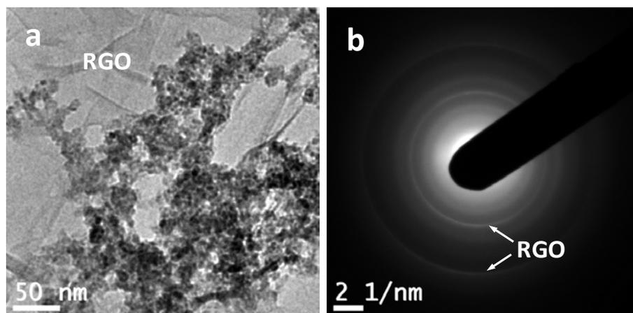
**Fig. S4** TEM image (a) and SAED pattern (b) of product prepared by reducing  $\text{SnCl}_4$  on GO using  $\text{NaBH}_4$  and the same procedure for preparing RGO—IDTO nanohybrids.
