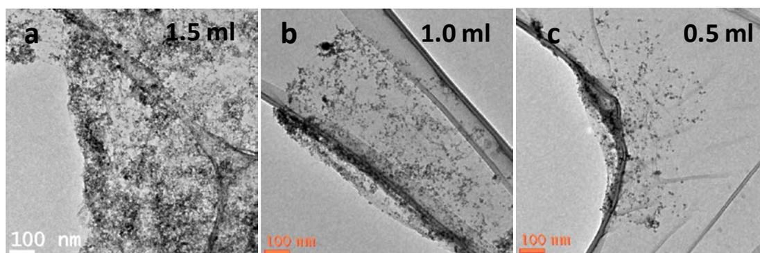
**Fig. S7** TEM images of RGO–RDTO nanohybrids prepared with different amounts of Ru by adding different amounts of  $\text{RuCl}_3$  (0.05 M) solutions (e.g., 1.5 ml, 1.0 ml and 0.5 ml) into 8 mg GO dispersion, while adding the same amount of  $\text{SnCl}_4$ .
