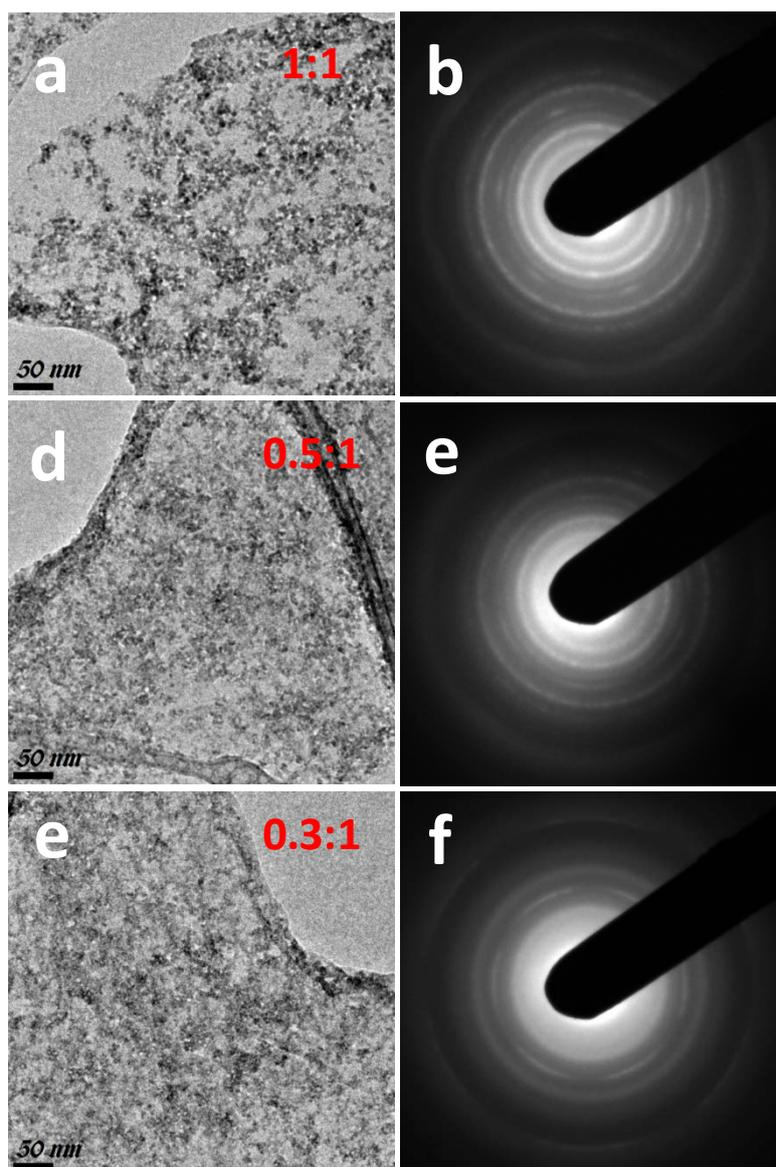
**Fig. S5** TEM images and SAED patterns of RGO-IDTO nanohybrids prepared with In/Sn=1:1 (a, b), 0.5:1 (c, d), 0.3:1 (e, f), respectively.
