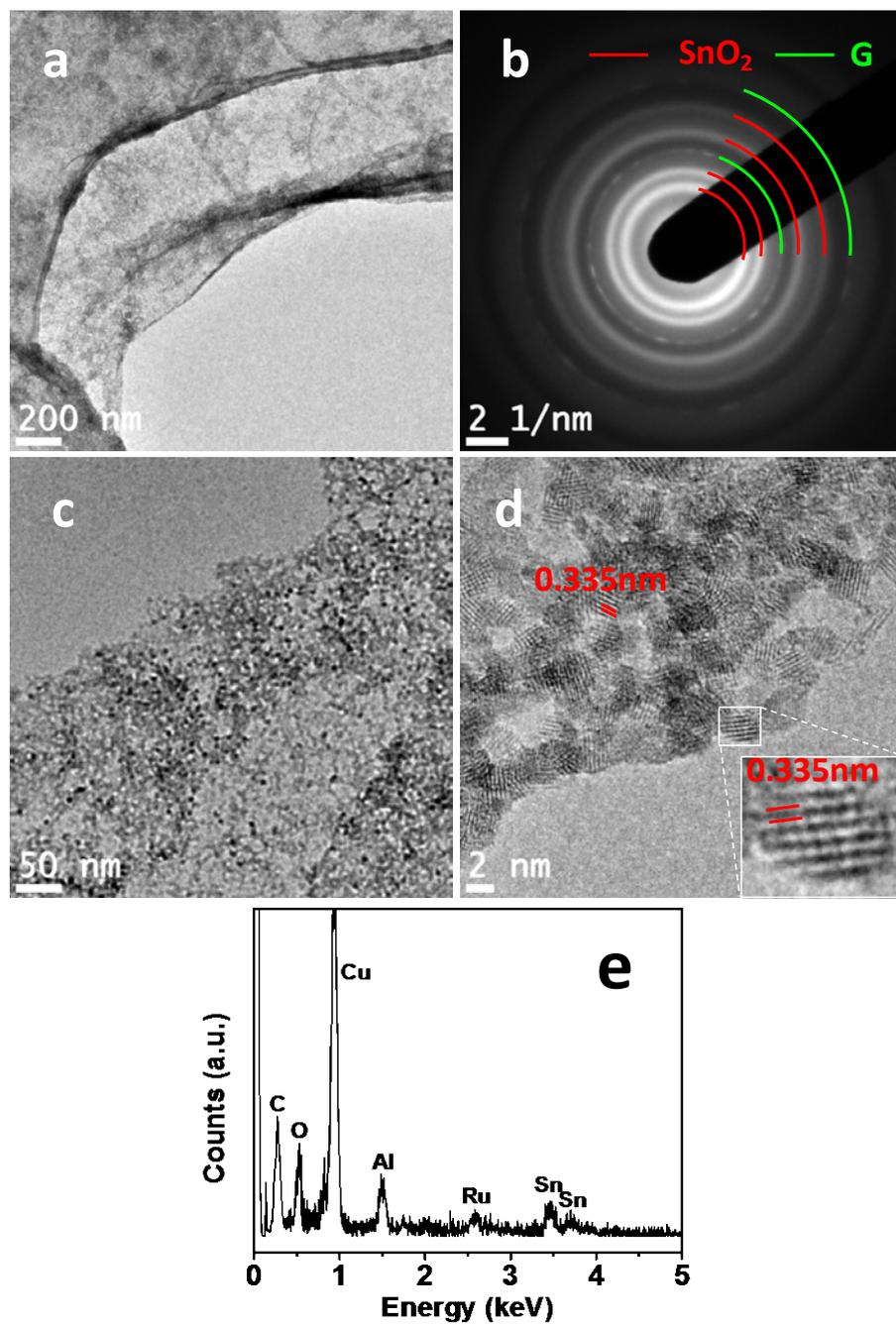
**Fig. S2** (a, c) low magnification TEM images of RGO-RDTO nanohybrids. (b) SAD pattern indexed to rutile SnO<sub>2</sub> and G. (d) HRTEM image of RGO-RDTO nanohybrids. (e) EDS spectrum of RGO-RDTO nanohybrids.
