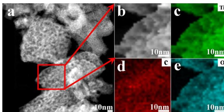
**Figure S4.** STEM images and EDX elemental maps of MPBT nanocrystals: (a) STEM image, b-e) corresponding partially STEM image and elemental maps. Elemental maps of Ti (green), C (red) and O (blue). The carbon element attributed to amorphous carbon films supported by standard Cu grids.
