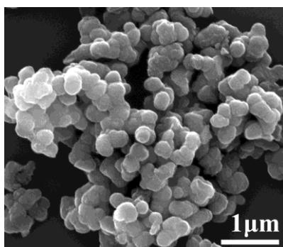
**Figure S2.** SEM image of white anatase phase TiO<sub>2</sub> (WT) nanoparticles.
