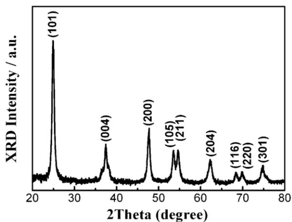
**Figure S10.** The XRD pattern of the obtained  $\text{TiO}_2$  nanoparticles by etching Ti foil without SiQDs.
