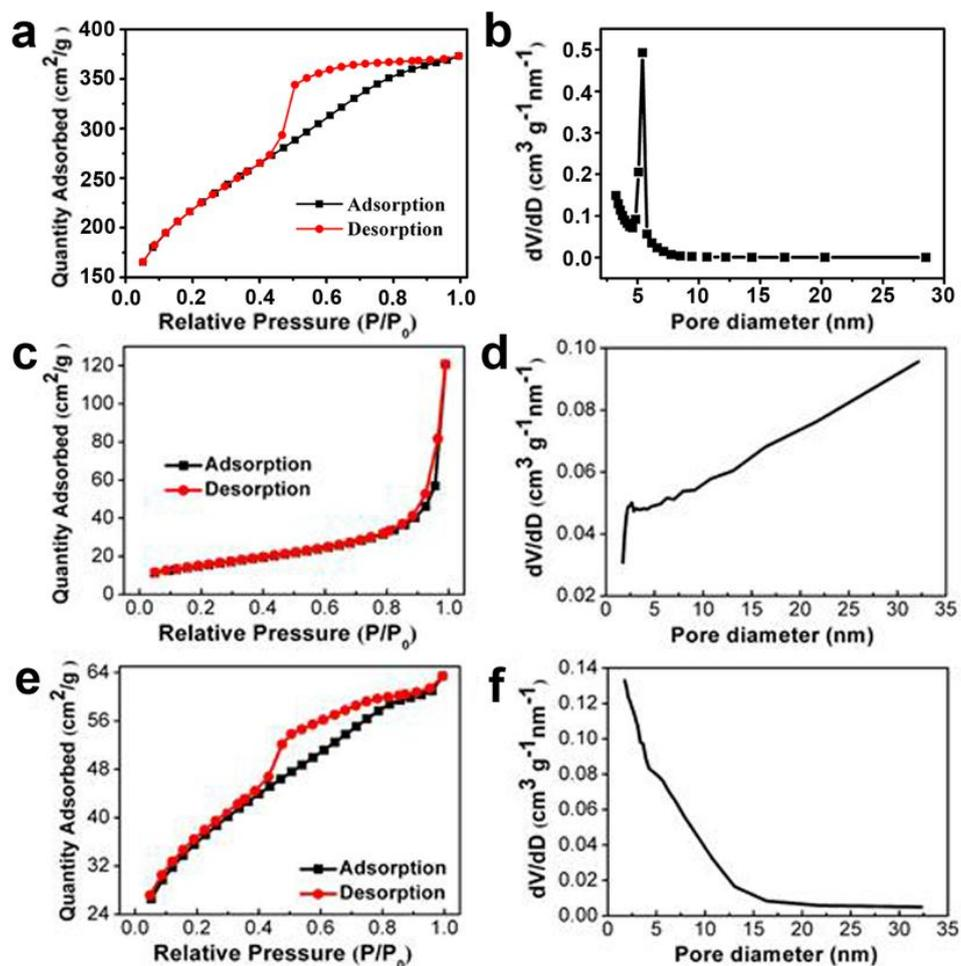
**Figure S6.** a) Nitrogen adsorption-desorption isotherm and b) pore size distribution curve of MPBT nanocrystals. c) Nitrogen adsorption-desorption isotherm and d) pore size distribution curve of BT nanoparticles. e) Nitrogen adsorption-desorption isotherm and f) pore size distribution curve of WT nanocrystals.
