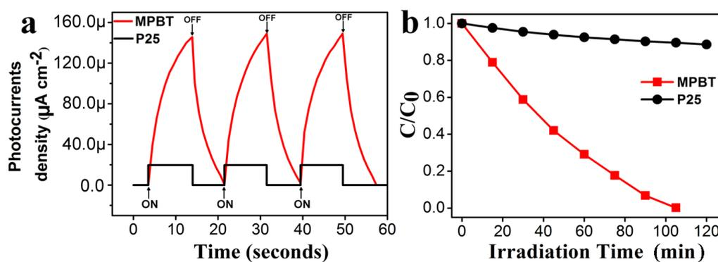
**Figure S5.** a) Photocurrent density versus time curves of MPBT nanocrystals and P25 nanoparticles measured in 0.1 M Na<sub>2</sub>SO<sub>4</sub> solution under simulated sunlight irradiation ( $I_0 = 33 \text{ mW cm}^{-2}$ ). b) Photocatalytic degradation of MO in the presence of MPBT nanocrystals and P25 nanoparticles under visible light irradiation ( $\lambda > 400 \text{ nm}$ ).
