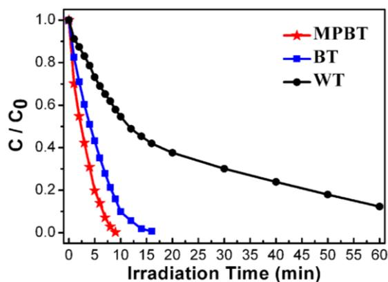
**Figure S7.** Photocatalytic degradation of MB in the presence of white anatase phase TiO<sub>2</sub> (black line), BT (blue line) and MPBT (red line) nanocrystals under visible light irradiation ( $\lambda > 400$  nm).
