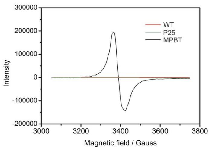
**Figure S3.** EPR spectra of WT nanoparticles, commercial P25, and MPBT nanocrystals recorded at 100 K.
