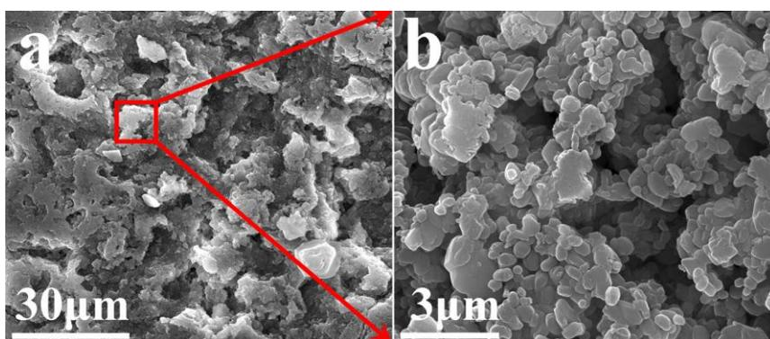
**Figure S9.** (a and b) SEM images of Ti foil after etching without SiQDs with different magnifications.
