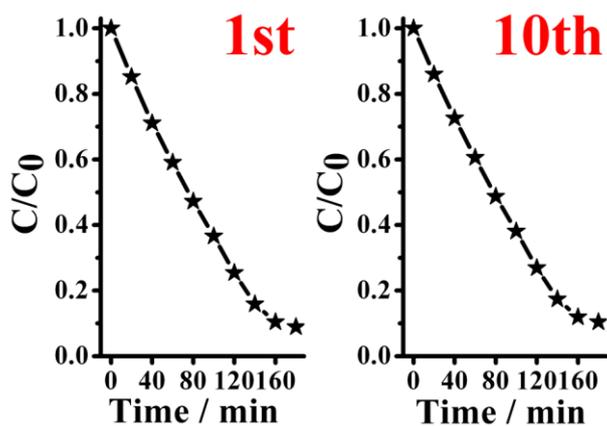
**Figure S8.** The repeatability experiments of MPBT nanocrystals in decomposing MO in ten times.
