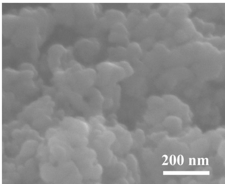
**Figure S2.** SEM image of commercial CdS nanoparticles.
