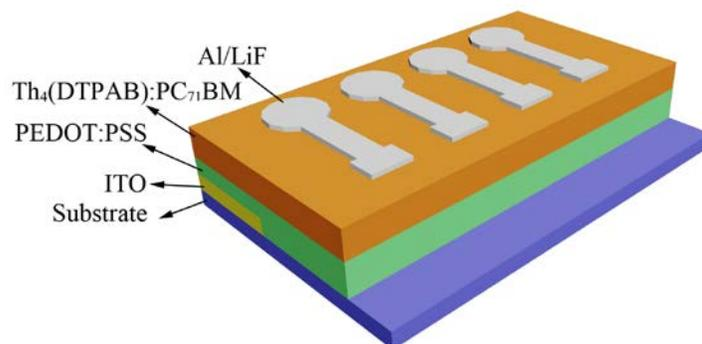
**Fig. S3.** Schematic device structure of the OSCs
