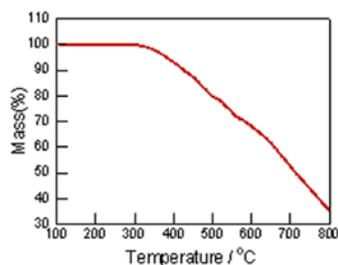
**Fig. S1.** TG curve of  $\text{Th}_4(\text{DTPAB})$  at  $10\text{ °C min}^{-1}$  under nitrogen
