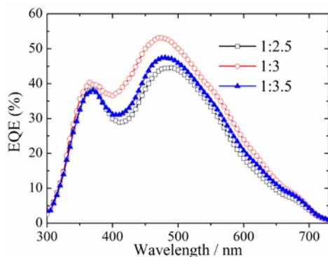
**Fig. S4.** EQEs of the OSCs based on  $\text{Th}_4(\text{DTPAB}):\text{PC}_{71}\text{BM}$  with different stoichiometries
