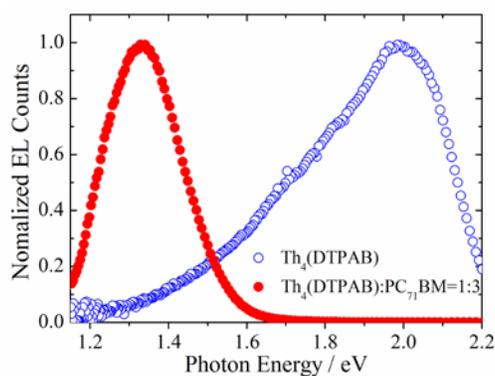
**Fig. S5.** EL spectra of  $\text{Th}_4(\text{DTPAB})$  and its blend with  $\text{PC}_{71}\text{BM}$  with the ratio of 1:3
