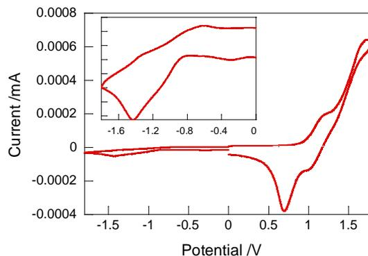
**Fig. S2.** Cyclic voltammograms of  $\text{Th}_4(\text{DTPAB})$  film on glass-carbon electrode in an acetonitrile solution of  $0.1\text{ mol L}^{-1}$  TBAP with a scan rate of  $50\text{ mV/s}$ .
