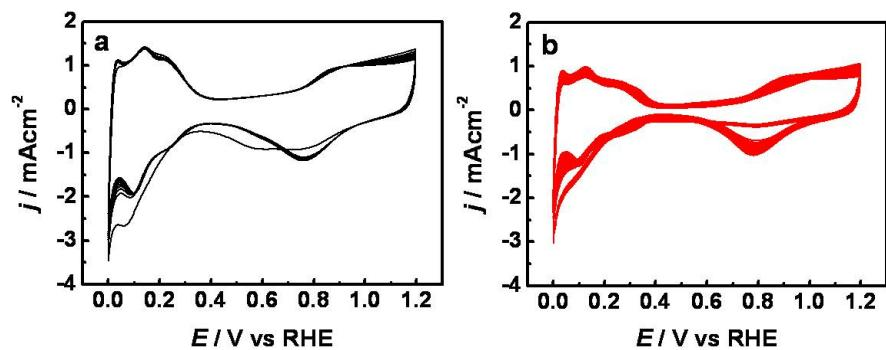
**Fig. S6** Initial 10 consecutive CV curves for commercial Pt/C (a) and Pt foam/C (b) in N<sub>2</sub>-purged HClO<sub>4</sub> (0.1 M) aqueous solution at 25 °C (0-1.2 V vs RHE, sweep rate 100 mVs<sup>-1</sup>).
