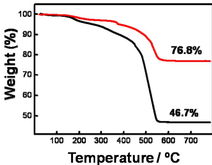
**Fig. S4** TG diagram of Pt foam/C with different metal loadings. The weight loss below 100 °C is due to the release of adsorbed water molecules, and the weight change in the range of 100-400 °C may come from Pt-catalyzed slow pyrolysis of carbon species, and the sharp weight loss beginning at 400 °C likely corresponds to the burning of carbon.
