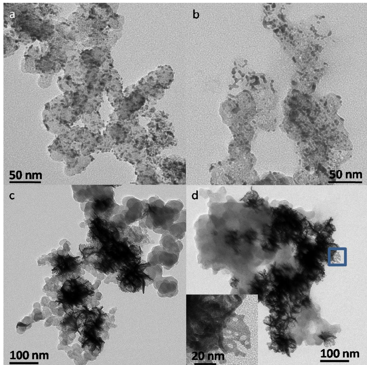
**Fig. S8** TEM images of commercial Pt/C and Pt foam/C before (a, c) and after (b, d) accelerated durability test. (Inset: magnified area selected in the blue square showing nanopores.)
