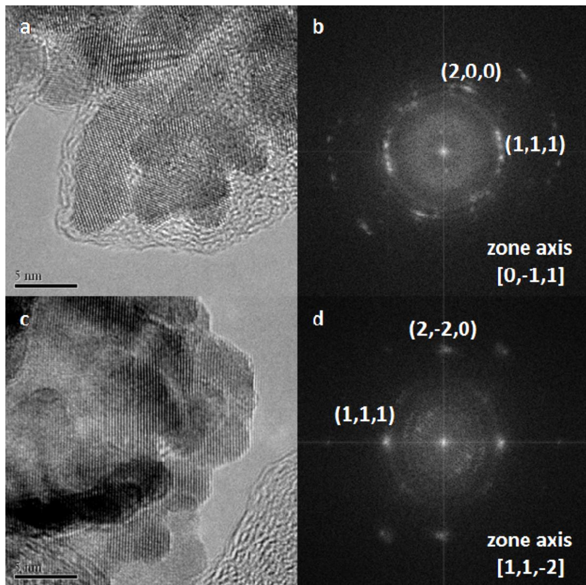
**Fig. S7** HRTEM images of randomly selected constituent dendritic nanosheets of Pt foam/C (a) and (c) and their corresponding electron diffraction patterns (b) and (d) obtained by FFT with labelled crystal planes and zone axes.
