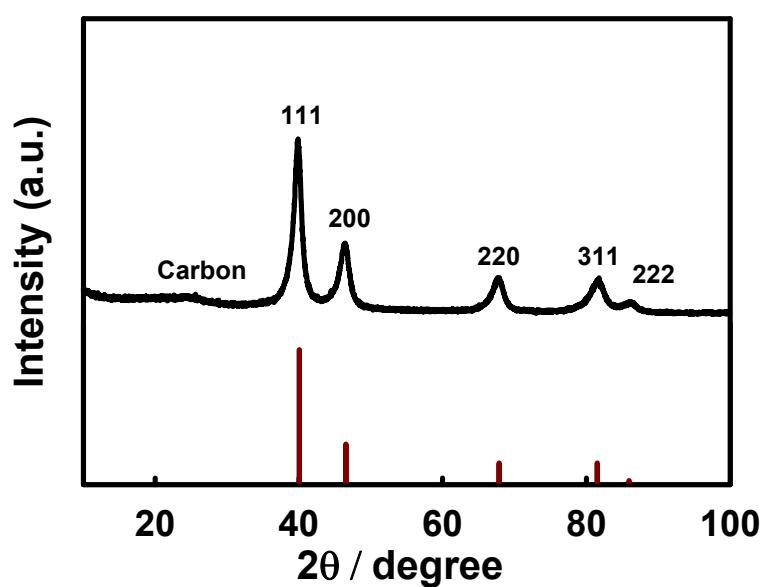
**Fig. S3** XRD pattern of the Pt foam/C accompanied by the standard XRD pattern of Pt. *Reaction conditions:* DSPC/cholesterol (5 mM, 30 mL), Vulcan XC-72 carbon black (144 mg), K<sub>2</sub>PtCl<sub>4</sub> aq. (10 mM, 30 mL), and AA (792 mg) under ambient conditions.
