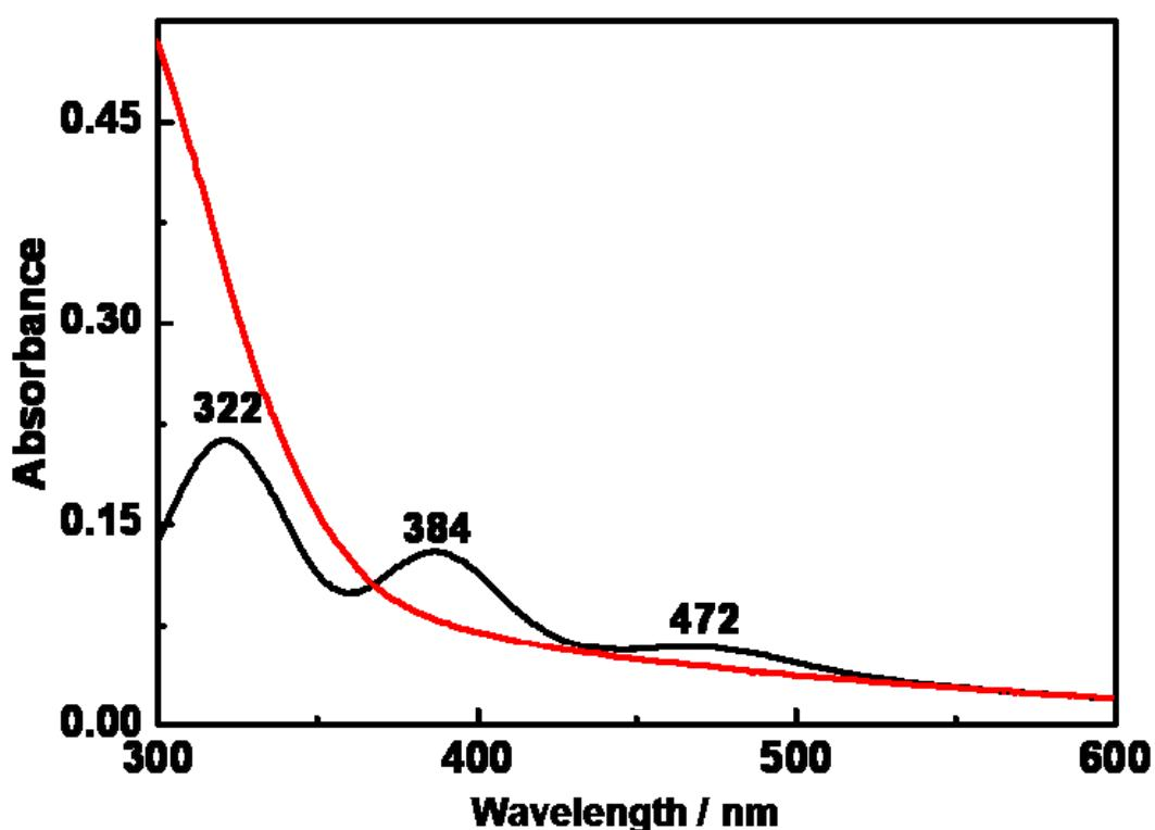
**Fig. S1** UV-visible spectrum of the supernatant of a synthetic system after 2 h of reaction (red line). A representative UV-visible spectrum of 10 mM Pt (II) aqueous solution (black line) is included to show the absorption maxima for the platinum complexes. *Reaction conditions:* DSPC/cholesterol (5 mM, 1 mL), Vulcan XC-72 carbon black (4.76 mg), K<sub>2</sub>PtCl<sub>4</sub> (20 mM, 1 mL), and AA (26.4 mg) under ambient conditions.
