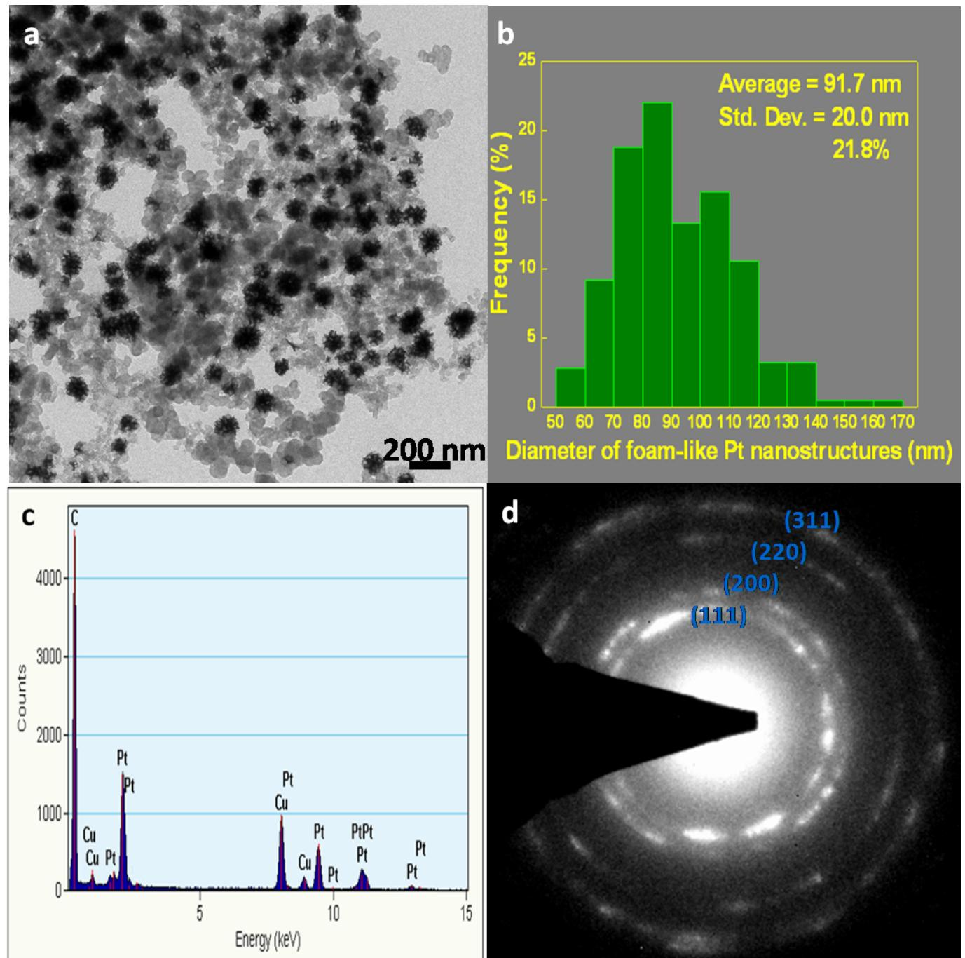
**Fig. S2** (a) TEM image of Pt foam/C, (b) plot of frequency versus diameter for more than 200 randomly selected carbon supported Pt foam with an average size, standard deviation, and percentage ratio of the standard deviation to the average size, (c) Energy-dispersive X-ray spectroscopy (EDX), and (d) selected area electron diffraction (SAED) pattern of Pt foam/C.
