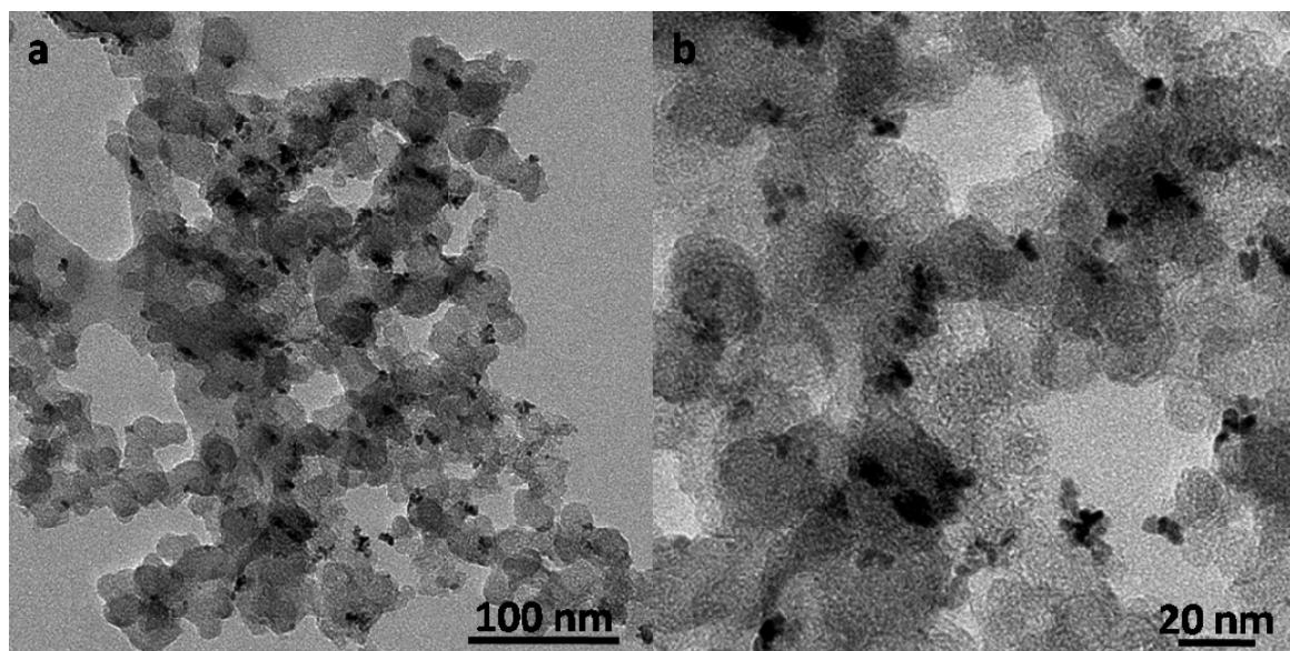
**Fig. S5** TEM image of nascent dendritic Pt nanosheets and Pt nanoparticles supported on carbon at low (a) and high (b) magnification. *Reaction conditions:* DSPC/cholesterol (5 mM, 1 mL), Vulcan XC-72 carbon black (4.76 mg), K<sub>2</sub>PtCl<sub>4</sub> (1 mM, 1 mL), and AA (26.4 mg) under ambient conditions.
