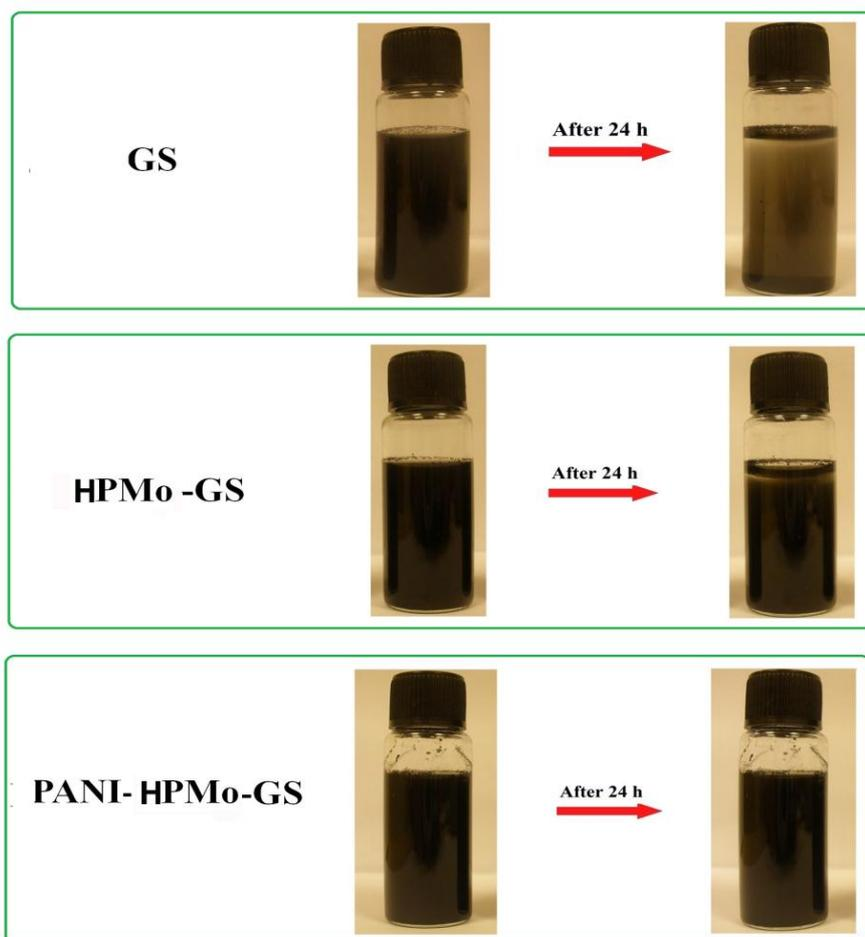
**Fig.S2.** The dispersion of GS, HPMo-GS and PANI- HPMo-GS in distilled water
