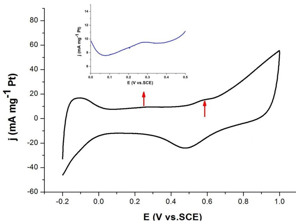
**Fig.S6.** Cyclic voltammograms of the Pt/PANI-HPMo-GS catalyst measured in 0.5 M H<sub>2</sub>SO<sub>4</sub>
