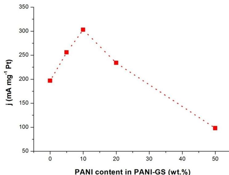
**Fig.S1.** Forward peak current densities for methanol oxidation as a function of PANI content in PANI-HPMo-GS.
