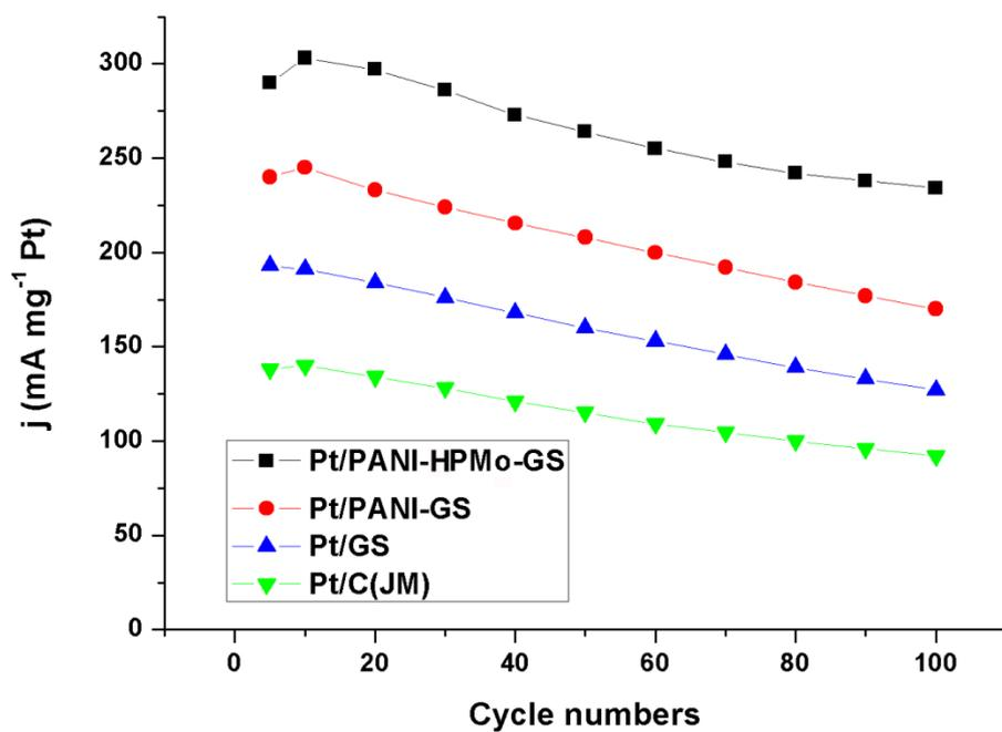
**Fig.S7.** The forward peak current densities for methanol oxidation as a function of scanning cycles measured in 1 M CH<sub>3</sub>OH + 0.5 M H<sub>2</sub>SO<sub>4</sub>.
