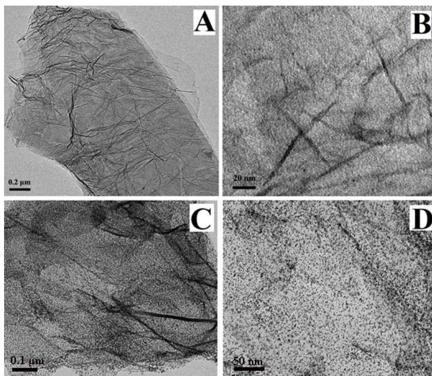
**Fig.S4.** TEM images of PANI-HPMo-GS (A and B) and Pt/PANI-HPMo-GS (C and D) at different magnifications
