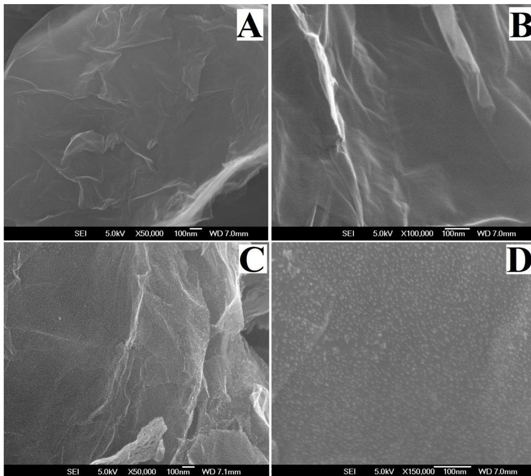
**Fig.S5.** SEM images of PANI-HPMo-GS (A and B) and Pt/PANI-HPMo-GS (C and D) at different magnifications.
