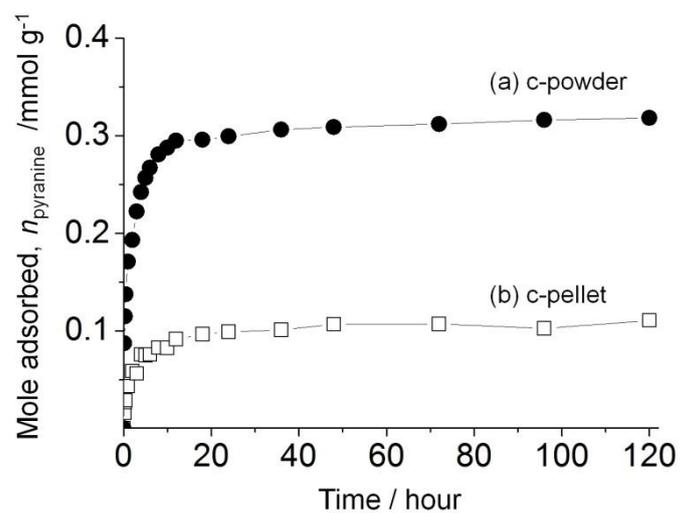
**Figure S5. Pyranine adsorption properties of c-pellet and c-powder.** Sample mass: 0.23 g; outer surface area of c-pellet: 185 mm<sup>2</sup>. The result clearly shows the diffusion limitation; c-pellet shows lower pyranine accumulation due to smaller amount of accessible reaction sites.
