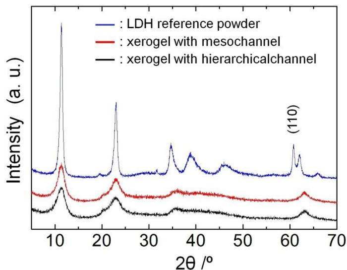
**Figure S6. XRD patterns of the reference LDH powder and xerogels.** The sharp (110) diffraction observed in LDH reference pellet indicates large in-plane dimension of crystallites. The crystalline size estimated by Scherrer's equation is 24 nm. Broad diffraction lines at  $\sim 63^\circ$  for xerogels can be assigned to supernatant of (110) and (113) diffractions, indicating small in-plane dimension of their crystallite sizes
