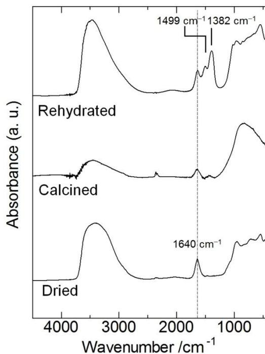
**Figure S4. FT-IR spectra of xerogel at respective steps in rehydration process.** The dotted line is guide for see. The peaks of 1499 and 1382 cm<sup>-1</sup> observed after rehydration are ascribed to CO<sub>3</sub><sup>2-</sup> ions introduced in interlayers.<sup>6</sup>
