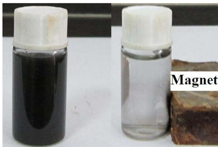
Figure S6 Photographs of  $\text{Fe}_3\text{O}_4@\text{C}$  magnetic separation phenomenon.
