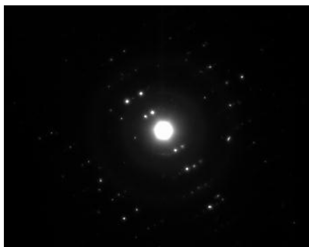
Figure S2. Selected-area electron diffraction of core shell LFP@CNTs-10h nanowire.
