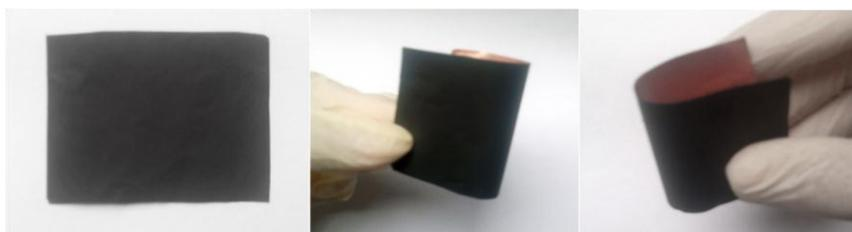
**Fig. S3** Photographs of SnS<sub>2</sub> nanocrystals@RGO substrate electrode.
