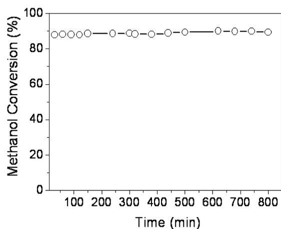
**Figure S5.** Reaction performance of SBA-15 supported Pt nanorods with time on stream.
