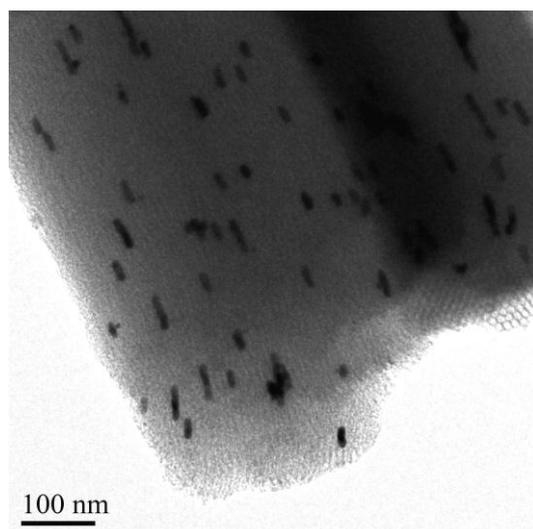
**Figure S6**, TEM image of SBA-15 supported Pt nanorods after catalytic reaction.
