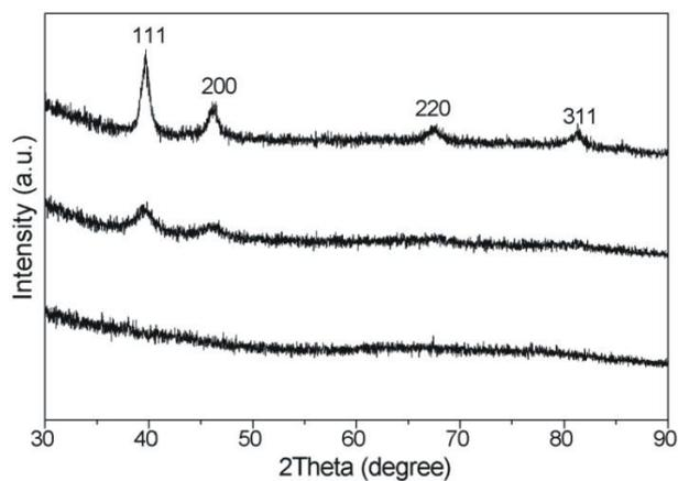
**Figure S3.** High angle XRD patterns of (a) SBA-15, and (b) Pt nanoparticles/SBA-15, (c) Pt nanorods/SBA-15.
