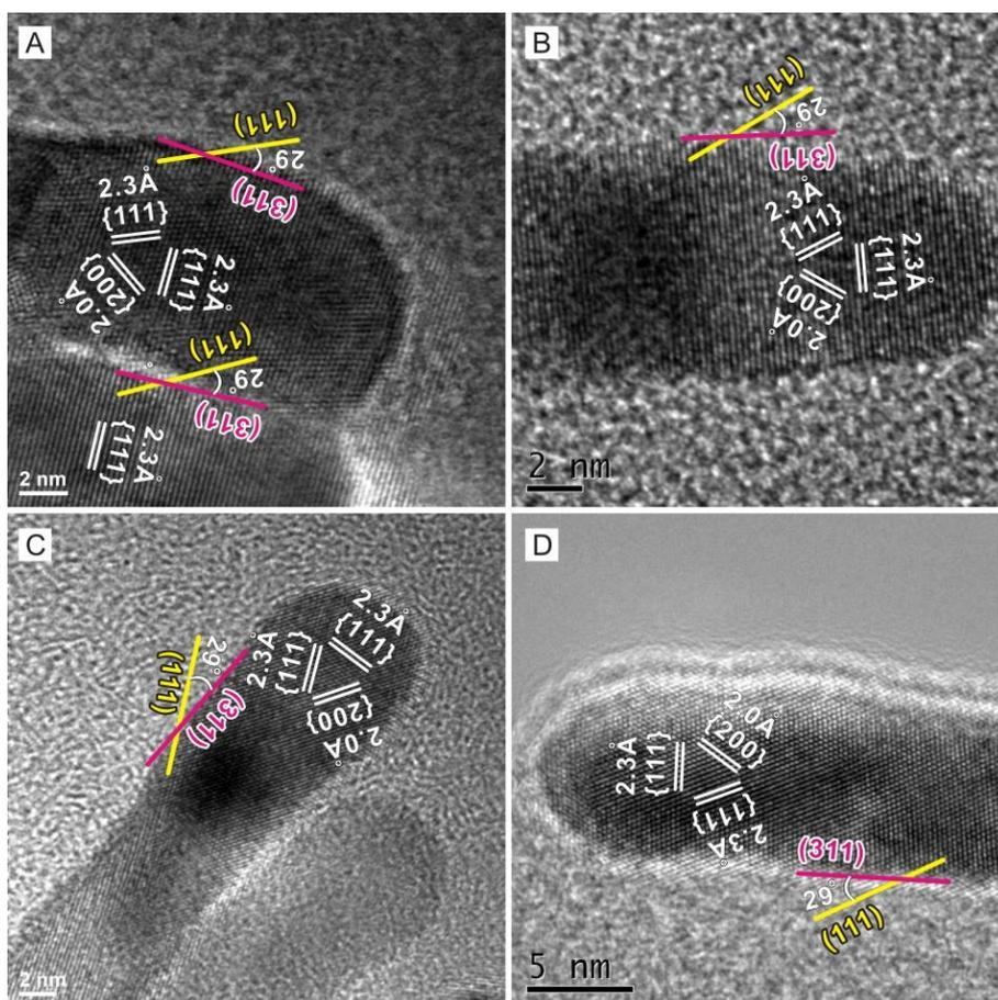
**Figure S4.** HRTEM images of Pt nanorods, all of the angles are  $29^\circ$ , corresponding to the calculated data ( $29.5^\circ$ ) of the angle between (111) and (311), illustrating the Pt nanorods are bounded by {311} facets.
