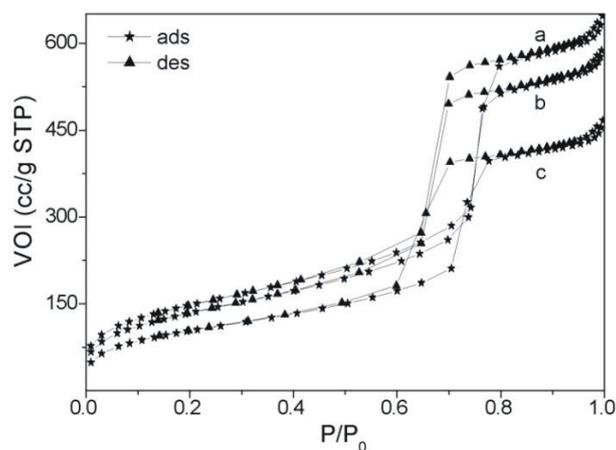
**Figure S2.** Nitrogen adsorption isotherms of (a) SBA-15, (b) Pt nanoparticles/SBA-15 and (c) Pt nanorods/SBA-15.
