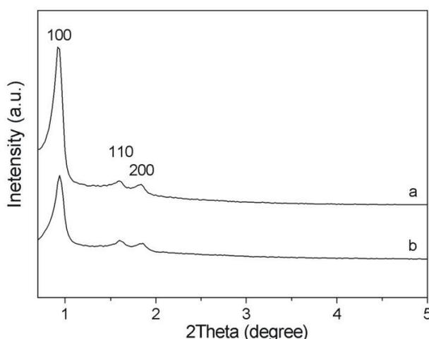
**Figure S1.** Small angle XRD patterns of (a) SBA-15 (a) before and (b) after embedding Pt nanorods.
