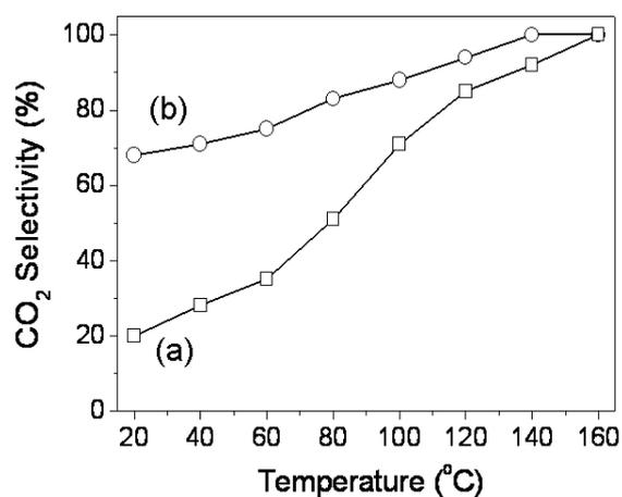
**Figure S7**. Selectivity of CO<sub>2</sub> over the SBA-15 supported Pt (a) nanorods and (b) nanoparticles catalysts.
