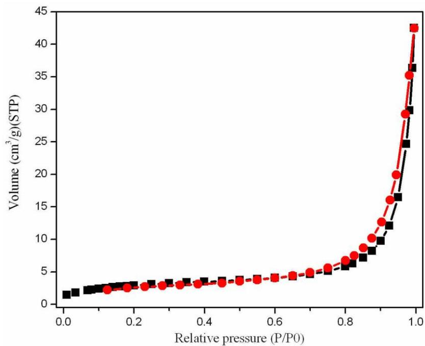
**Figure S0.** Nitrogen adsorption/desorption of the hexagonal  $\text{Zn}_2\text{GeO}_4$  nanorod-bundles obtained at 473 K for 24 h.
