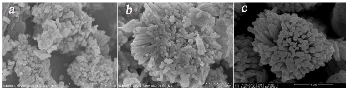
**Figure S1.** SEM images of the products obtained at 473 K with different solvothermal system: (a)  $\text{H}_2\text{O}$ -ethanolamine, (b)  $\text{H}_2\text{O}$ -diethanolamine, and (c)  $\text{H}_2\text{O}$ -triethanolamine.
