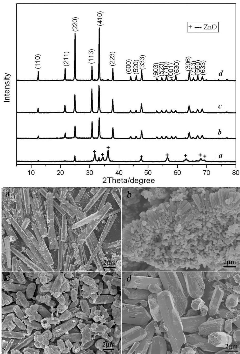
**Figure S2.** XRD patterns and SEM images of the products obtained at 473 K with different NaOH amount: (a) 0.1 g, (b) 0.25 g, (c) 0.4 g, and (d) 0.6 g.
