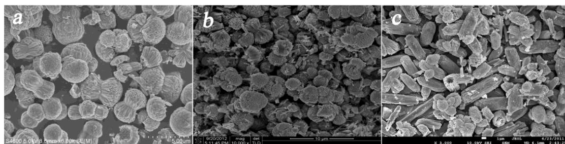
**Figure S3.** XRD patterns and SEM images of the products obtained at 473 K with different solvothermal treatment times of (a) 30 min, (b) 12 h, and (c) 24 h.
