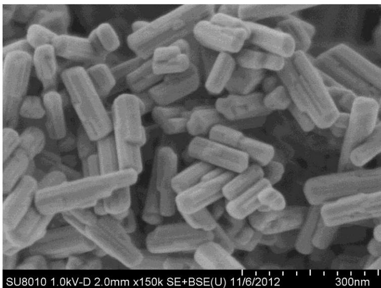
**Figure S4.** SEM images of the hexagonal Zn<sub>2</sub>GeO<sub>4</sub> nanorods prepared by a hydrothermal method.
