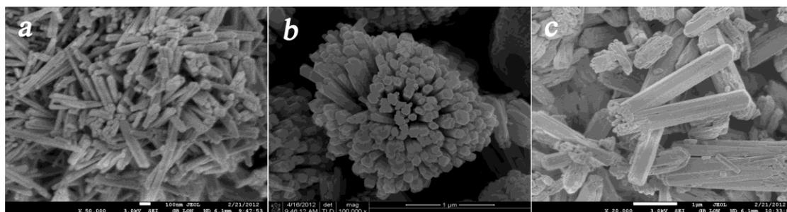
**Figure S5.** SEM images of the products obtained at 473 K with different mass ratio of H<sub>2</sub>O to TEA: (a) 18:2, (b) 15:5, and (c) 10:10.
