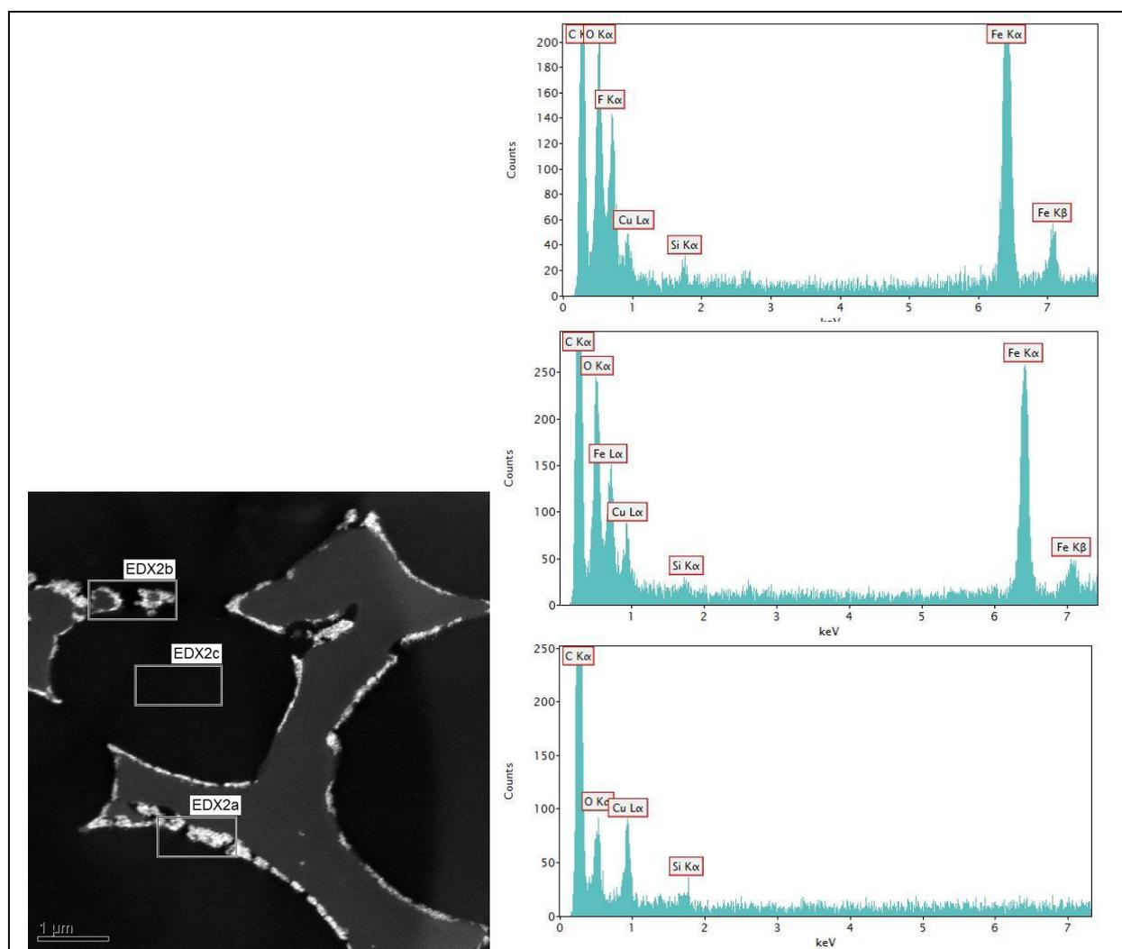
**Fig. S9** EFTEM image of pDCPD-15w-1.5v and EDX images (top: EDX2a; middle: EDX2b and below: EDX2c)
