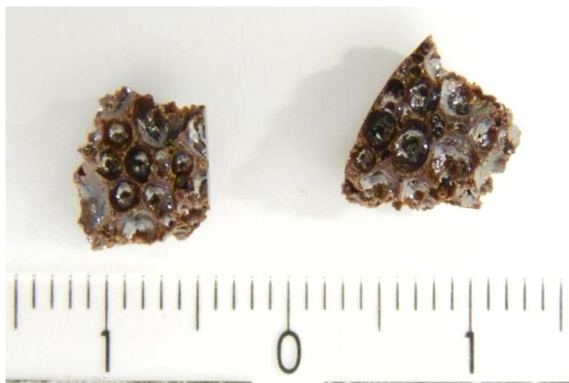
**Fig. S4** Macroscopically observed pores in **pDCPD-xw**
