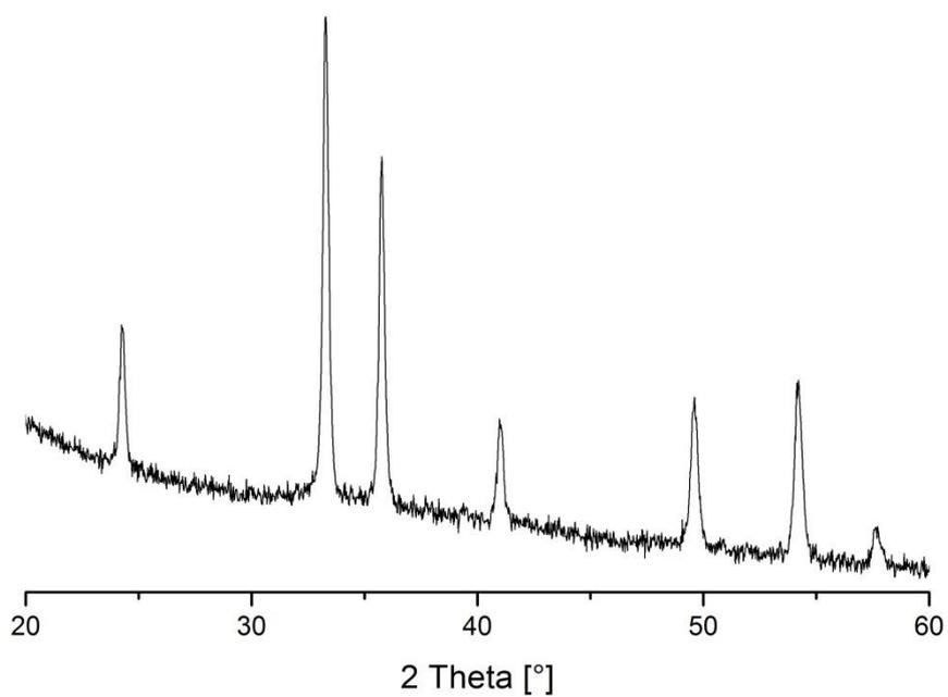
**Fig. S13** X-ray powder diffraction pattern (CuK $\alpha$ , measured on Bruker D8 Advance) of the sample **pDCPD-30w-10v** upon burning @ 550°C in pure oxygen corresponding to  $\alpha$ -Fe<sub>2</sub>O<sub>3</sub>
