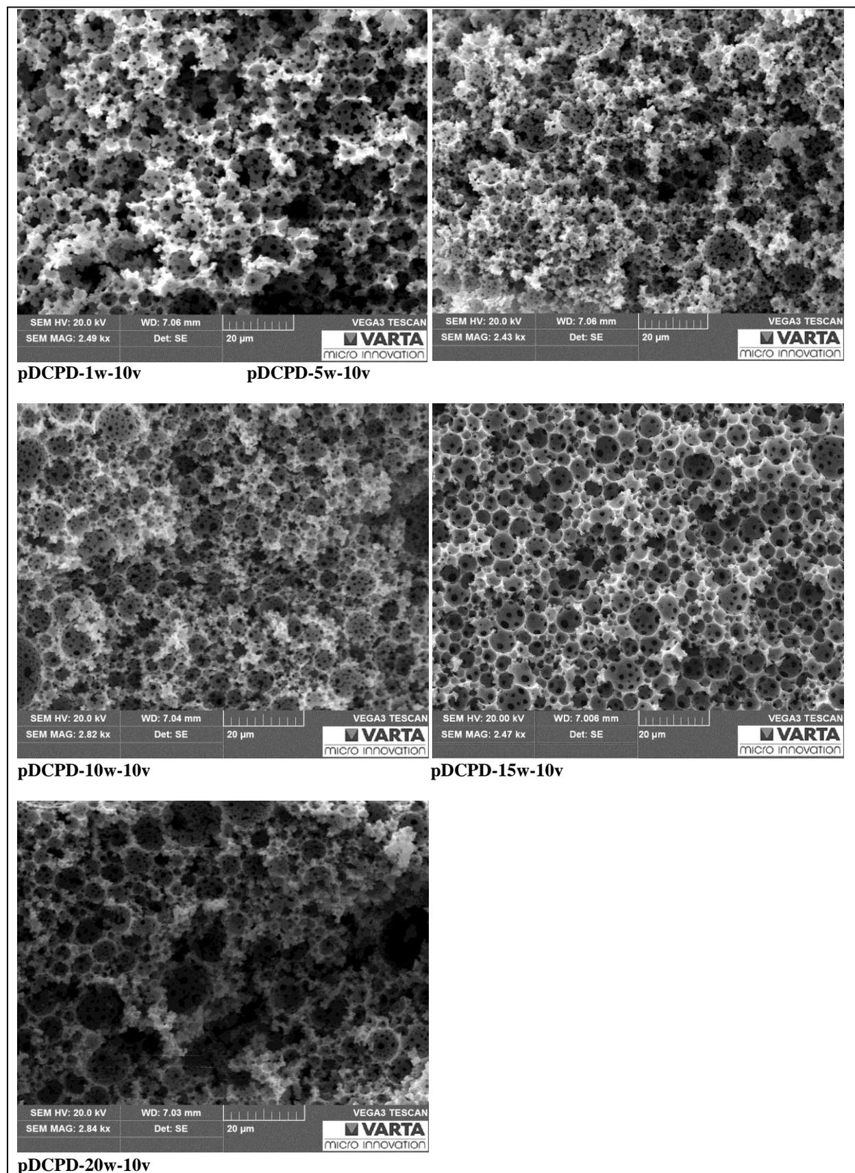
Fig. S7 SEM-pictures of the nanocomposite foams prepared with 10 v% surfactant
