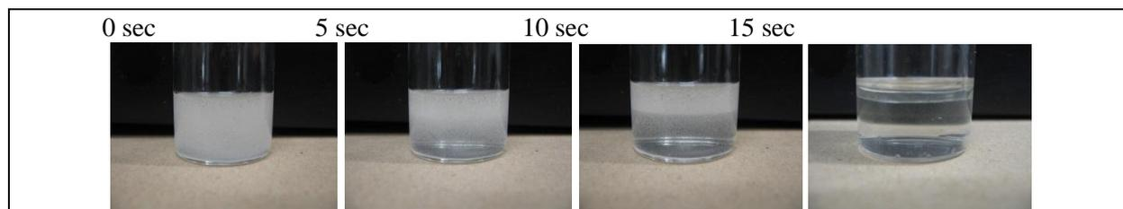
**Fig. S1** Binary mixture of **DCPD** (20 v%) and water (80 v% @ 80°C)
