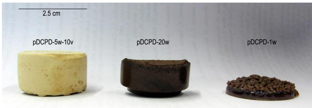
**Fig. S5** Photograph showing the quality of moulded parts; ideal shape of the mould is only obtained in case of **pDCPD-5w-10v**
