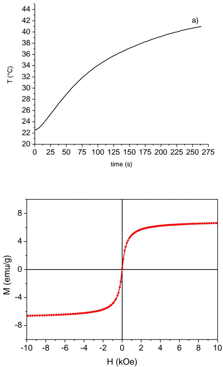
**Fig. S12** Inductive heating of **pDCPD-15w-1.5v** (above) and magnetization of **pDCPD-15w-1.5v** (below)
