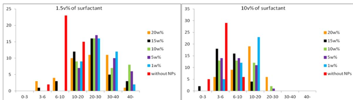
**Fig. S8** Pore size distributions of poly(DCPD)-nanocomposite-HIPEs from the corresponding SEM micrographs
