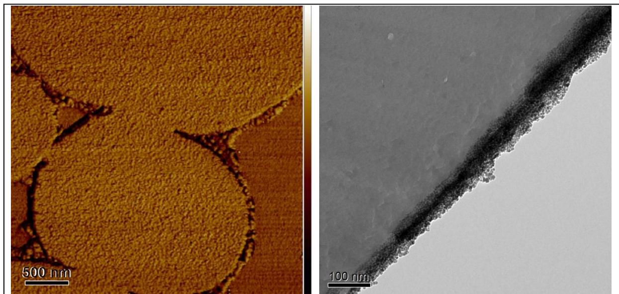
**Fig. S11** AFM and SEM pictures of pDCPD-15w-1.5v
