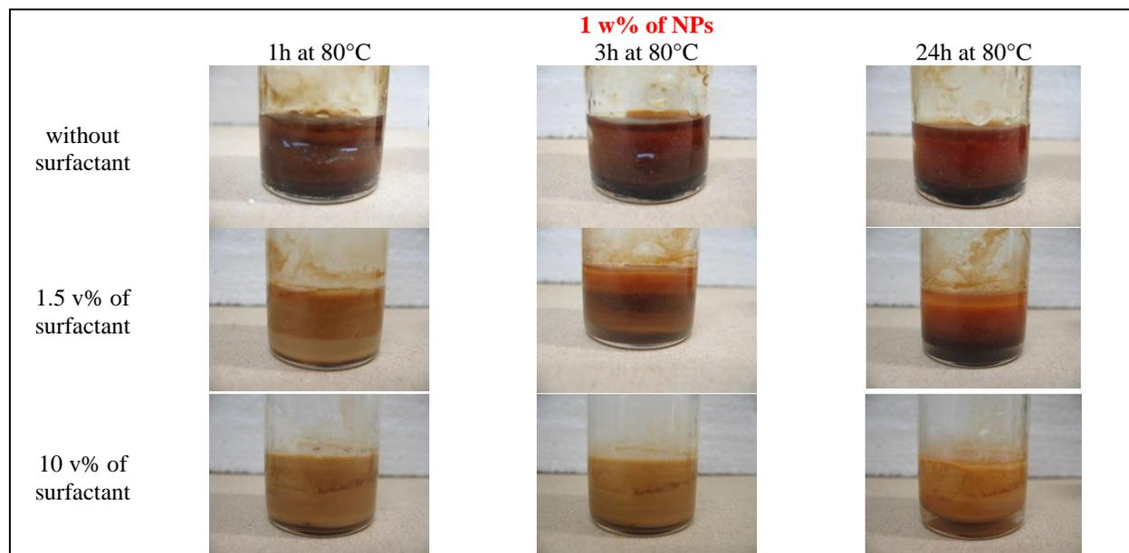
**Fig. S2** Ternary and quaternary mixtures of **DCPD** (20 v%) and water (80 v% @ 80°C)
