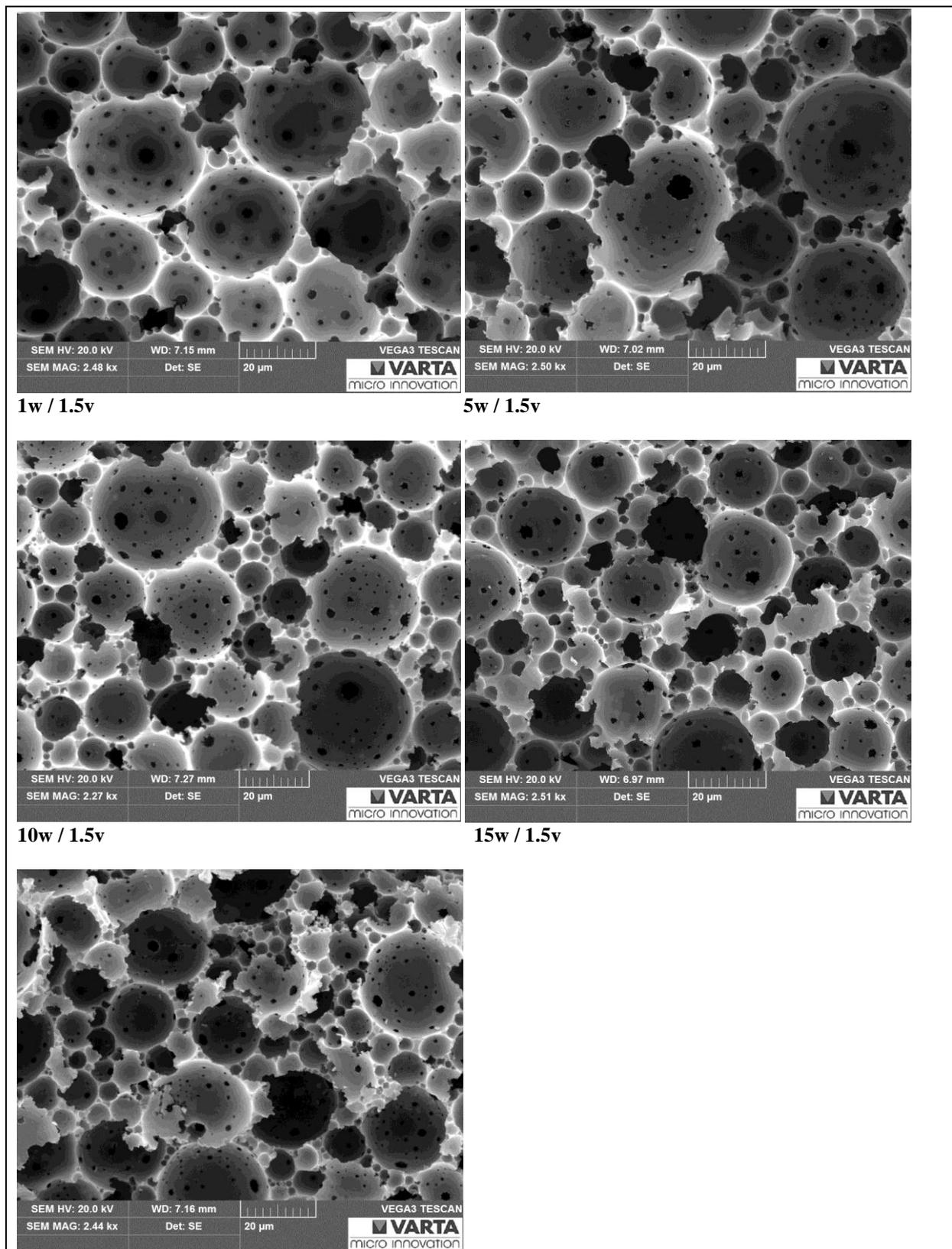
**Fig. S6** SEM-pictures of the nanocomposite foams prepared with 1.5 v% surfactant
