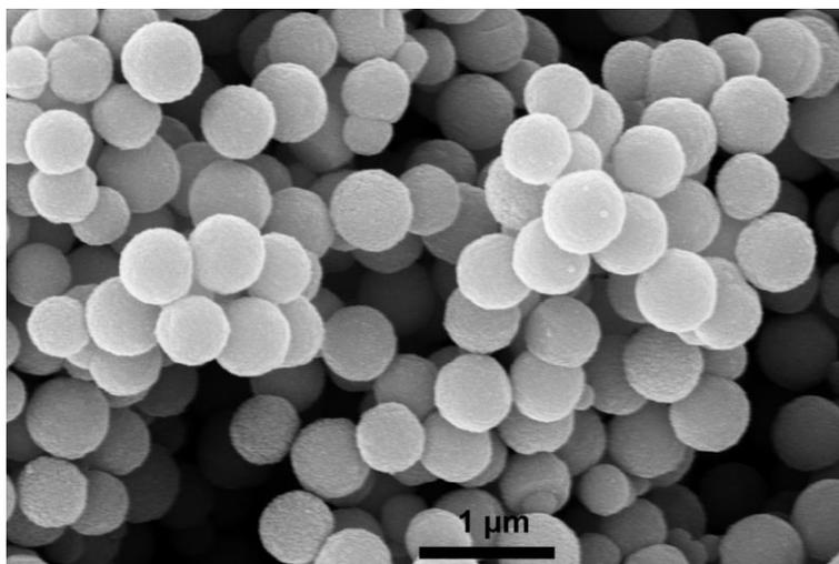
Figure S1. The SEM image of Fe<sub>3</sub>O<sub>4</sub> microspheres.
