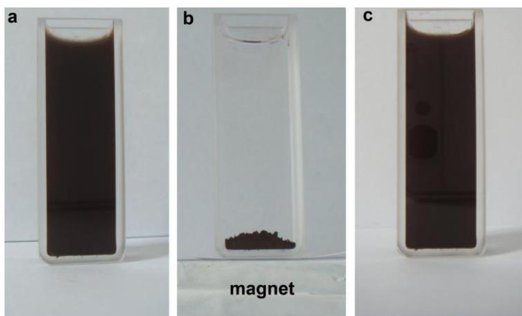
Figure S2. The digital photographs of Pd(0.1)/MFe<sub>3</sub>O<sub>4</sub> responding to external magnetic field: (a) without external magnetic field, (b) with external magnetic field, and (c) after the removal of external magnetic field.
