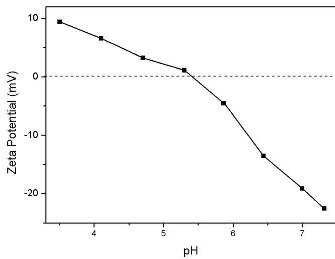
Figure S3. Zeta-potential measurement result of Pd(0.1)/Fe<sub>3</sub>O<sub>4</sub> catalyst at different pHs.
