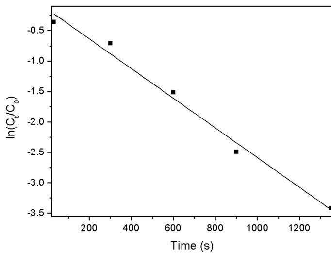
Figure S5. The catalytic bromate reduction data fitting curve by pseudo-first-order kinetic model.
