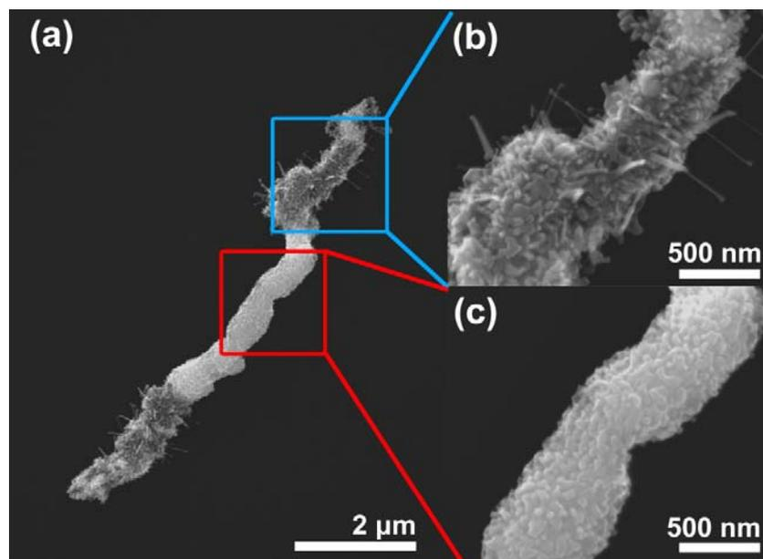
**Fig. S7** The initial state of ZnO NSSs grew on the Au-Pt-Au nanowire. (a) is the overall image of ZnO NSSs. (b) and (c) are magnified images of ZnO NSSs grew on Au and Pt segment, respectively.
