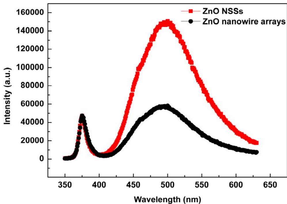
**Fig. S11** Photoluminescence (PL) spectra for ZnO NSSs and ZnO nanowire arrays.
