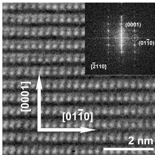
**Fig. S5** HRTEM image of individual ZnO nanowire grew from Au nanowire (55 nm in diameter). Inset shows FFT image.
