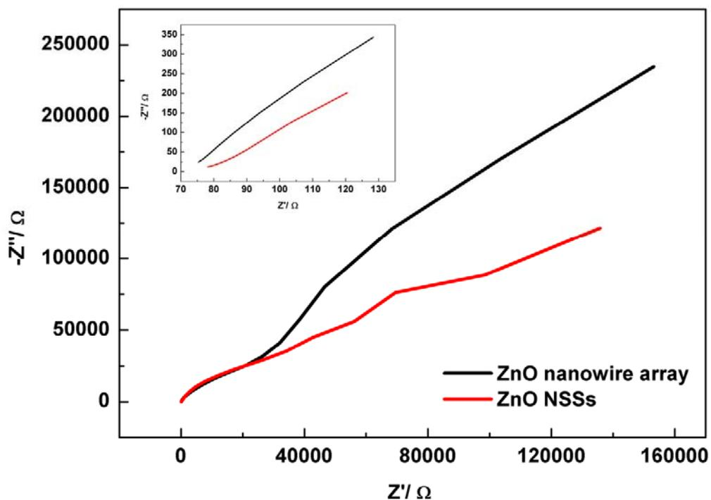
**Fig. S12** Electrochemical impedance spectroscopy (EIS) of ZnO nanowire array and ZnO NSSs electrodes.
