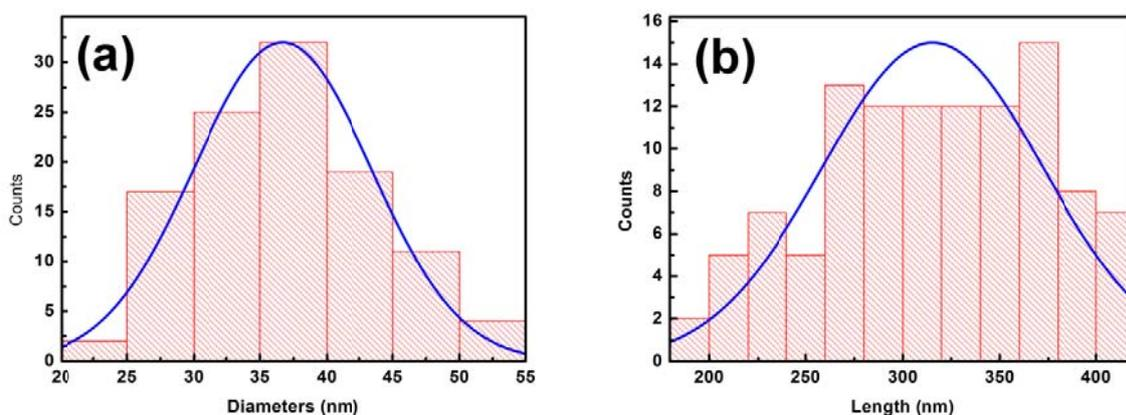
**Fig. S9** Histograms of diameter (a) and length (b) for ZnO nanowires grown on porous Au film.
