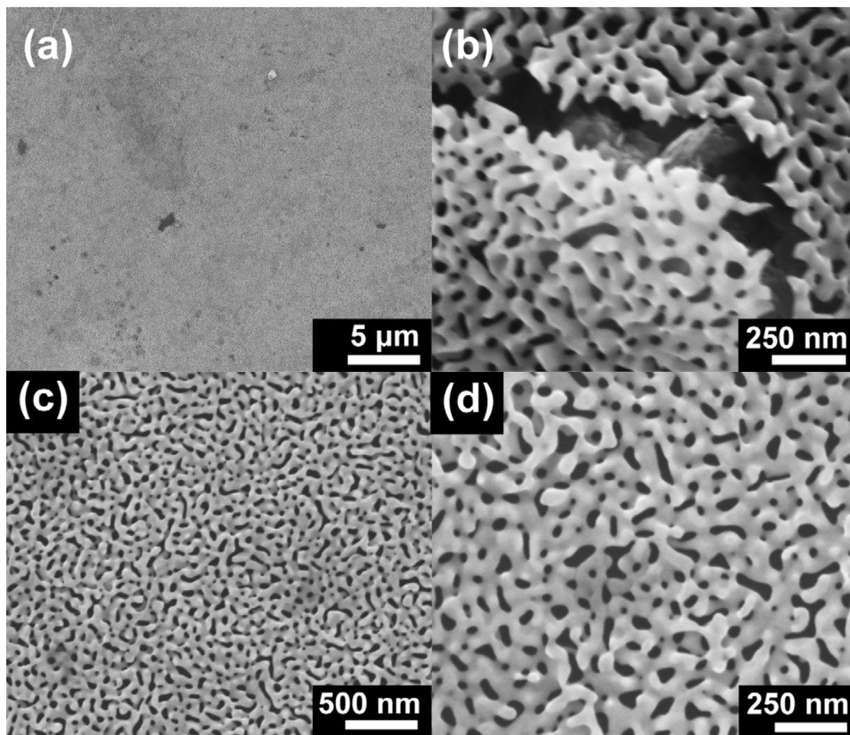
**Fig. S8 (a-d) SEM images of as-growth porous Au. The diameter of each ligament is uniform and around 50 nm.**
