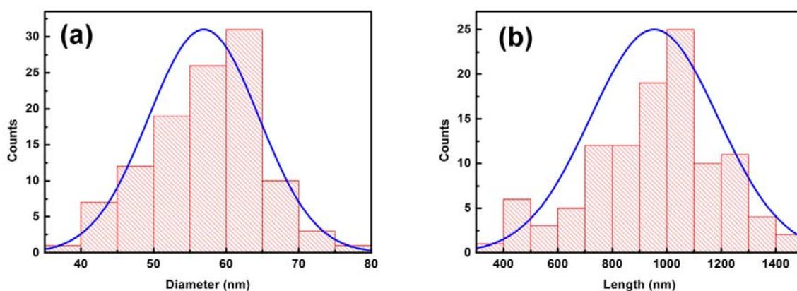
**Fig. S3** Histograms of diameter (a) and length (b) of ZnO nanowires catalyzed by 300 nm diameter Au nanowires.
