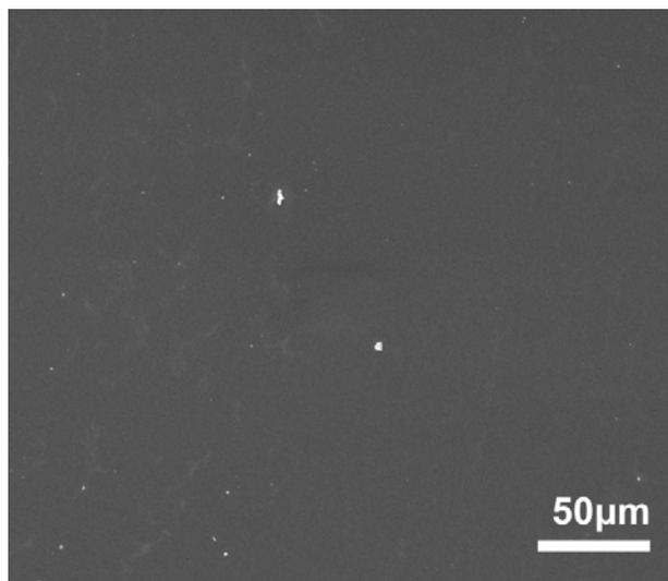
**Fig. S1 SEM image of a control sample showing ZnO essentially cannot grow on bare silicon substrate.**
