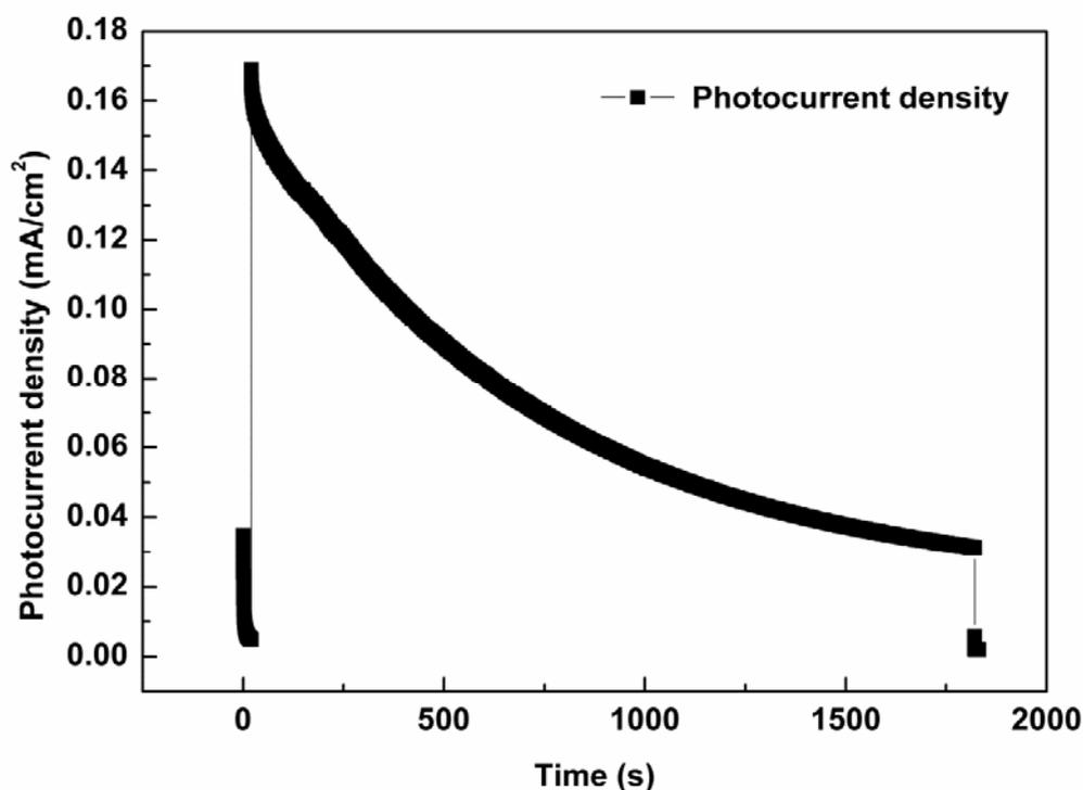
**Fig. S13 Stability test of ZnO NSSs for 30 min under 100 mW/cm<sup>2</sup> AM1.5 G at 1.21V vs. RHE.**
