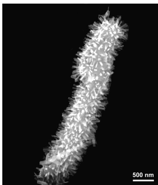
**Fig. S6** SEM image of ZnO NSSs grew on a Pt nanowire.
