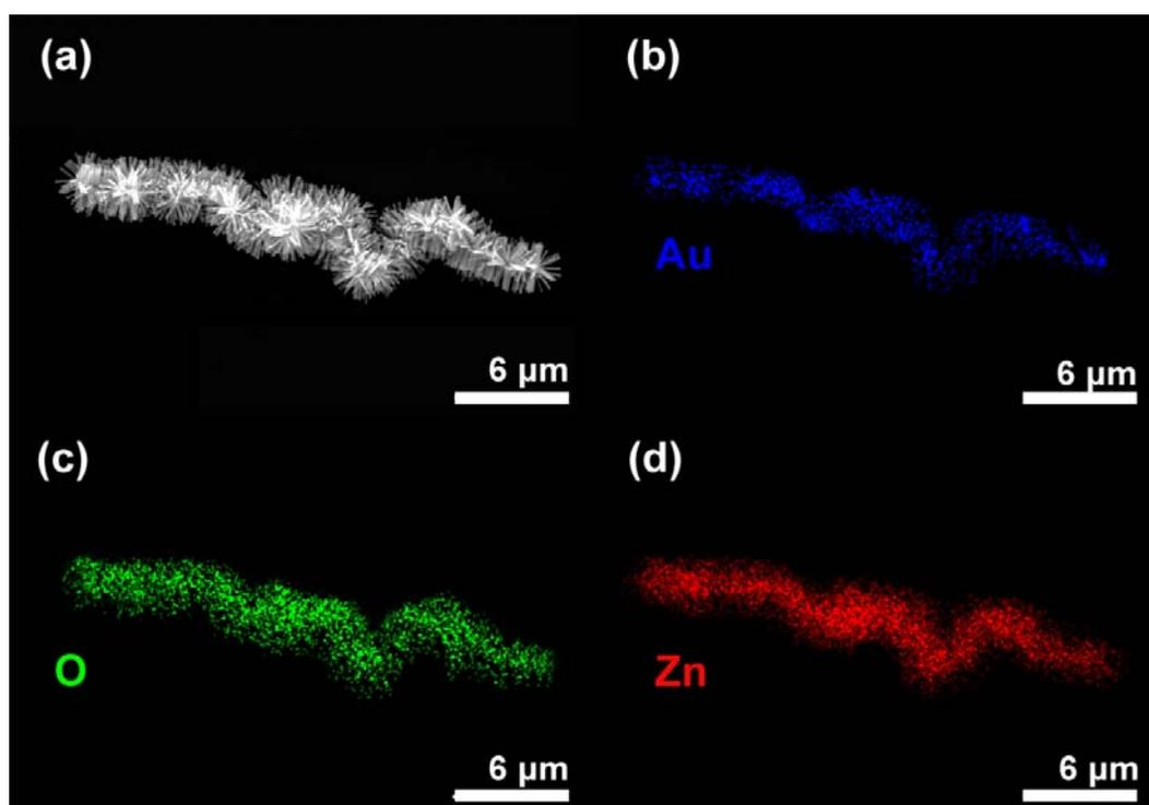
**Fig. S4** EDX mapping images of a single ZnO NSS. (a) is the SEM image of ZnO NSSs. (b), (c) and (d) show gold, oxygen and zinc element distribution, respectively.
