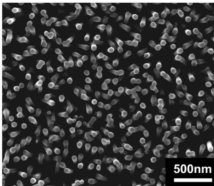
**Fig. S2 SEM image of ZnO nanowire arrays synthesized on 5 nm thick Au film.**
