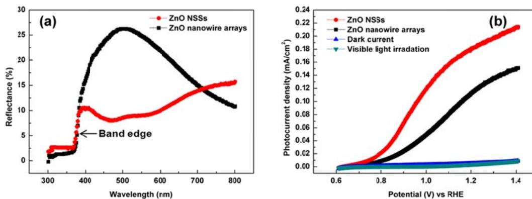
**Fig. S10** (a) UV-vis reflectance spectra for ZnO nanowire arrays and ZnO NSSs. (b) LSVs recorded under visible light irradiation.
