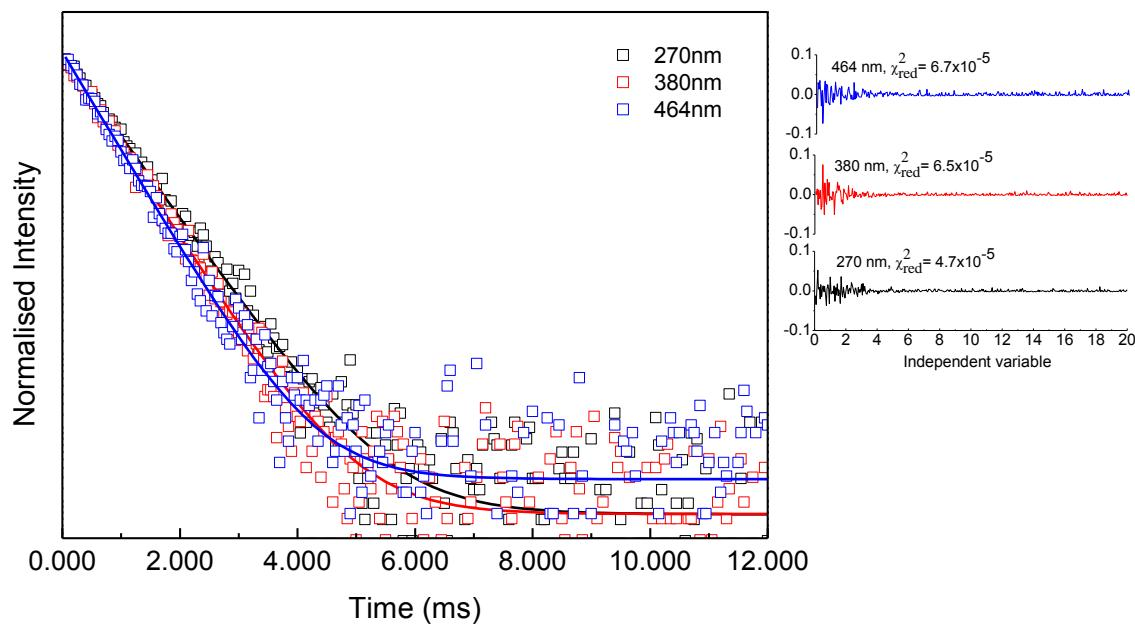
**Figure S20** – Room temperature (300K) emission decay curves excited at 270, 370 and 464 nm and monitored at 612 nm of **MtU5Eu-II**. The solid lines correspond to the data best fit using a single exponential function. On the right side the respective residual plots and the reduced- $\chi^2$  ( $\chi^2_{\text{red}}$ ) values are displayed.
