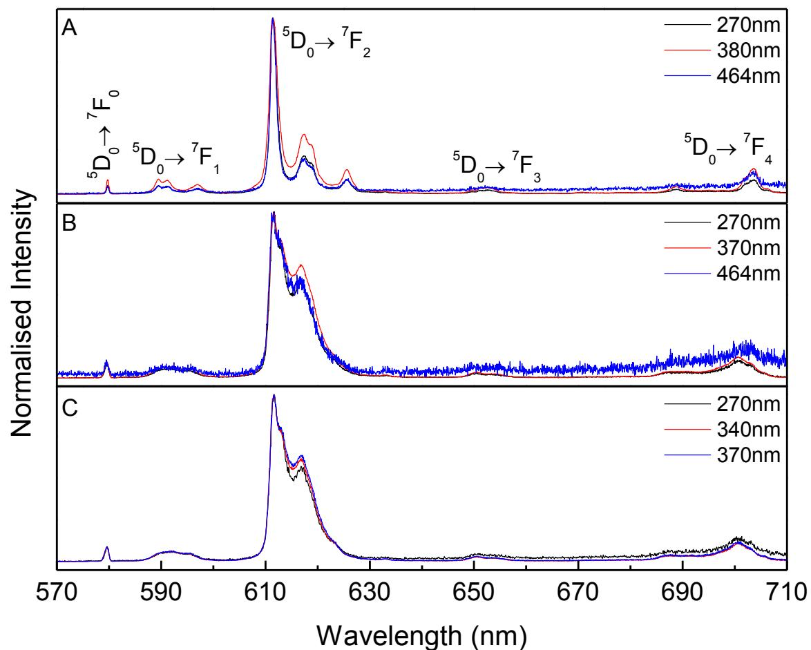
**Figure S18** - Low temperature (12K) emission spectra of (A) complex **II** and of (B) **MtU5Eu-II** excited between 270 and 464 nm.
