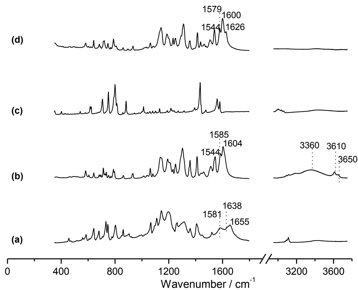
**Figure S3** – Raman spectra of the tta ligand (a), Eu(tta)<sub>3</sub>(H<sub>2</sub>O)<sub>2</sub> complex **I** (b), ephen ligand (c) and Eu(tta)<sub>3</sub>ephen complex **II** (d).
