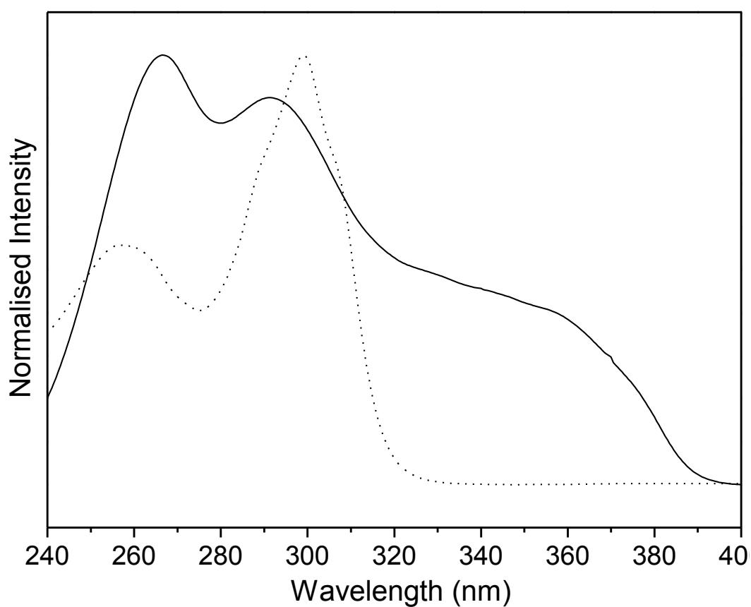
**Figure S14** – UV-Vis absorption spectra of  $\text{Eu}(\text{NO}_3)_3(\text{ephen})_2$  complex **III** (black line) and  $\text{Eu}(\text{tta})_3(\text{H}_2\text{O})_2$  complex **I** (red line) in ethanolic solution ( $10^{-5}$  and  $10^{-4}$  M, respectively)
