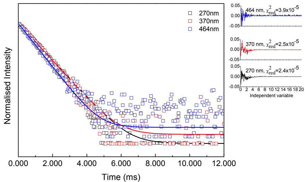
**Figure S21** - Room temperature (300K) emission decay curves excited at 270, 340 and 370 nm and monitored at 612 nm of **FtU5Eu-II**. The solid lines correspond to the data best fit using a single exponential function. On the right side the respective residual plots and the reduced- $\chi^2$  ( $\chi^2_{\text{red}}$ ) values are displayed.
