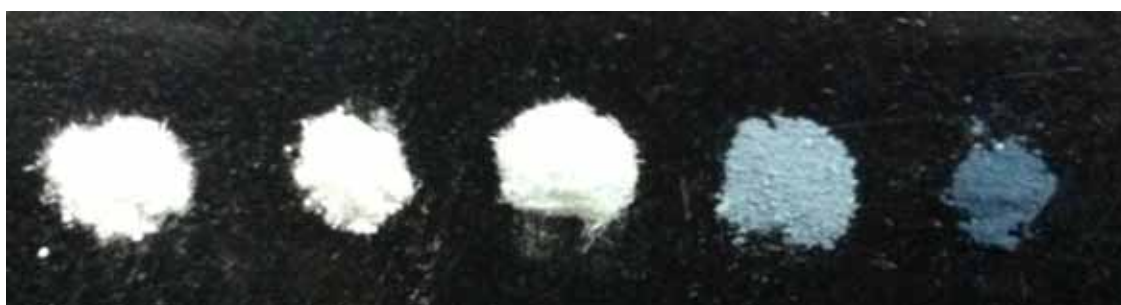
Fig. S6. The color transformation of products upon different reaction time. From left to right: 2, 7, 10, 12 and 18 h.
