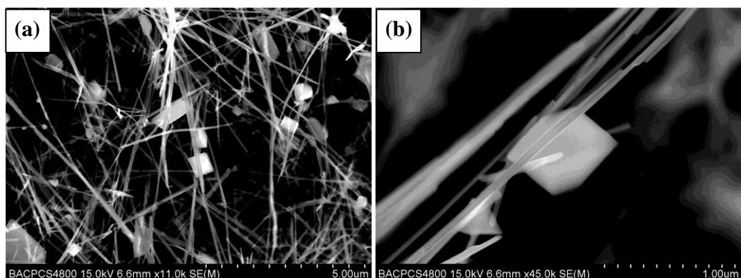
**Fig. S5** SEM images of the products obtained by hydrothermal treatment of 0.05 g KW in 10 mL 0.07 M  $\text{Co}(\text{NO}_3)_3$  aqueous solution at 150–160 °C for 24 h.
