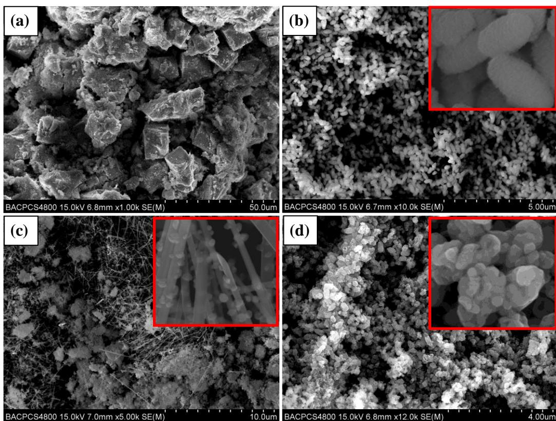
**Fig. S2** SEM images of the products obtained by hydrothermal treatment of 0.05 g KW in 10 mL 0.2 M  $\text{Fe}(\text{NO}_3)_3$  aqueous solution (170–180 °C, 36 h) with the addition of (a) 0.3 g SDBS, (b) 0.2 g SDBS, (c) 0 g SDBS, (d) 0.086g SDS.
