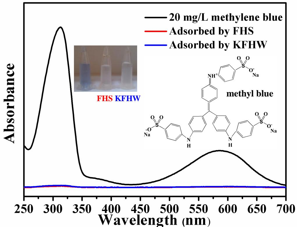
**Fig. S8** UV-vis absorption spectra and optical image of methyl blue dye before (10 mL, 20 mg/L, black curve) and after (red and blue curves) adsorption treatment for 720 min with 20 mg as-prepared FHS and KFHW nanostructures.
