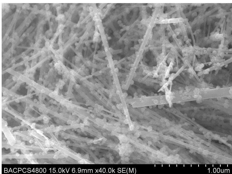
**Fig. S4** SEM image of the products obtained by hydrothermal treatment of 0.05 g KW in 10 mL 0.1 M  $\text{Fe}(\text{NO}_3)_3$  aqueous solution at 170–180 °C for 36 h.
