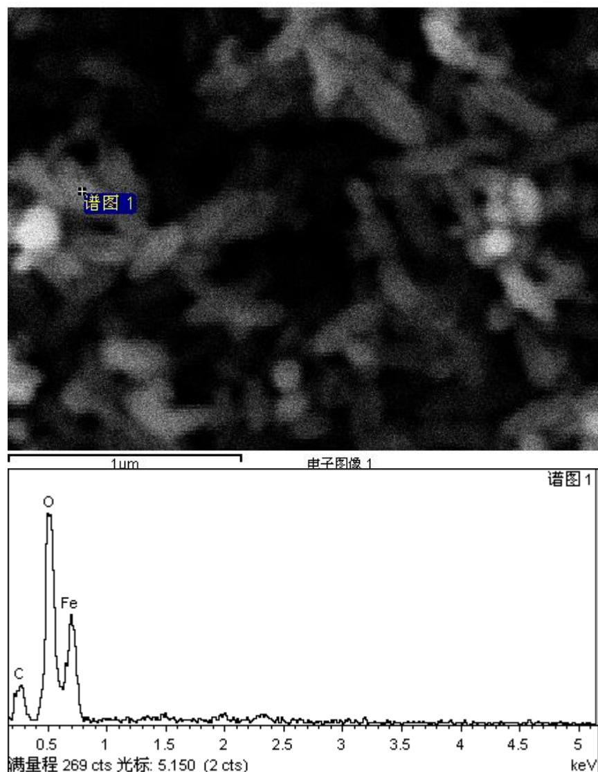
**Fig. S1** EDX spectrum of FHSs. The C signal is from carbon conductive tape.
