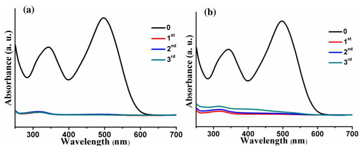
**Fig. S9** Adsorption performance of FHS (a) and KFWH (b) toward 80 mg/L Congo red solution within three cycles.
