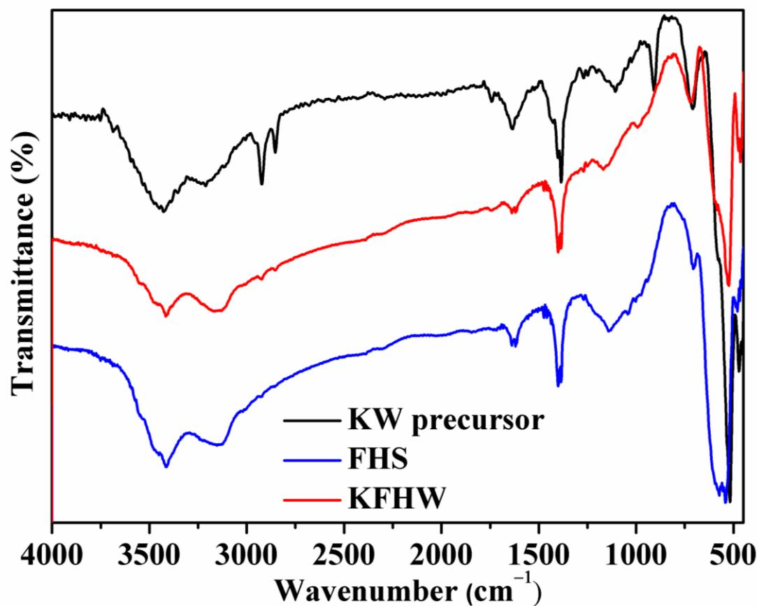
**Fig. S7** FTIR spectra of KW precursor, as-prepared FHS and KFHW nanostructures, showing the presence of hydroxyl groups on their surface. The broad, intense band at  $3412 \text{ cm}^{-1}$  is ascribed to the stretching of O–H.
