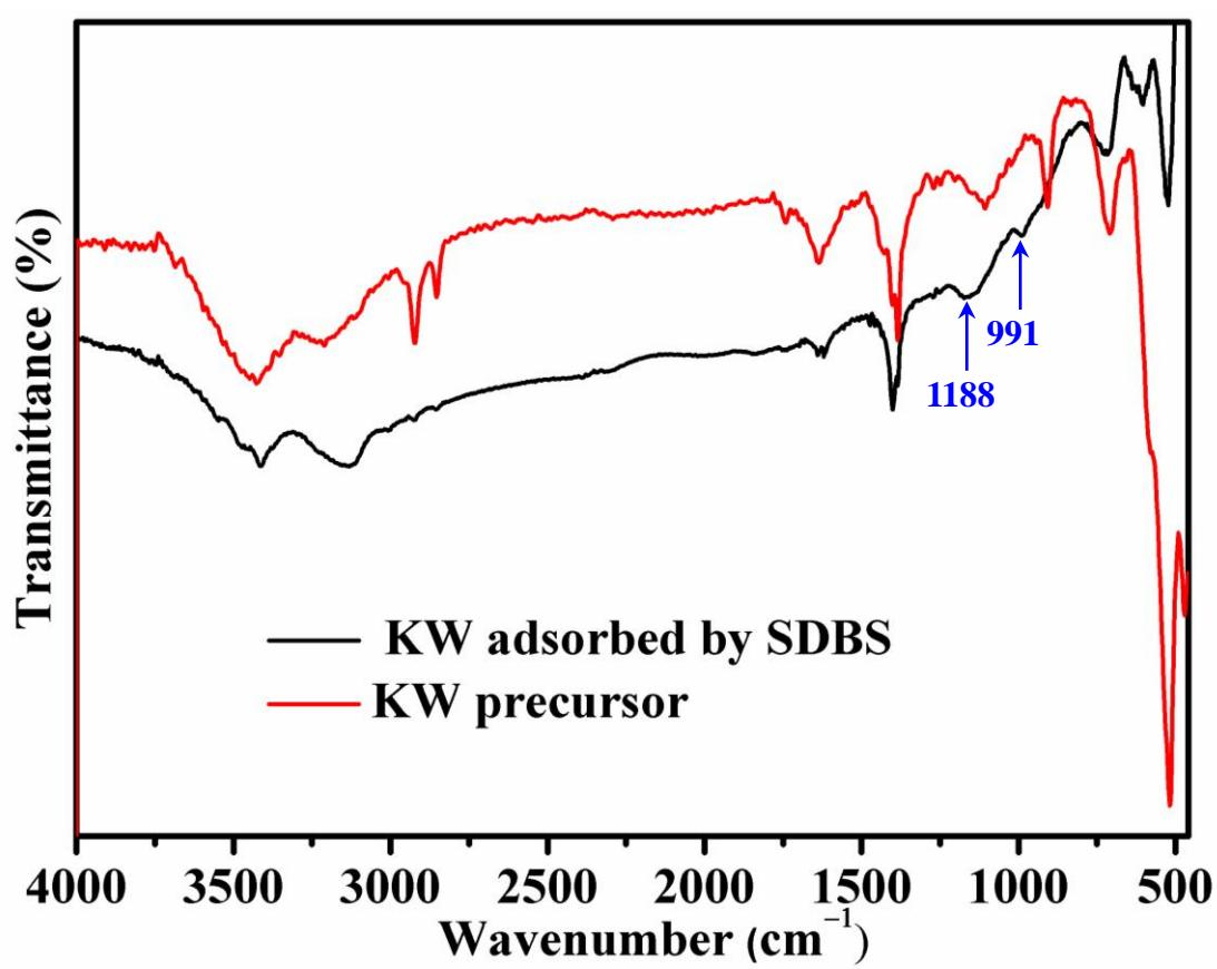
**Fig. S3** FTIR spectra of KWs before and after adsorption of SDBS.
