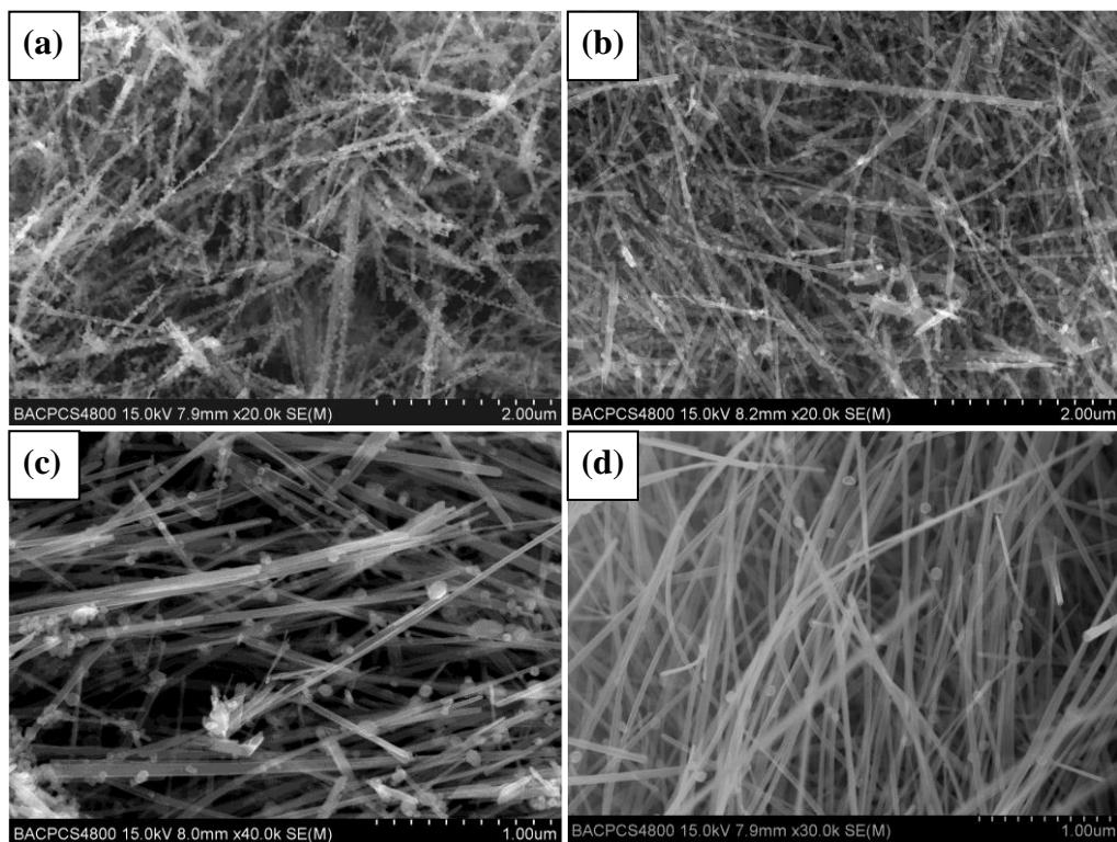
**Fig. S6** SEM images of the products obtained by hydrothermal treatment of 0.05 g KW in 10 mL  $\text{Fe}(\text{NO}_3)_3$  aqueous solution with different concentration at 150–160 °C for 24 h. (a) 0.08 M, (b) 0.06 M, (c) 0.04 M, (d) 0.02 M.
