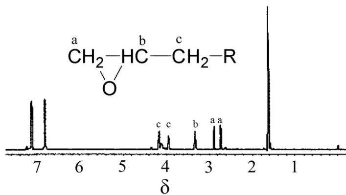
**Fig. S4.** <sup>1</sup>H-NMR Spectrum of epoxy resin E-44.
