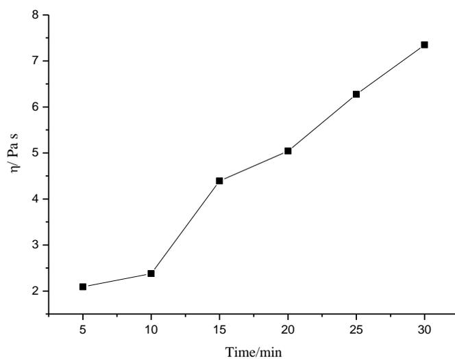
**Fig. S1.** Viscosity-time curves of resin system at 25°C. The solution viscosity increases obviously after 10 min.
