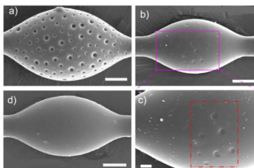
**Fig. S2.** SEM images of porous polymer BOS fabricated after different reaction temperature. (a) 25 °C, (b, c) 50 °C, (d) 75 °C. Scale bars, 10 μm.
