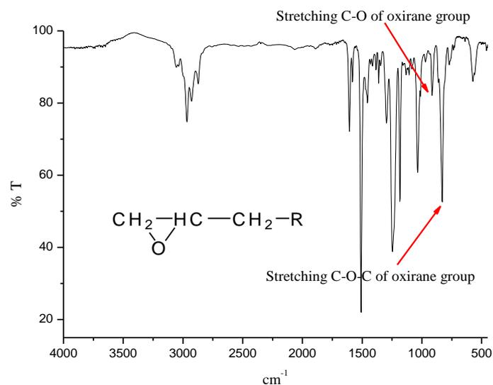
**Fig. S3.** FTIR curve of epoxy resin E-44. The bands at 913, 834 cm<sup>-1</sup> were attributed to the characteristic bands of E44.
