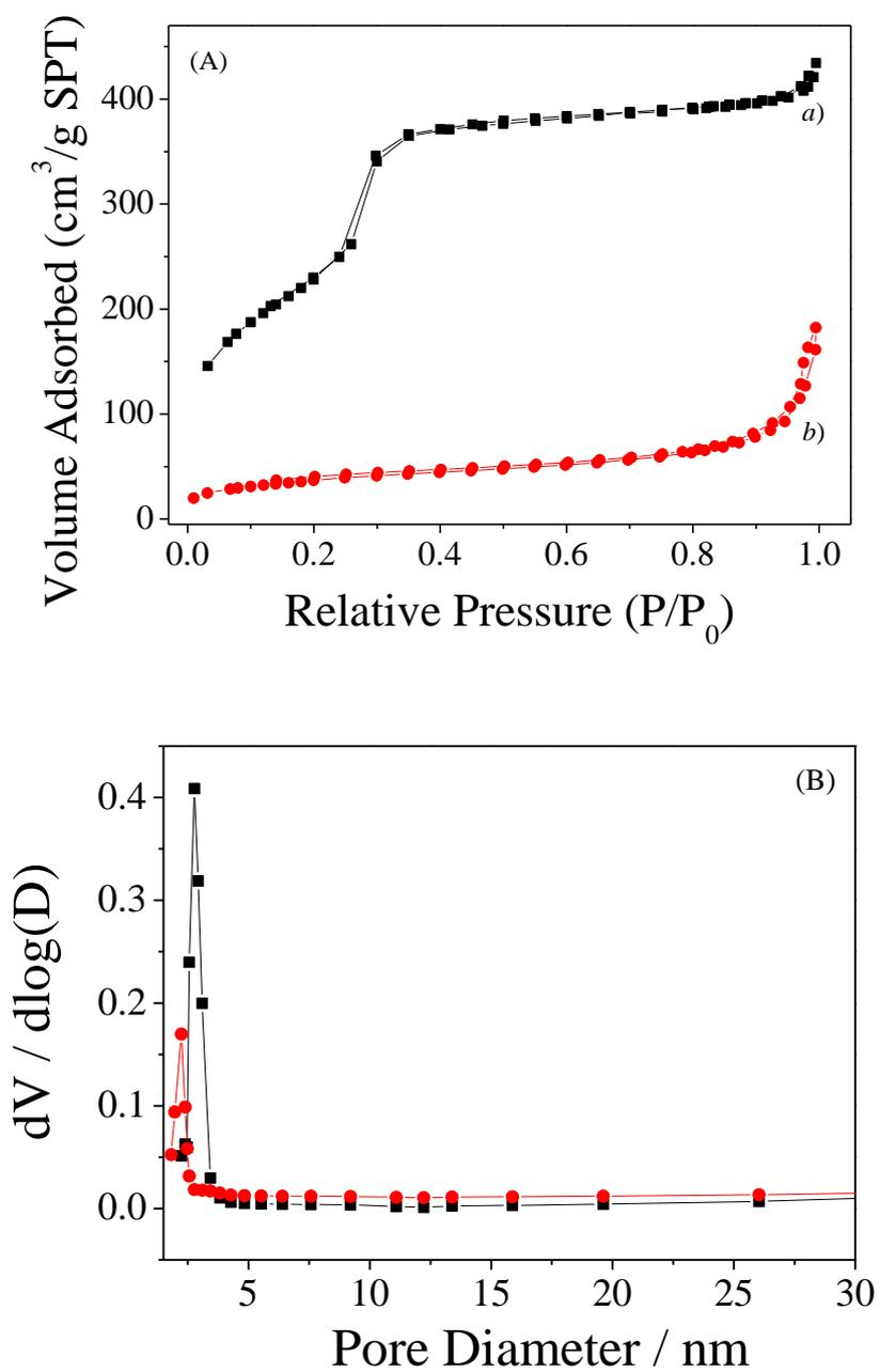
**Figure S5.** (A) BET nitrogen sorption isotherms and (B) BJH pore size distribution plots of (a)  $N_3$ -MSN( $NH_2$ ), and (b) P(OEGMA-*co*-RhBHA) coated MSN with CQA in the inner surface.
