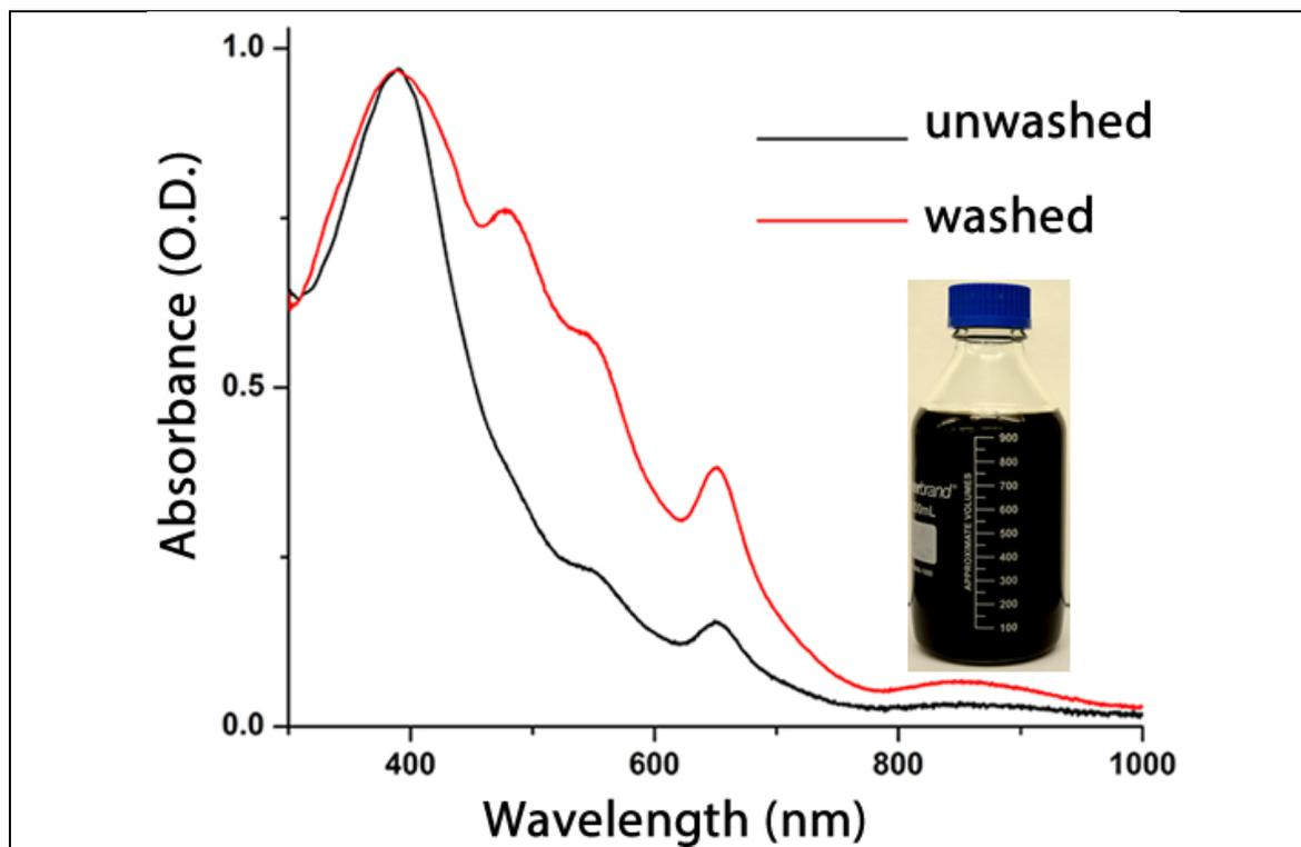
**Figure S2.** 40X scaled-up synthesis of  $\text{Ag}_{44}(\text{SR})_{30}$  NCs. The total amount of NCs in solution is 172 mg.
