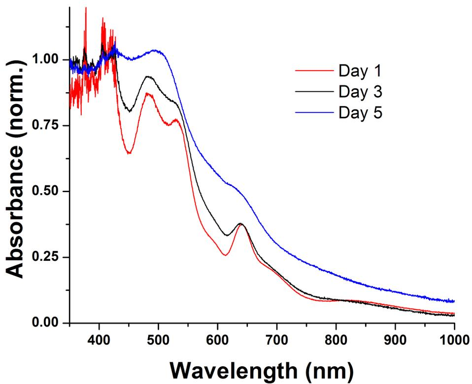
Figure S3. UV-Vis absorption spectra of 3-MBA Ag NCs with time.
