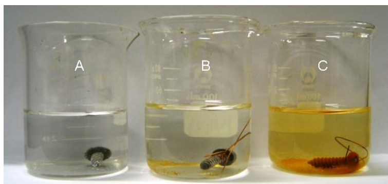
Fig. S1. Photo image of iron nails in different medium for 5 days at room temperature (about 20 °C). (A) water; (B) 0.2 M \text{NH}_4\text{Cl} ; (C) 0.2 M (\text{NH}_4)_2\text{SO}_4 .
