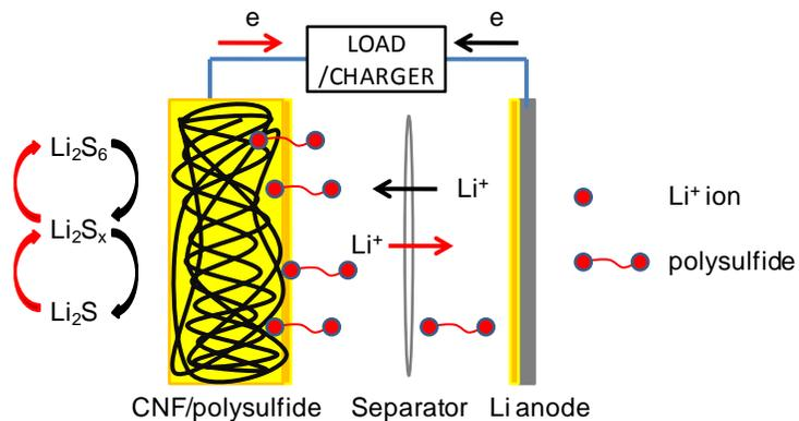
**Figure S1.** Schematic of the CNF paper/dissolved polysulfide cell.
