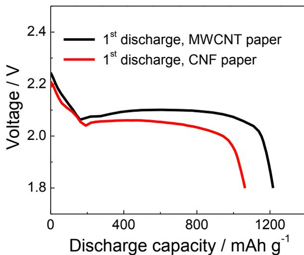
**Figure S2.** 1<sup>st</sup> discharge voltage profiles of the Li/dissolved polysulfide cells with a CNF paper electrode and a MWCNT paper electrode, cycled at C/5 rate.
