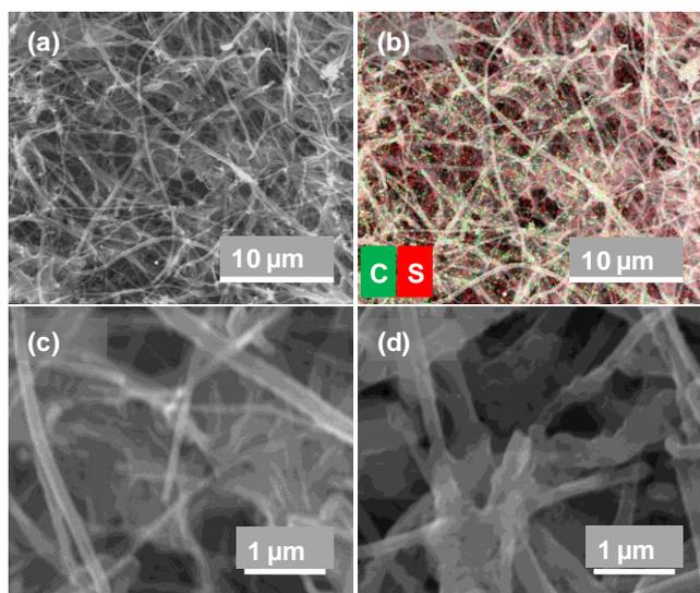
**Figure S5.** (a) SEM image of the CNF electrode after the 2<sup>nd</sup> charge in the capacity-controlled one-plateau cycling, (b) EDS sulfur and carbon mappings for the region shown in (a), with the sulfur signal in red and carbon signal in green, (c) magnified image of the region shown in (a), and (d) magnified image of the region shown in Fig. 3c.
