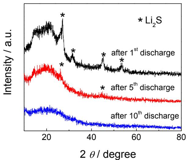
**Figure S3.** XRD patterns of the CNF paper electrode after 1<sup>st</sup>, 5<sup>th</sup>, and 10<sup>th</sup> discharge.
