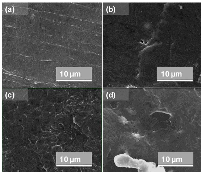
**Figure S4.** SEM images of the lithium metal anode (a) before cycling and after the (b) 1<sup>st</sup>, (c) 5<sup>th</sup>, and (d) 10<sup>th</sup> discharge.
