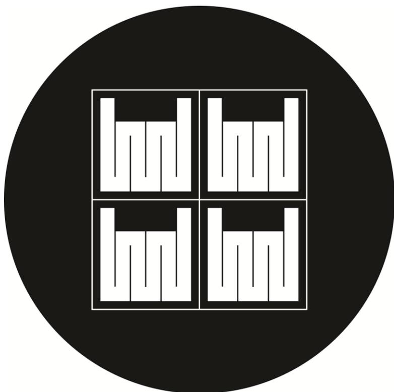
**Figure S1.** The negative used for etching the microfluidic glass chips. Four glass chips were made using one glass wafer.
