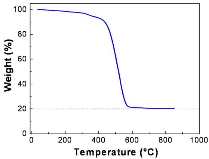
**Figure S2:** TGA image of Pd/N-SG sample
