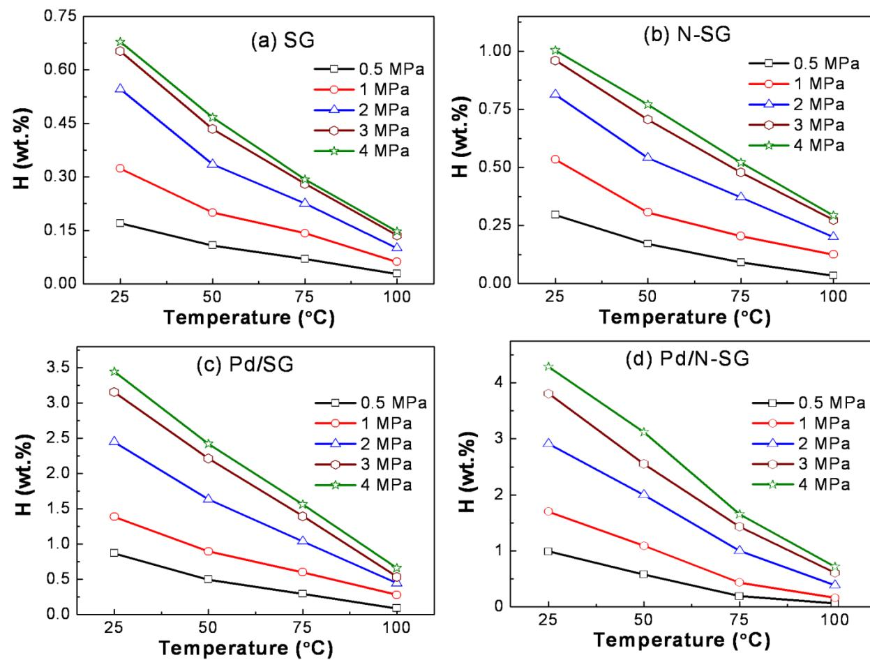
**Figure S3:** Temperature variations of hydrogen storage capacity for the samples SG, N-SG, Pd/SG and Pd/N-SG at different pressures.
