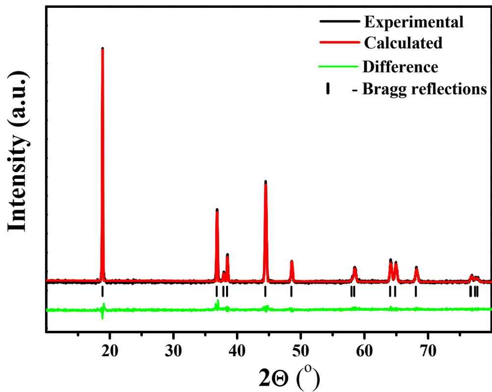
Fig. S2. Rietveld refinement of the structure of  $\text{Li}_3\text{CoRuO}_5$  from PXRD data.
