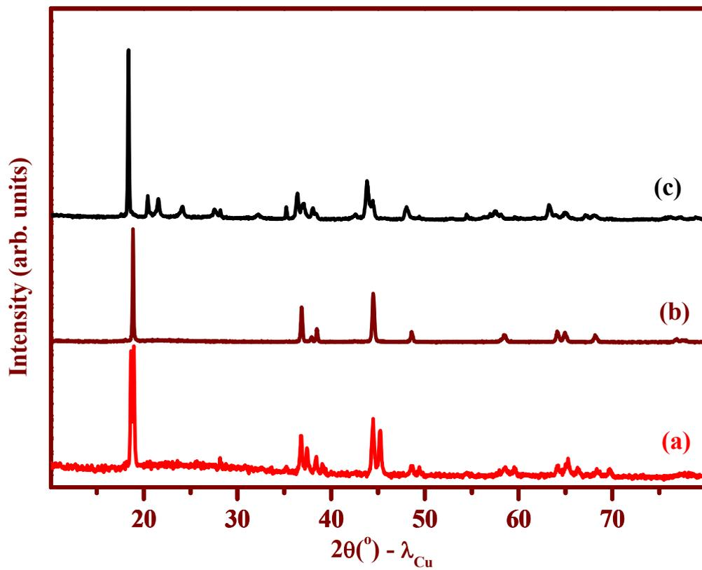
Fig. S1. PXRD patterns of  $\text{Li}(\text{Li}_x\text{Co}_{1-3x}\text{Ru}_{2x})\text{O}_2$ : (a)  $x = 0.1$ ; (b)  $x = 0.2$ ; (c)  $x = 0.3$ .
