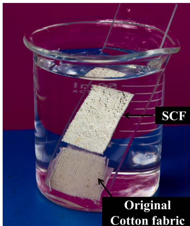
Fig. S4 Photograph of a sample of uncoated cotton fabric (below) and of an SCF sample (above) after immersion into water. A plastron layer is visible on the surface of the SCF.
