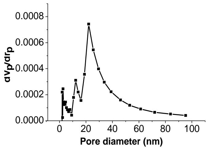
**Figure S8.** Pore size distribution of CdO architectures obtained by BET analysis.
