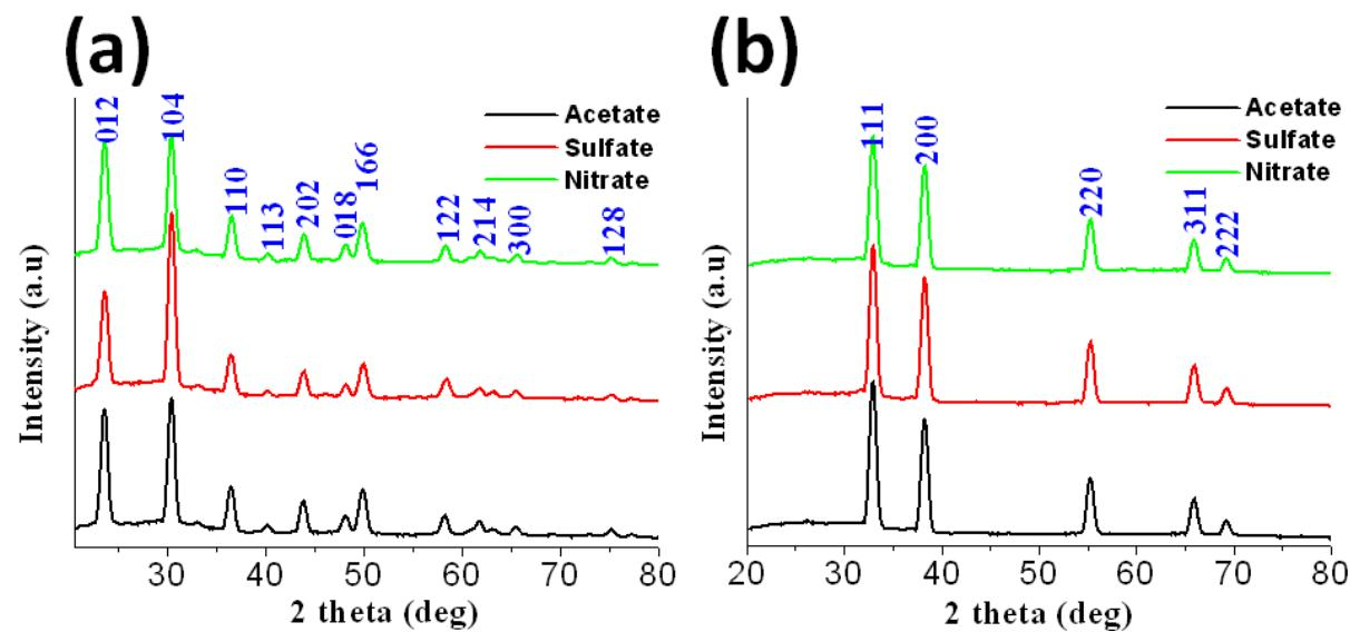
**Figure S3.** XRD patterns of (a)  $\text{CdCO}_3$  and (b)  $\text{CdO}$  crystals obtained using different  $\text{Cd}^{2+}$  ion precursors
