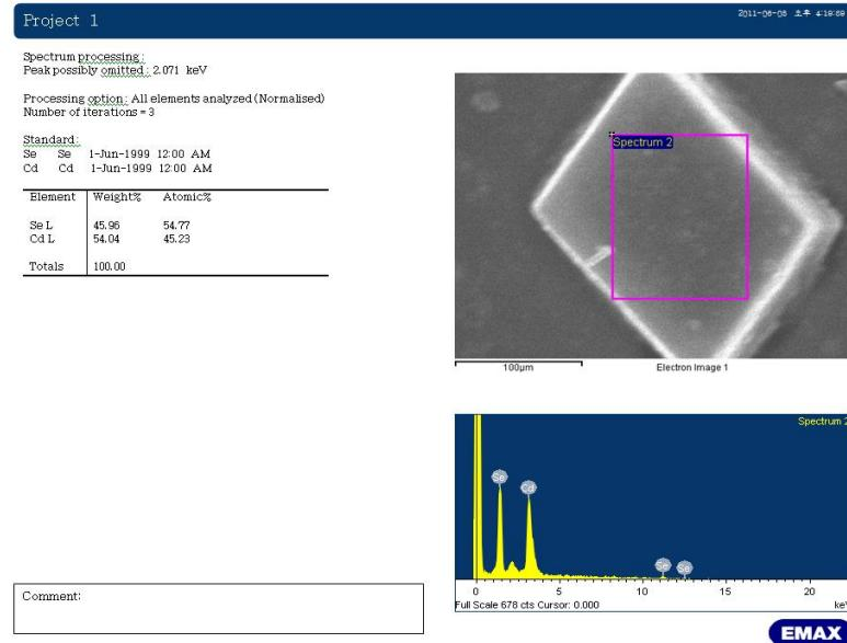
**Figure S5.** EDX analysis of CdO-CdSe crystal obtained after 30 min. of ion exchange reaction
