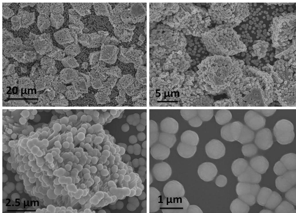
**Figure S6.** SEM images of the  $\text{CdCO}_3$  crystals with different magnifications, after ion exchange with  $\text{Se}^{2-}$  ion solution
