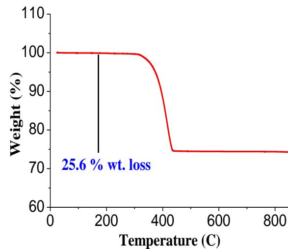
**Figure S1.** Thermo-gravimetric analysis (TGA) of CdCO<sub>3</sub> crystals obtained under nitrogen flow at heating rate of 10 °C min<sup>-1</sup>
