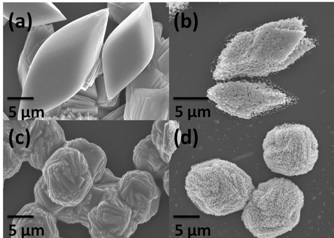
**Figure S2.** SEM images of the  $\text{CdCO}_3$  and  $\text{CdO}$  crystals obtained using  $\text{CdSO}_4$  (a) and  $\text{Cd}(\text{CH}_3\text{COO})_2$  (c) as  $\text{Cd}^{2+}$  ion precursors.
