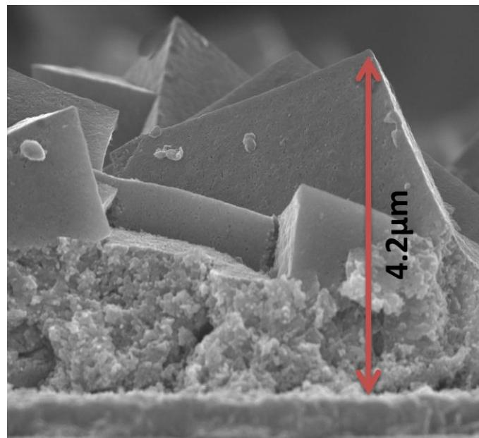
**Figure S7.** Cross section SEM image of the CdO architectures on ITO surface.
