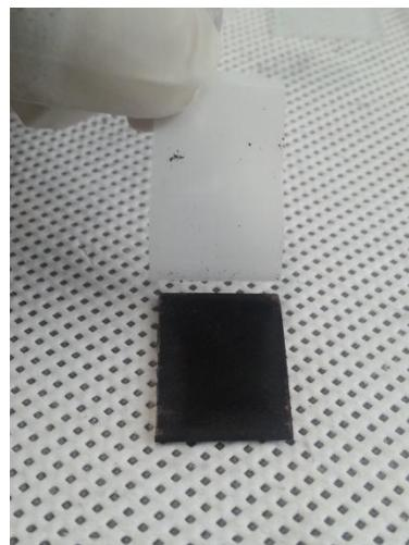
**Figure S9.** Scotch tape after complete removal from ITO/CdO-CdSe architecture surface
