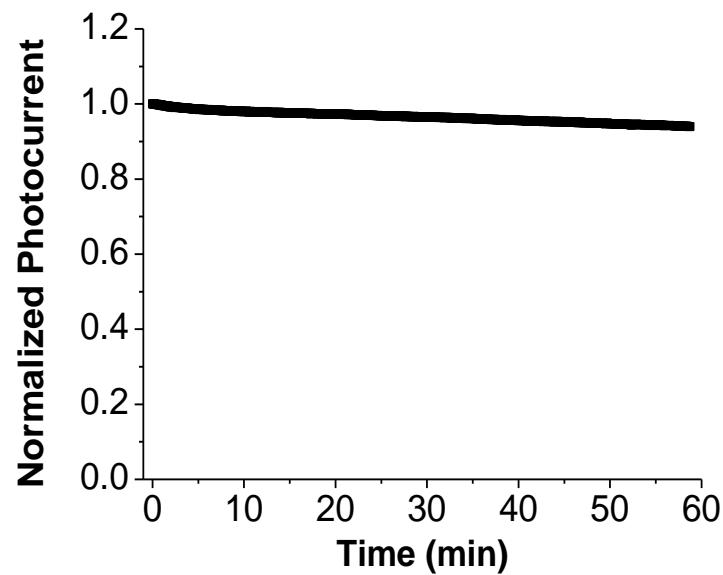
**Figure S10.** A plot of normalized Short-circuit current density versus time of the CdO-CdSe photoelectrochemical cell obtained under continuous illumination of 1Sun for 1 hour. Almost 93 % of photocurrent was retained after 1 hour of continuous illumination. With a proper sealant, it should be possible to avoid electrolyte evaporation during long-term irradiation which would give more stability to the device.
