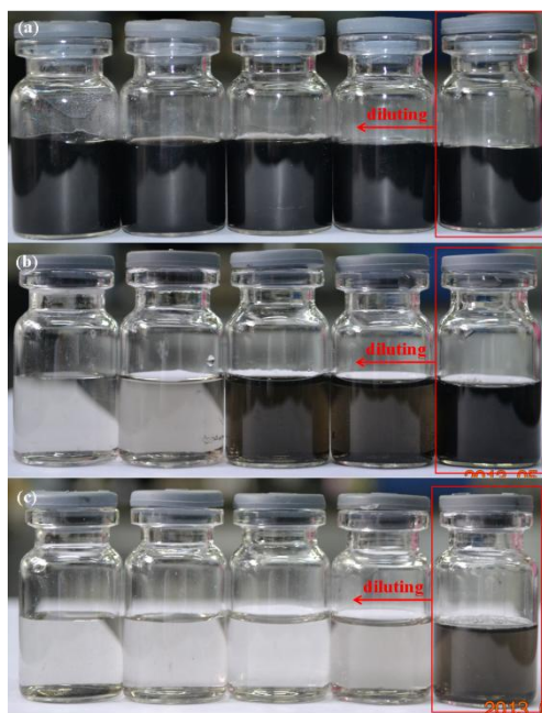
Fig. S4. Photographic images of original (a) LRD (1.83 mg/mL SWNTs in 20 mg/mL LRD), (b) SDBS (0.04 mg/mL in 4 mg/mL SDBS) and SDS (0.02 mg/mL in 4 mg/mL SDS) dispersed SWNTs (marked with red rectangles). The dispersions were further diluted to 0.5, 0.4, 0.2 and 0.1 of their original concentrations (right to left).
