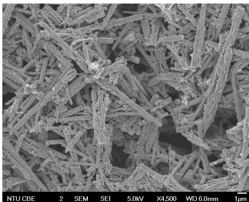
Fig. S11 A typical SEM image of porous \text{Co}_3\text{O}_4 nanorods.
