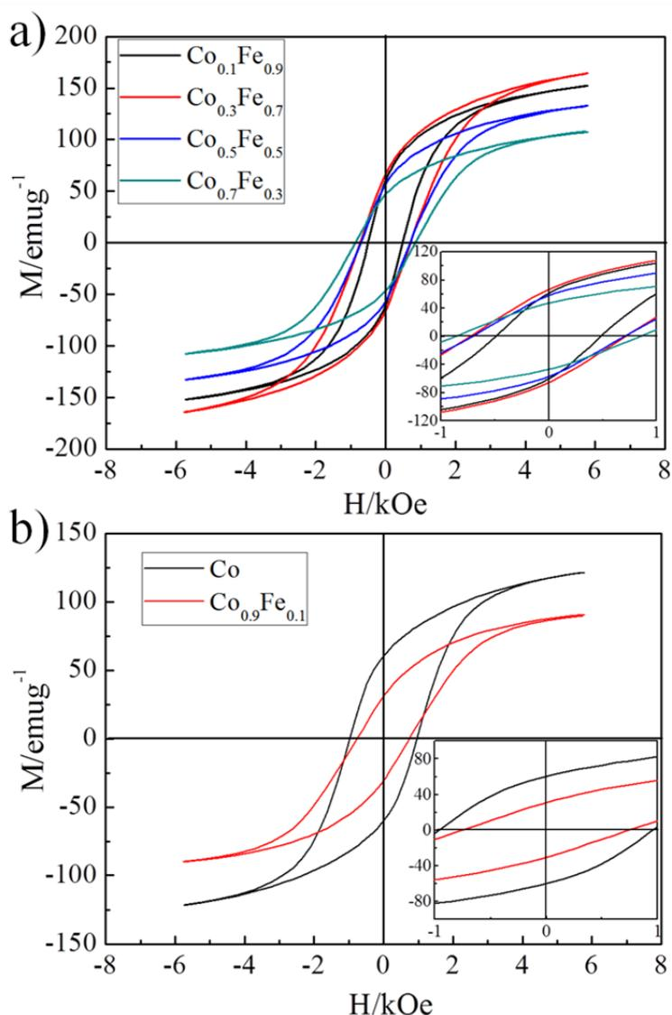
**Figure. S4** Magnetic hysteresis loops (M-H loops) of a) leaf-like dendritic Co<sub>x</sub>Fe<sub>1-x</sub> (x = 0.1, 0.3, 0.5 and 0.7) and b) grain-like dendritic Co<sub>0.9</sub>Fe<sub>0.1</sub> and ε-Co at room temperature. The inset is the expanded low-field hysteresis curves.
