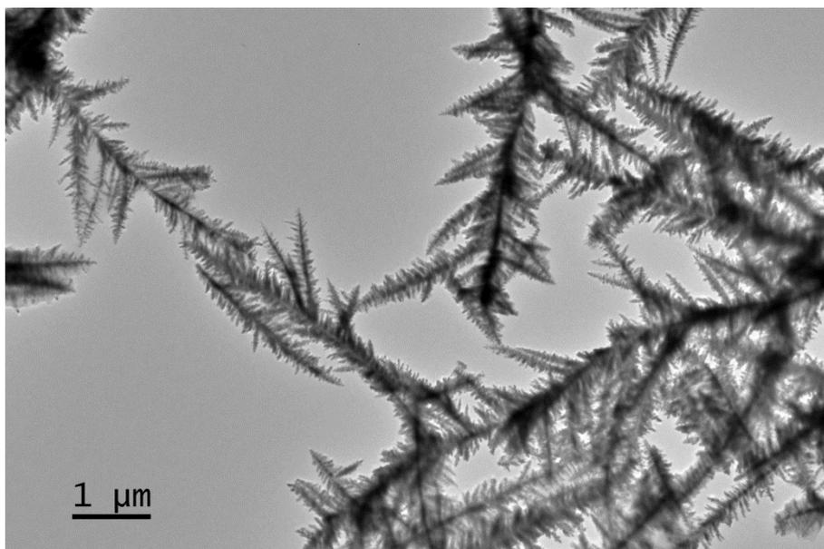
**Figure S1.** TEM image of the grain-like dendritic micro-nano structure  $\epsilon$ -Co.
