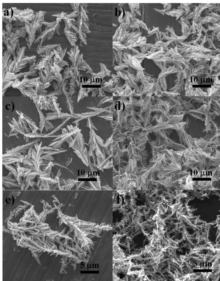
**Figure S2.** Low-magnification SEM images of leaf-like dendritic a)  $\text{Co}_{0.1}\text{Fe}_{0.9}$ , b)  $\text{Co}_{0.3}\text{Fe}_{0.7}$ , c)  $\text{Co}_{0.5}\text{Fe}_{0.5}$  and d)  $\text{Co}_{0.7}\text{Fe}_{0.3}$  alloys, and grain-like dendritic e)  $\text{Co}_{0.9}\text{Fe}_{0.1}$  alloy and f)  $\epsilon\text{-Co}$ .
