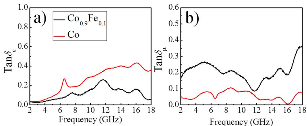
**Figure S5.** a) The dielectric loss tangents ( $\tan\delta_\epsilon=\epsilon''/\epsilon'$ ) and b) magnetic loss tangents ( $\tan\delta_\mu=\mu''/\mu'$ ) of grain-like dendritic micro-nano structure  $\text{Co}_{0.9}\text{Fe}_{0.1}$  alloys and  $\epsilon\text{-Co}$  under different frequencies.
