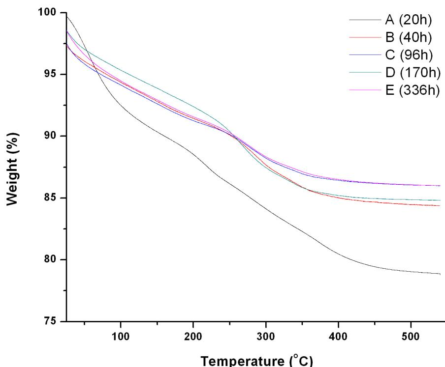
**Figure S1.** TGA curves for samples A, B, C, D and E reacted for 20h, 40h, 96h, 170h and 336h, respectively. The mass loss region between 25 °C and 150 °C is attributed to surface adsorbed water. The onset of mass loss observed at approximately 200 °C is attributed to loss of organic material adsorbed to the titanium dioxide nanoparticles surfaces.
