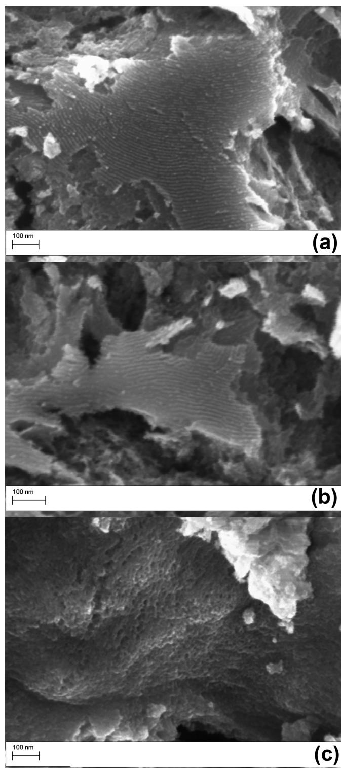
Figure S3. SEM micrographs of films F (a), G (b), H (c) display pores within the mesorange.
