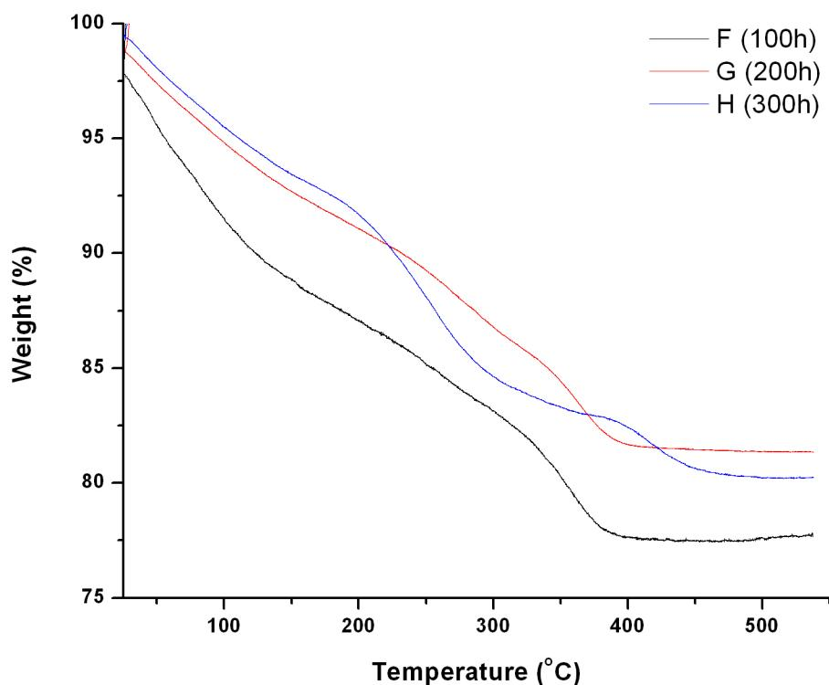
**Figure S2.** TGA curves for sample films F, G and H aged for 100h, 200h and 300h, respectively. The mass loss region between 25 °C and 150 °C is attributed to surface adsorbed water. The onset of mass loss observed at approximately 200 °C is attributed to loss of organic material adsorbed to the titanium dioxide nanoparticle surfaces.
