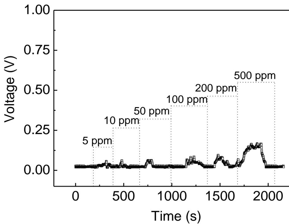
**Fig. S1** Dynamic response-recovery curves of the sensor to HCHO with different concentrations at 260 °C.
