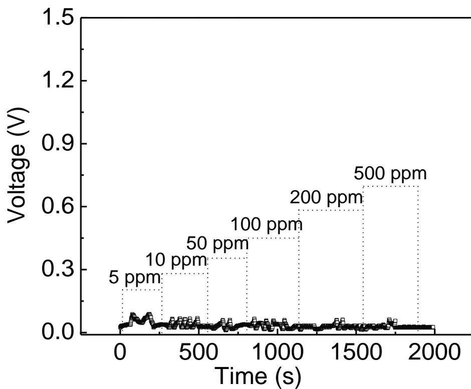
**Fig. S2** Dynamic response-recovery curves of the sensor to NH<sub>3</sub> with different concentrations at 260 °C.
