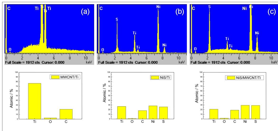
**Fig. S2** EDS spectra of the MWCNT/Ti (a), NiS/Ti (b), and NiS/MWCNT/Ti (c) CEs, respectively.
