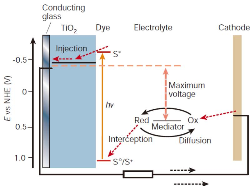
**Fig. 5** Schematic of energy levels and operation of the DSSC. (cited from M. Gratzel, *Nature* 2001, 414, 338-344).
