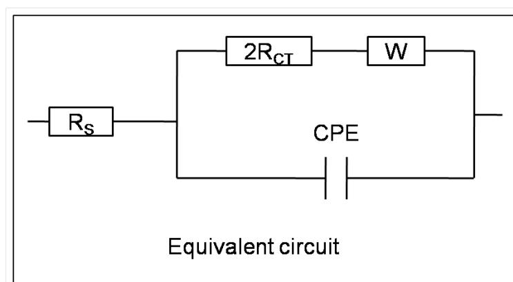
**Fig. S3** Equivalent circuit used for fitting the EIS results of the symmetric cells.
