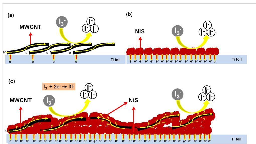
**Fig. S4** Schematic of the catalytic mechanisms of MWCNT (a), NiS (b), and NiS/MWCNT (c) CEs, respectively.
