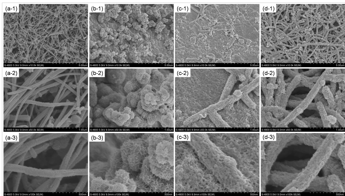
**Fig. S1** SEM images of MWCNT/Ti (a-1, a-2, and a-3), NiS/Ti (b-1, b-2, and b-3), NiS/MWCNT/Ti with sparse MWCNT (c-1, c-2, and c-3), and NiS/MWCNT/Ti with enough MWCNT (d-1, d-2, and d-3) CEs, respectively.
