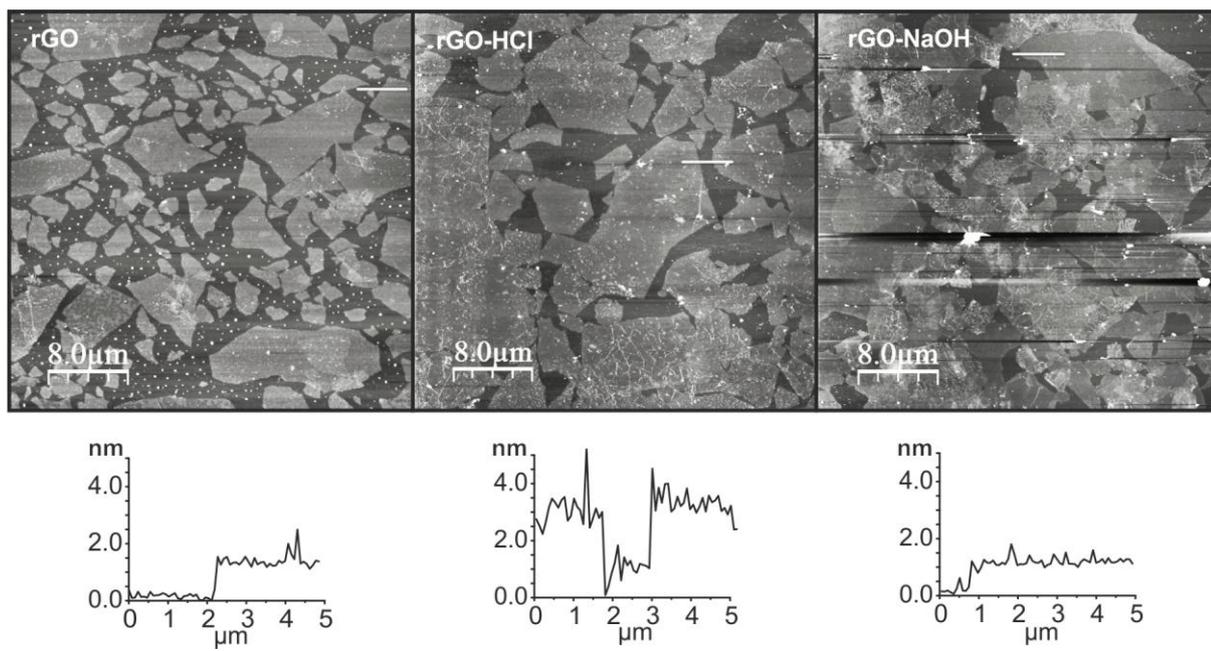
Figure S4. AFM images of reduced GO (rGO), rGO-HCl and rGO-NaOH on Si/SiO<sub>2</sub> substrates with height-profiles below.
