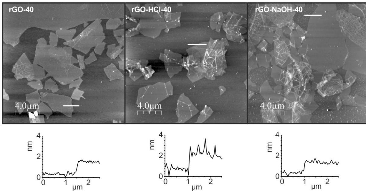
Figure S5. AFM images of rGO-40, rGO-HCl-40 and rGO-NaOH-40 on Si/SiO<sub>2</sub> substrates with height-profiles below.
