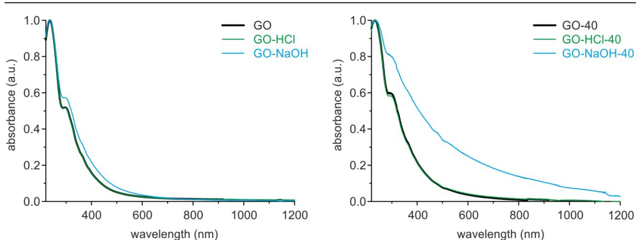
Figure S1. left: UV-Vis spectra of GO, GO-NaOH and GO-HCl (treated with 0.1M HCl; normalized on absorption at 235 nm) and right: UV-Vis spectra of GO-40, GO-NaOH-40 and GO-HCl-40:
