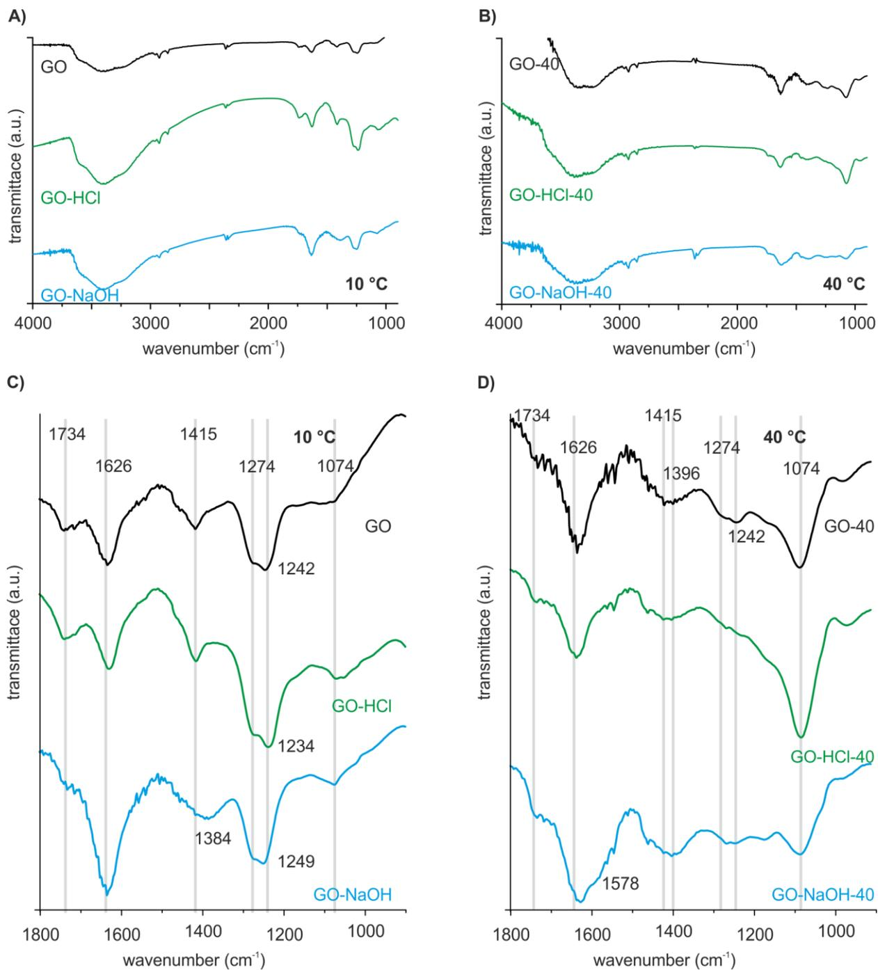
Figure S2. FTIR spectra of GO, GO-HCl and GO-NaOH and GO-40, GO-HCl-40 and GO-NaOH-40; A) and B) overview of GO samples treated at 10 °C or 40 °C and C) and D) enlargement of the fingerprint region (1800-900 cm<sup>-1</sup>) of GO samples treated at 10 °C or 40 °C.
