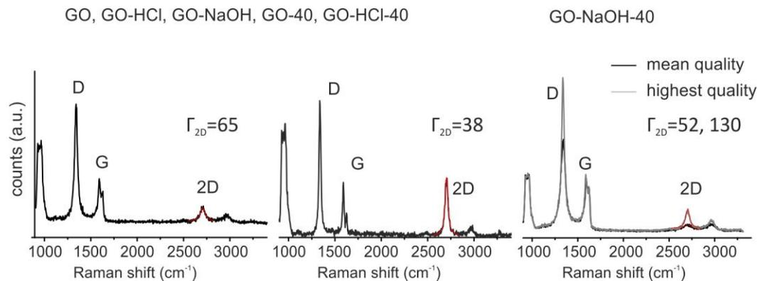
Figure S6. Typical Raman spectra of rGO; left: mean quality of spectra (rGO, rGO-HCl, rGO-NaOH, rGO-40, rGO-HCl-40 and middle: Raman spectrum of high-quality flakes; right: Raman spectra of rGO-NaOH-40; mean quality with  $\Gamma_{2D}=130\text{ cm}^{-1}$  and highest quality with  $\Gamma_{2D}=52\text{ cm}^{-1}$ .
