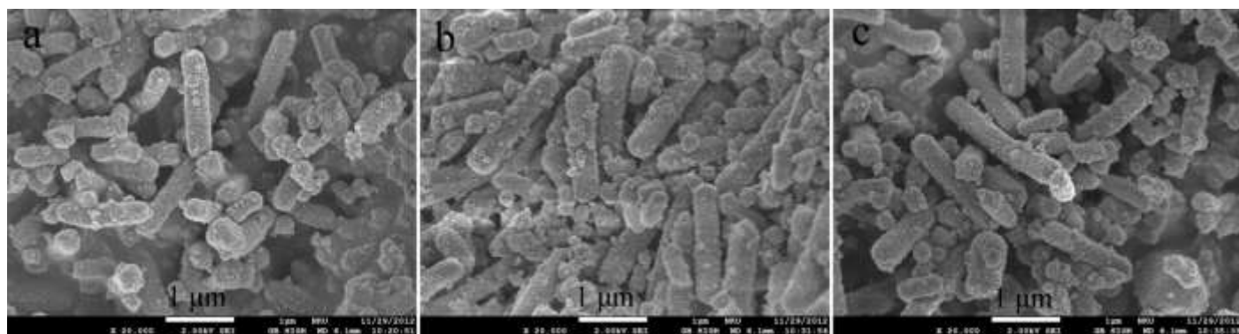
Figure S3. SEM images of the calcined samples prepared at 80 °C for (a) 0 h, (b) 6 h and (c) 24 h reaction time, respectively. 0 h means the sample was obtained after stirring 15 min of the reactant mixture at room temperature but without heating treatment in the 80 °C oven.
